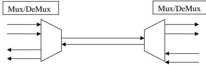
Figure 1: Multiplexer and de-multiplexer
