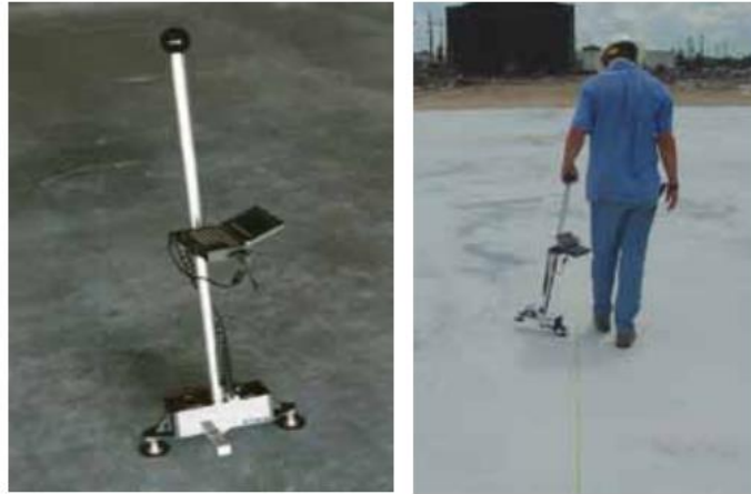
Figure 2.2. Dipstick Floor Profiler Used to Collect Data [20]
