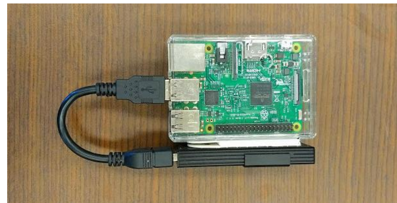
Fig. 2. Prototype radiation dosimeter consisting of a Timepix detector and Raspberry Pi 3 minicomputer.
