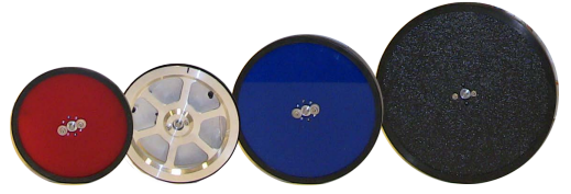
Fig. 7. Four wheel sizes used for experimental validation. These wheels are 10.16, 10.48, 12.7 and 15.24 cm in diameter.
