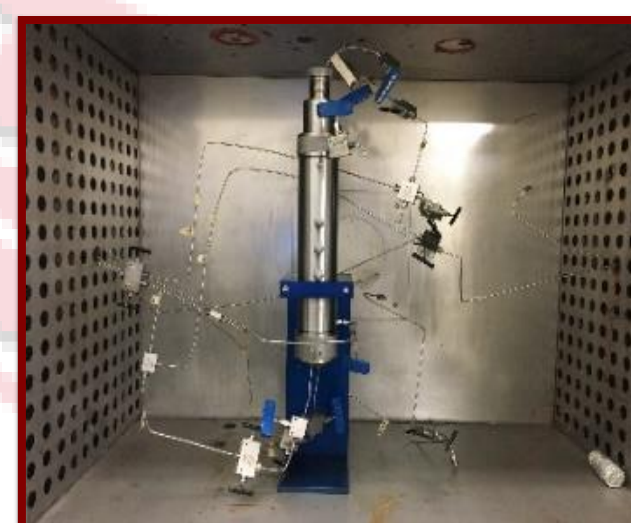
Figure 10: Injection and Vacuum Core Flood Mechanism
