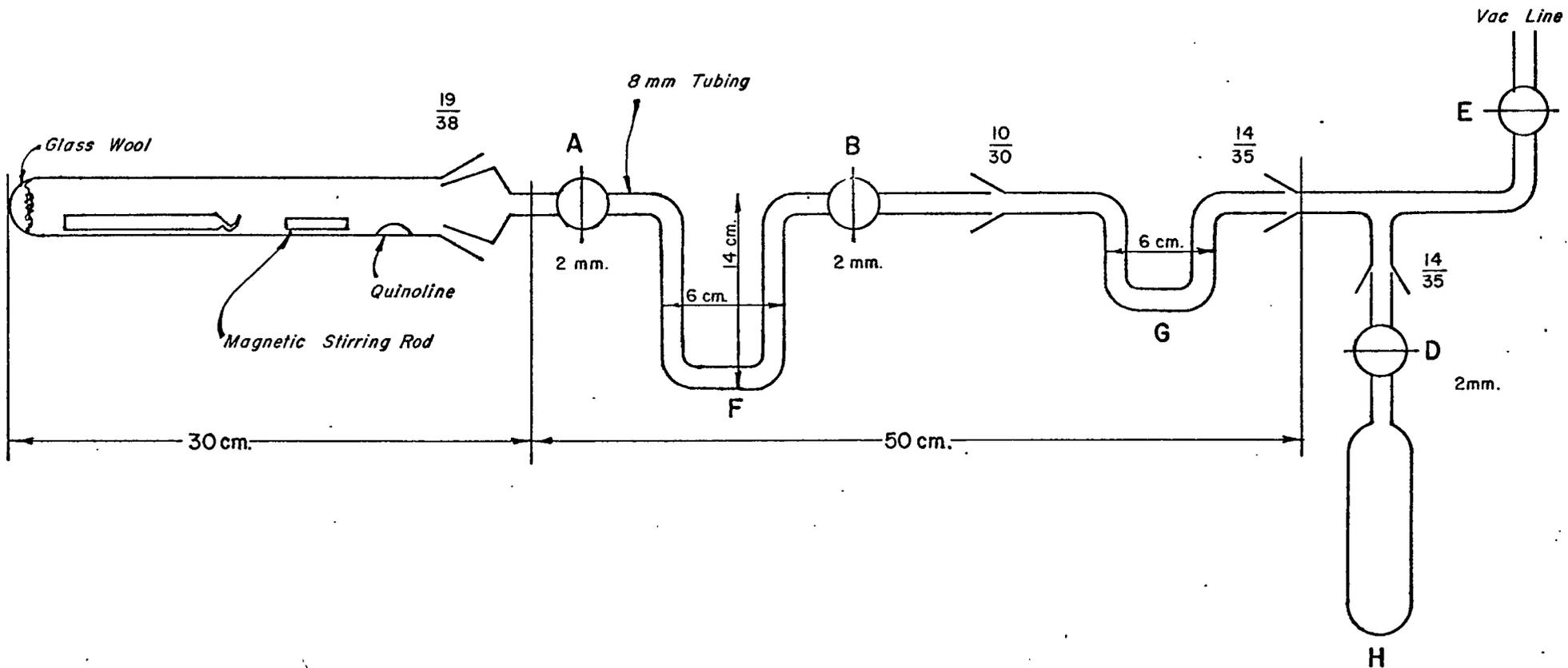
FIGURE 3 : Apparatus For Collection of CO<sub>2</sub>.
