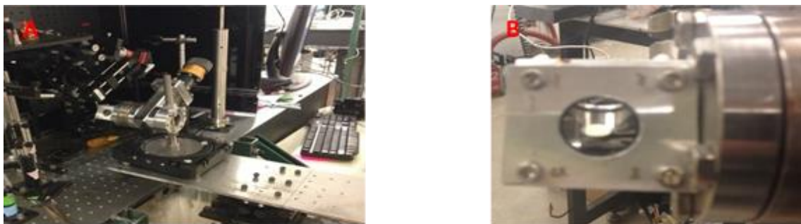
Figure 2-22: (A) SFG cell mounted on optical sample stage which is ready for SFG-imaging experiment. (B) SFG cell with polished platinum sample inside.
