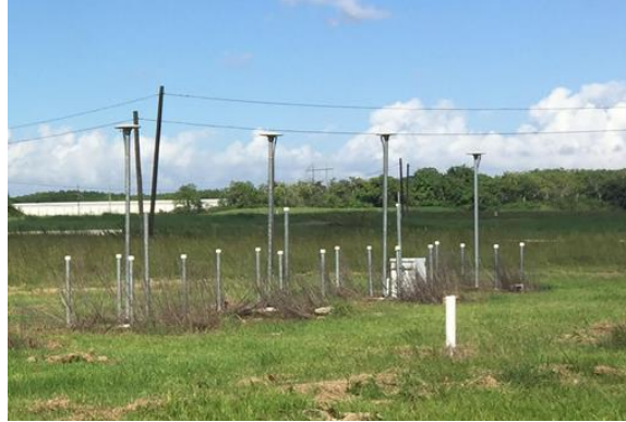
Figure 3-3: Site photo of UHCC Vertical GPS Array. From left to right: UHC1, UHC2, UHC3, and UHC0.
