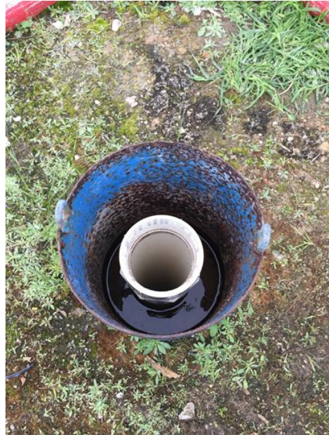
Figure 3-14: Field image of Blue well with Solinst water level meter Model 102 and inner PVC pipe.
