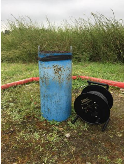
Figure 3-14: Field image of Blue well with Solinst water level meter Model 102 and inner PVC pipe.
