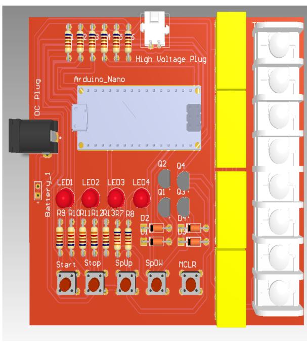
Figure 3. PCB of the control system
