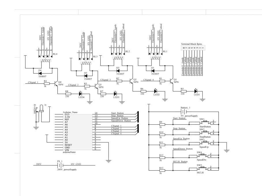
Figure 4. Schematic diagram of control system
