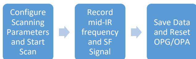
Figure 16: Logical flow of steps for SFG spectrum collection program.
