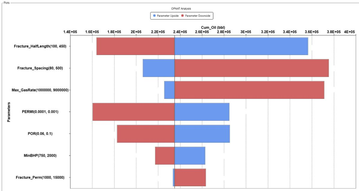
Figure 29. One parameter at a time sensitivity plot for cumulative oil
