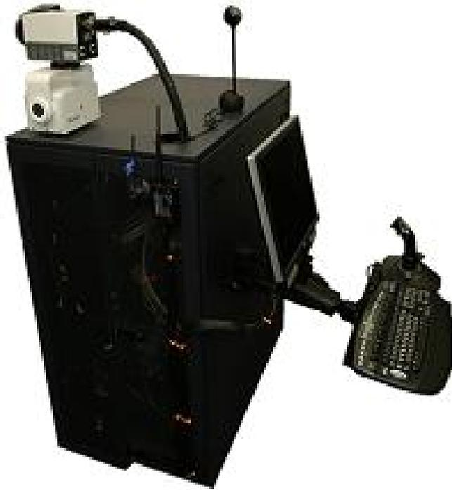
Figure 2.3: Custom thermal imaging system, ATHEMOS. The custom thermal imaging system developed by our group integrates a computer, a thermal camera, and several peripheral hardware components.
