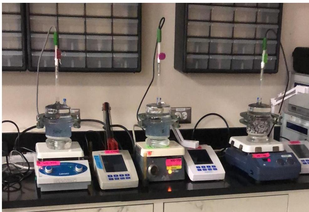
Figure 2.9 Spontaneous Water imbibition experimental set up.
