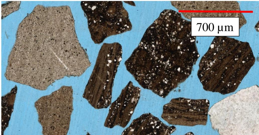
Figure 4.34 Bossier Formation Thin Section, B(60)700µm sample. Similar to the previous image, the fine particles observed in the smallest particle size are not present. Scale bar is the size of the particle size, in this case 700 µm.
