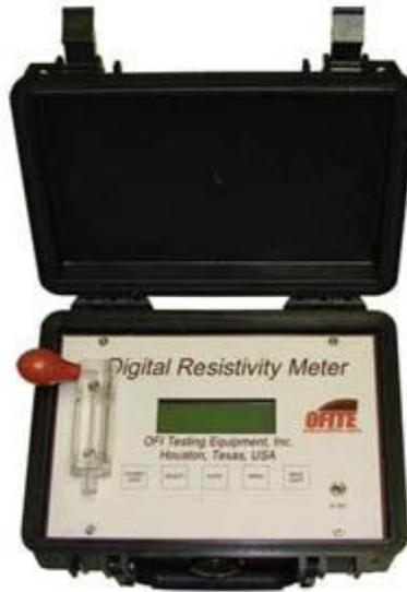
Figure 3-3: Direct resistivity measurement device
