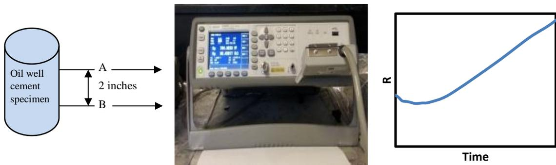
Figure 3-4: Typical components in the resistance measurements of the cement specimen
