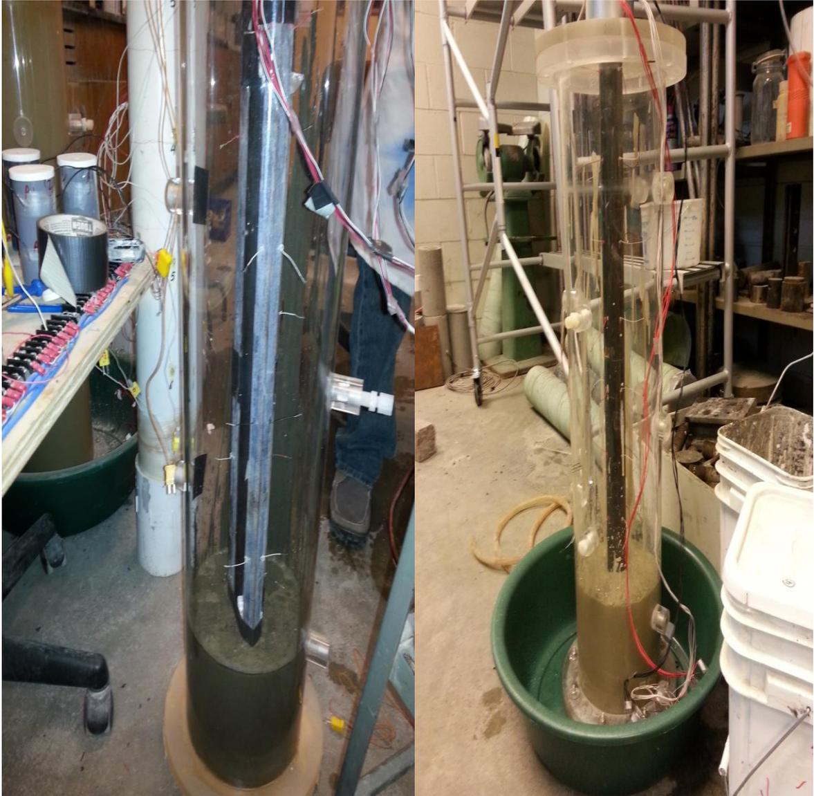
**Figure 3-10: The actual model with partially filled cement slurry (left) and drilling mud (right)**
