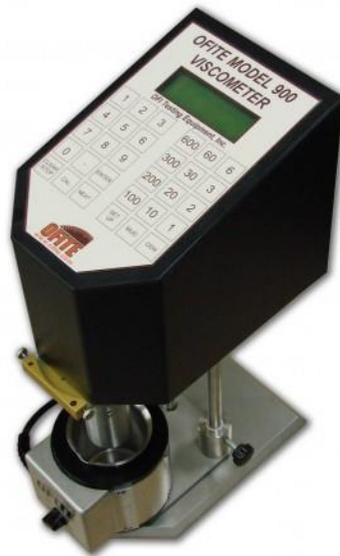
**Figure 3-2: Rotational viscometer used for rheological properties test**
