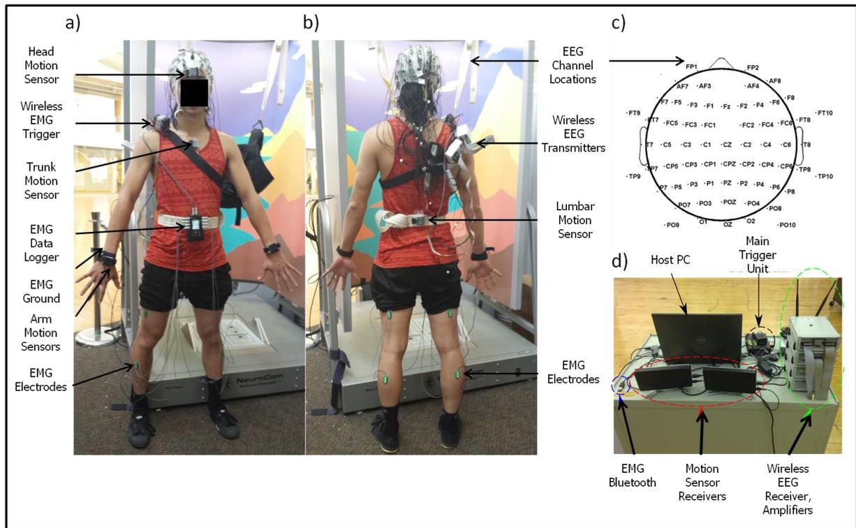
**Figure 3.1.** Data collection system mounted on a representative participant.
