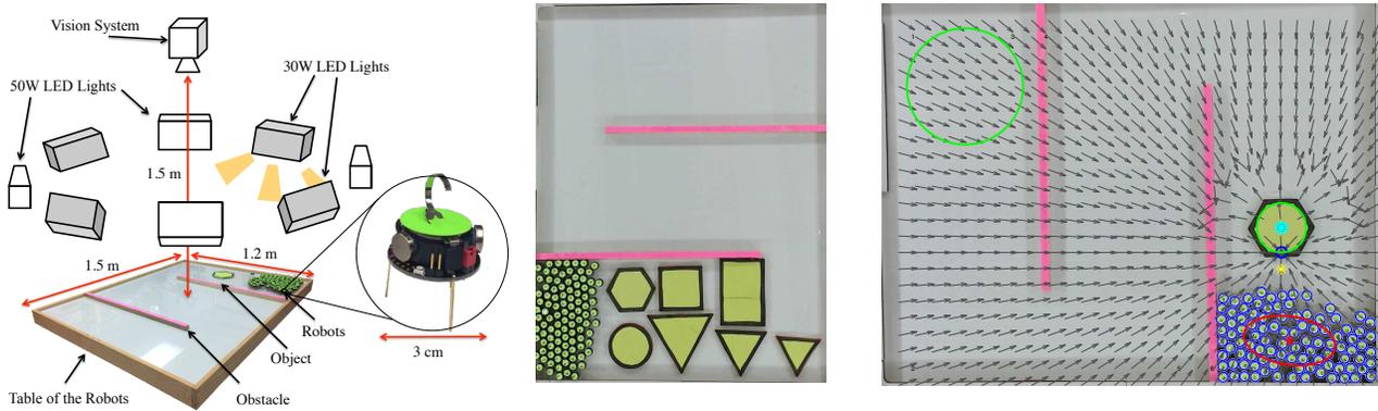
Fig. 19. Hardware platform. At right are the shapes used for hardware experiments and a visualization of the potential field.
