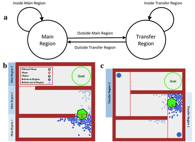
Fig. 13. Outlier rejection state machine and regions.
