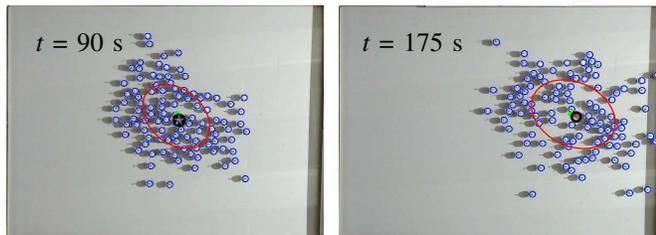
Fig. 20. Regulating mean  $x$  position of 100 kilobots using control law (11).
