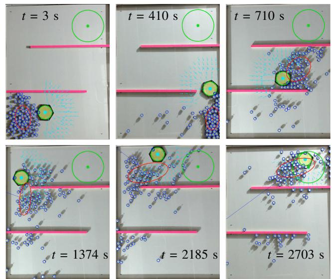
Fig. 21. Snapshots showing object manipulation experiment with 100 kilobots under automatic control. The automatic controller generates a policy to the goal, (see Extension 2).
