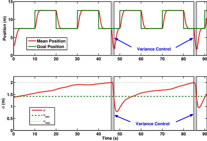
Fig. 10. Simulation result with 100 particles under hybrid control Alg. 1, which controls both the mean position (top) and variance (bottom). For ease of analysis, only  $x$  position and variance are shown.
