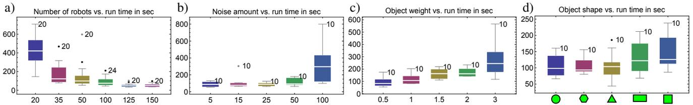
Fig. 18. Parameter sweep simulation studies for a) number of particles, b) different noise values, c) object weight, and d) object shape. Each bar is labelled with the number of trials. Completion time is in seconds.
