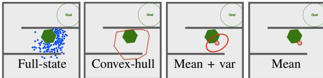
Fig. 4. Screenshots from task *Vary Visualization*. This experiment challenges players to quickly steer 100 particles (blue discs) to push an object (green hexagon) into a goal region. We record the completion time and other statistics.
