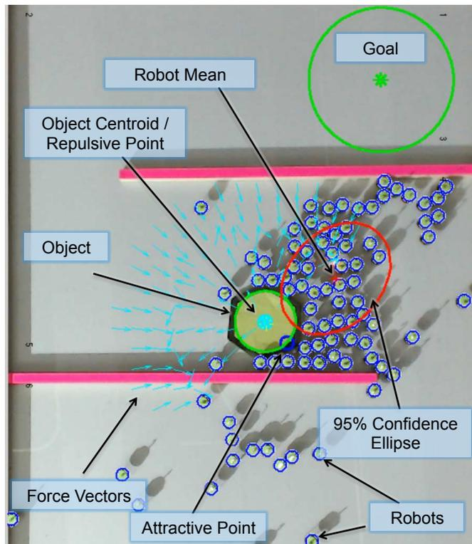
Fig. 1. A swarm of particles, all actuated by a uniform control input where each particle gets the same control input, can be effectively manipulated by a control law that uses only the mean and variance of the robot distribution. Here a swarm of particles (kilobot robots) pushes a green hexagon toward the goal (see video attachment).
