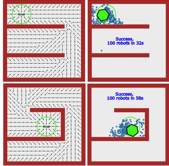
Fig. 16. We tested three workspaces. The control policies from value iteration for an E-shaped and a spiral workspace are shown in the left column.
