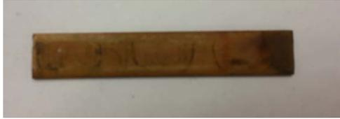
b. Corroded bar due to water and moisture at age of 35 days
