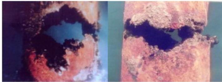
Figure 2.3 Casing failure due to severe corrosion
