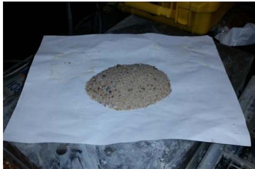
Figure 3.6 Sand used for polymer concrete specimens
