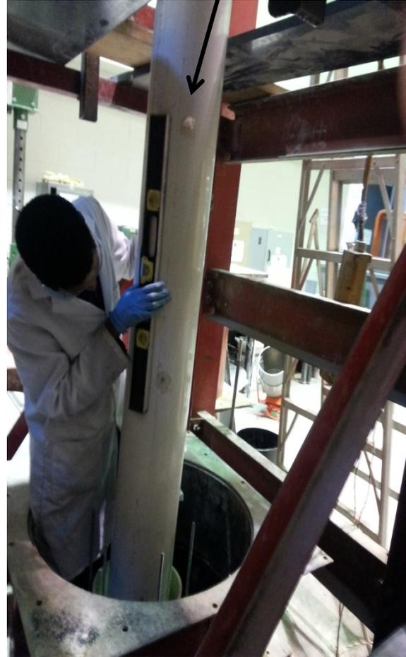
b. Casing embedded in PVC pipe
