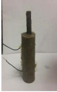
a. Corroded bar embedded
