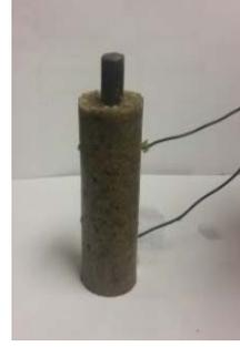
b. Non-corroded bar embedded
