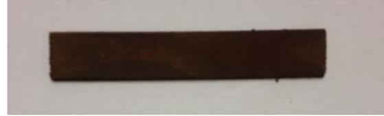
c. Corroded bar due to sulfuric acid at age of 56 days
