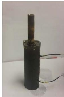
a. Corroded bar embedded
