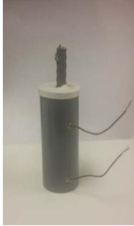
a. Corroded bar embedded
