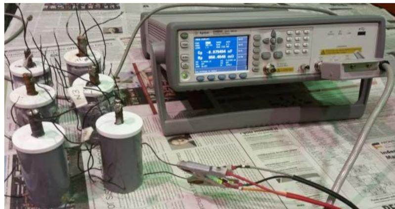
Figure 3.8 LCR meter device
