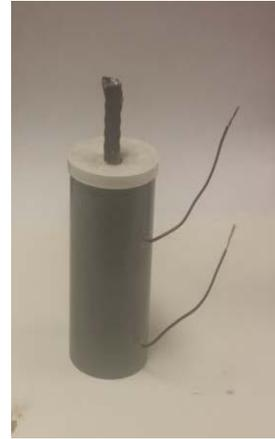
b. Non-corroded bar embedded
