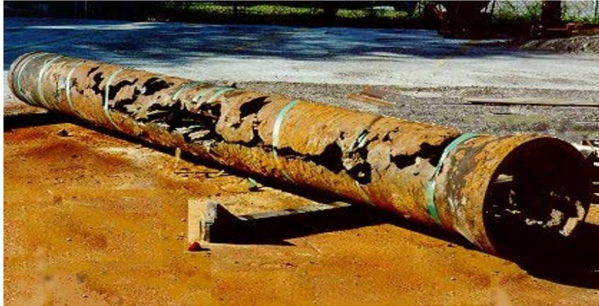
Figure 2.2 Pipeline failure due to severe corrosion
