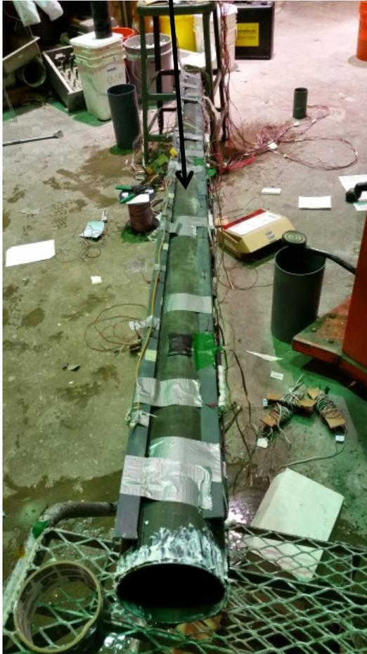
a. Steel casing pipe with instrumentation
