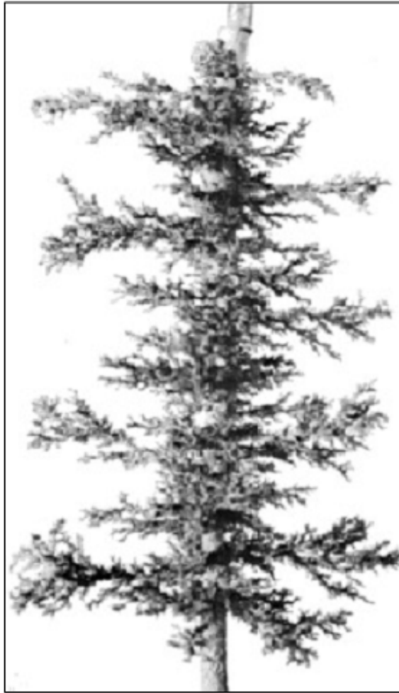
Figure 6.6: Wormholes created by injecting water through a radial core (of diameter 2 mm and length 50 mm) made of plaster (Daccord, 1987).
