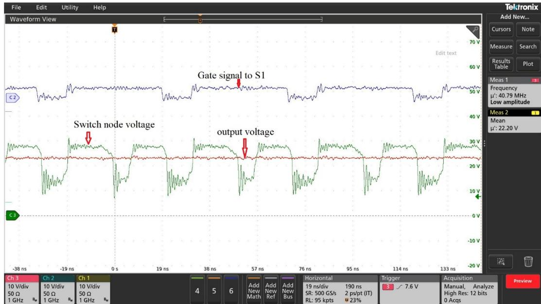
Figure 2-17: Experimental results of the FCTL converter at the duty cycle of 0.75 with 30 V input DC supply. The gate pulses to the top side devices are at 20 MHz and interleaved by an angle of  $180^\circ$ . The switch node voltage switching between 15 V and 30 V with twice the device switching frequency at 40 MHz.
