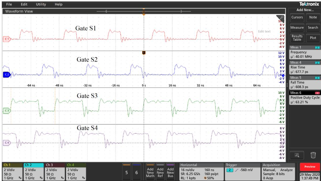
Figure 3-10: Gate pulses measured at 40 MHz (X-axis:16ns/div).
