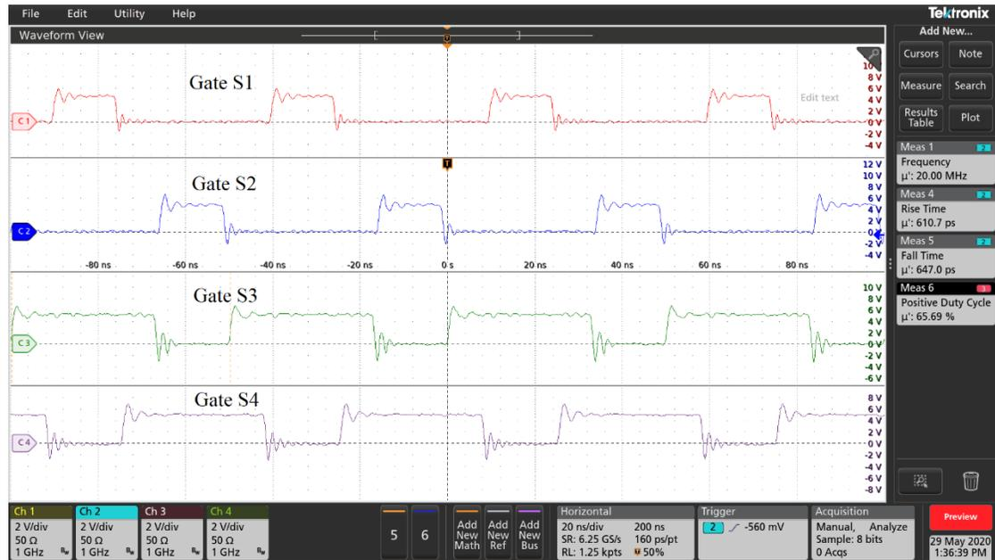
Figure 3-9: Measured gate pulses of the proposed gate drive technique at 20 MHz. Gate pulses to  $S_1$  and  $S_4$  are complementary. Gate pulses to  $S_2$  and  $S_3$  are complementary (x-axis:20ns/div).
