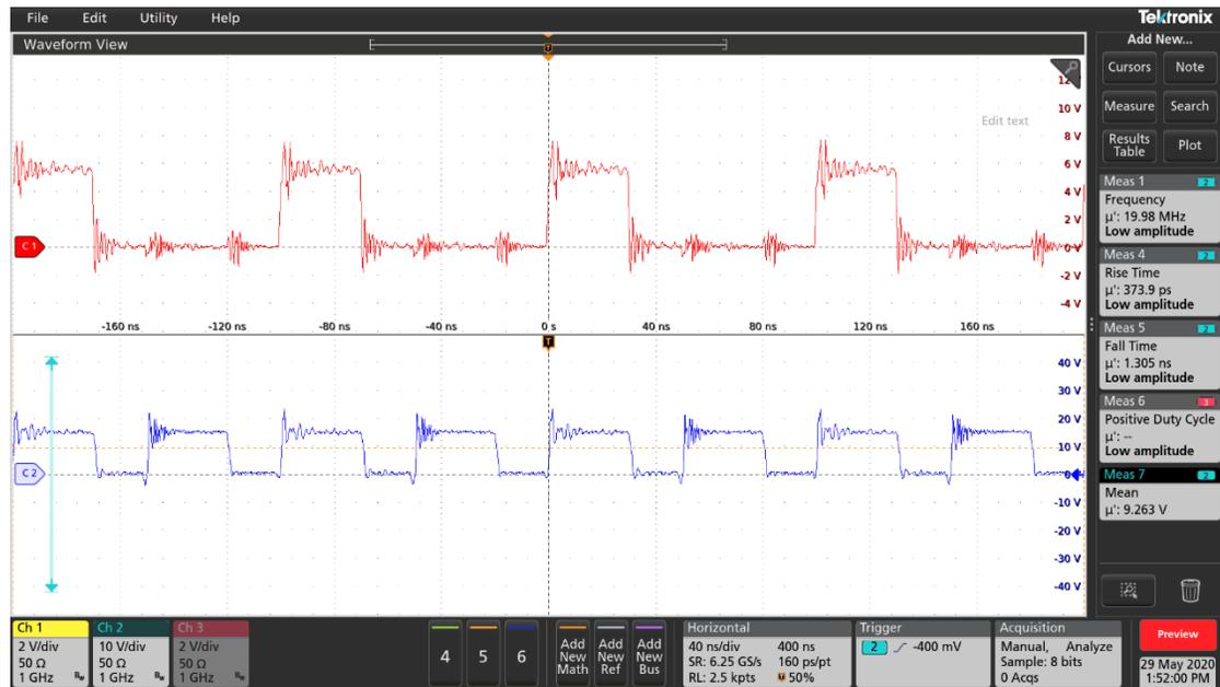
Figure 3-14: Experimental waveforms. Ch1: Gate signal. Ch2: Switch node voltage. The frequency of switch node voltage (40 MHz) is double the gate signal switching frequency (20 MHz).
