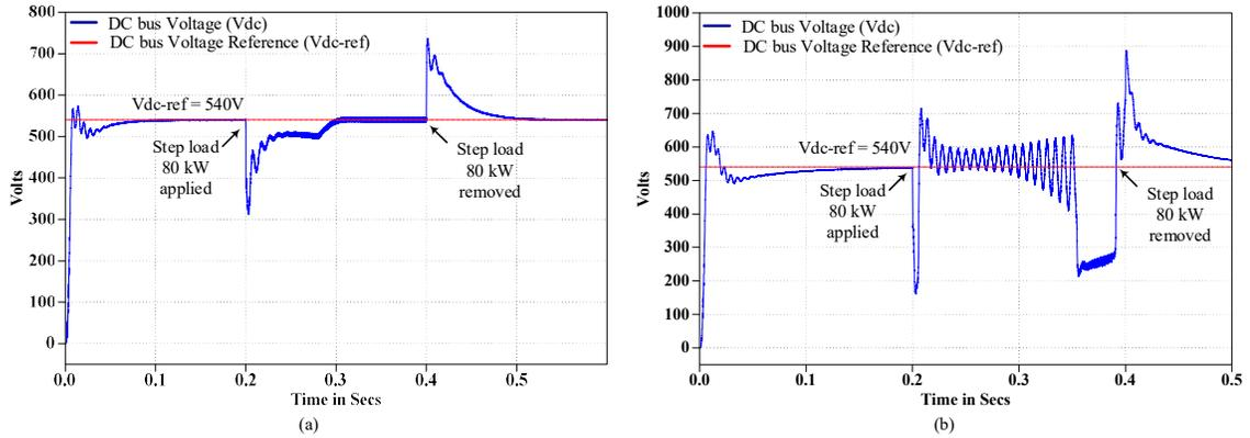
Fig. 5.12: DC-link voltage regulation of BSG based DRI regulated AC VSCF system during 80kW step load: (a) With EMI filters; (b) Without EMI filters.
