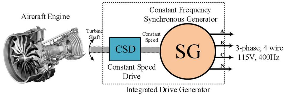
Fig. 1.2: Integrated Drive Generator (IDG) based 115V 400Hz AC system.
