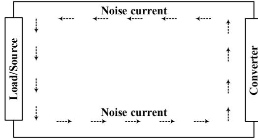
Fig. 5.4: Differential mode noise in the PEC system that flows from converter to load/source.
