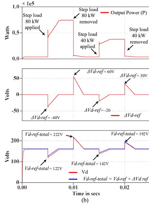
Fig. 3.13: AIVR algorithm for four-leg inverter control: (a) Flowchart of the AIVR algorithm; (b) Four-leg inverter control DQ0 axes voltages during 80kW & 40kW step load.
