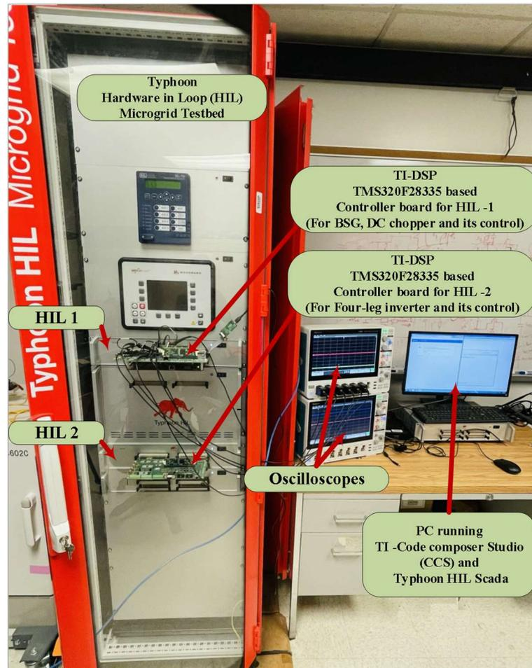
Fig. 3.15: C-HIL test set up.
