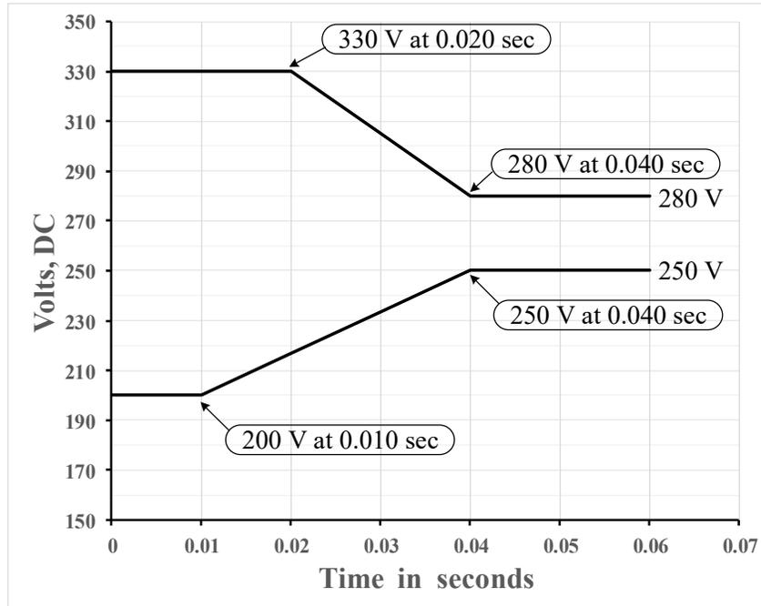
Fig. 2.2: MIL-STD-704 transient voltage specifications for 270V DC system [23].
