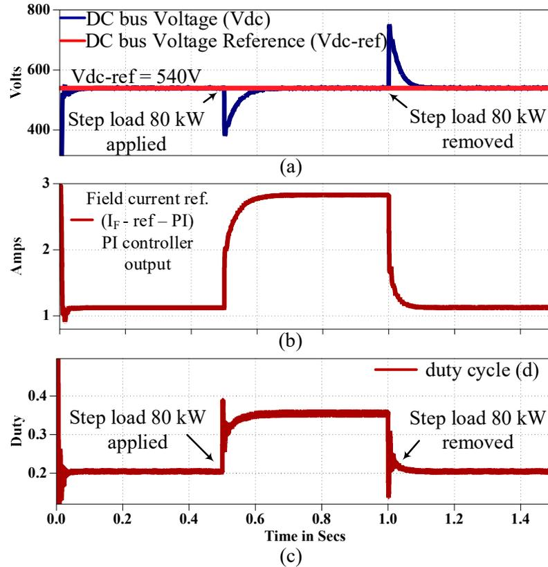
Fig. 3.6: Transient response of the DC chopper control during step change in DC load (80kW): (a) DC-link voltage; (b) Exciter field current; (c) Duty cycle.
