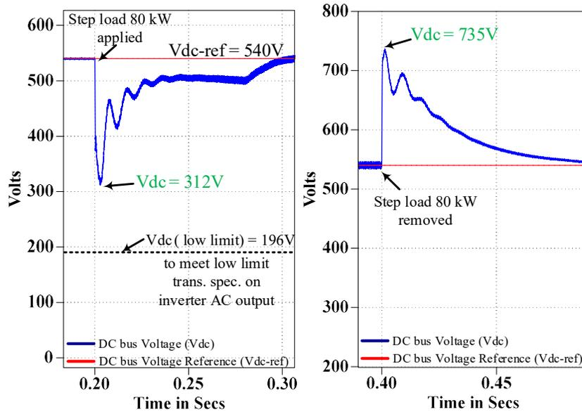
Fig. 3.14: (a) DC-link voltage of the VSCF system during step load 80kW with proposed control improvements on both four-leg inverter and BSG side with  $100\mu\text{F}$  DC-link capacitance.
