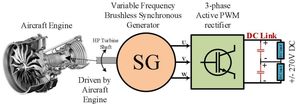
Fig. 1.10: VFG based active rectifier regulated +/-270V DC power system.
