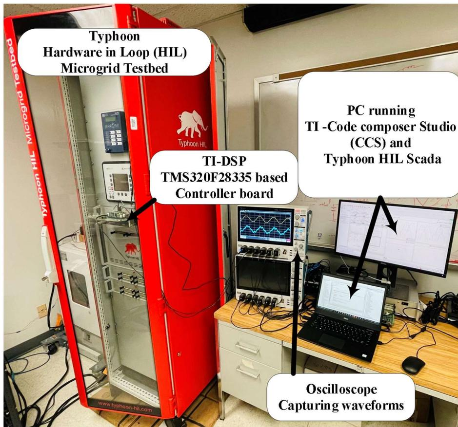
Fig. 4.3: C-HIL test set up.
