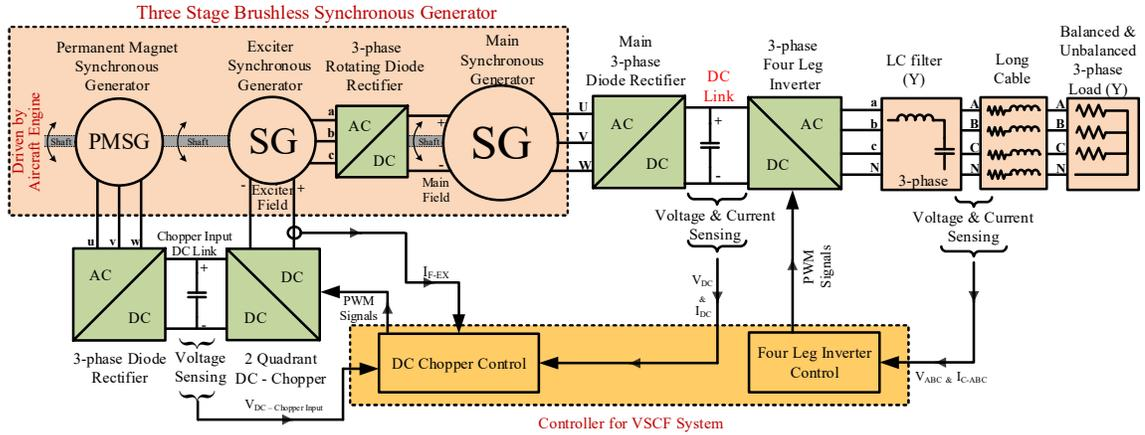
Fig. 3.2: Block diagram of a BSG based VSCF aircraft AC power system.
