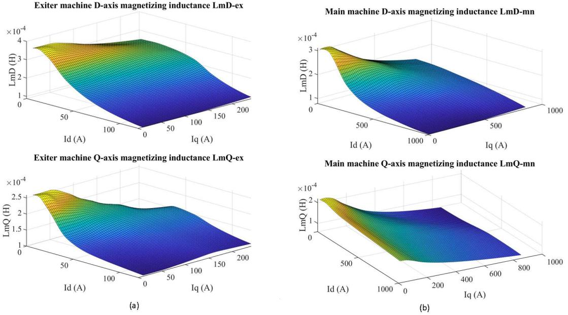
Fig. 3.16: DQ-axis currents vs magnetizing inductance: (a) Exciter SG; (b) Main SG.
