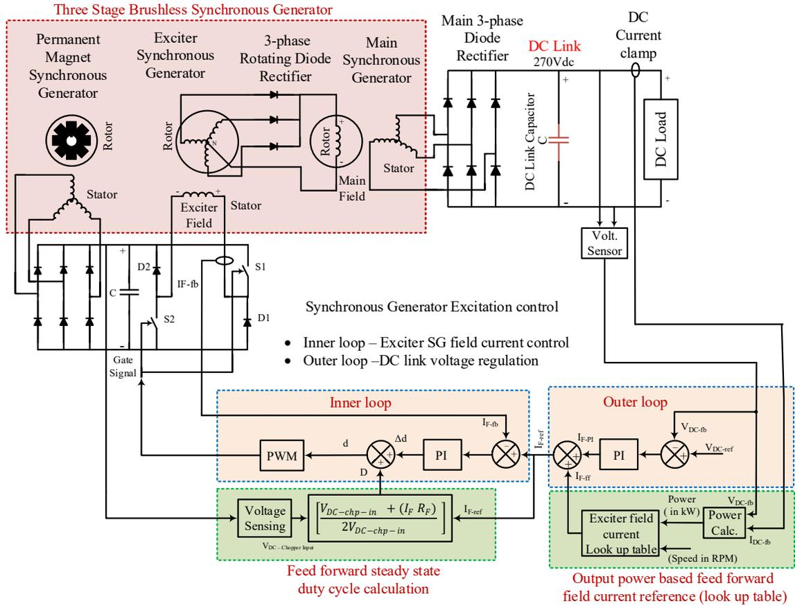
Fig. 2.7: Control block diagram of the exciter field current control and DC-link voltage regulation with feedforward compensation.
