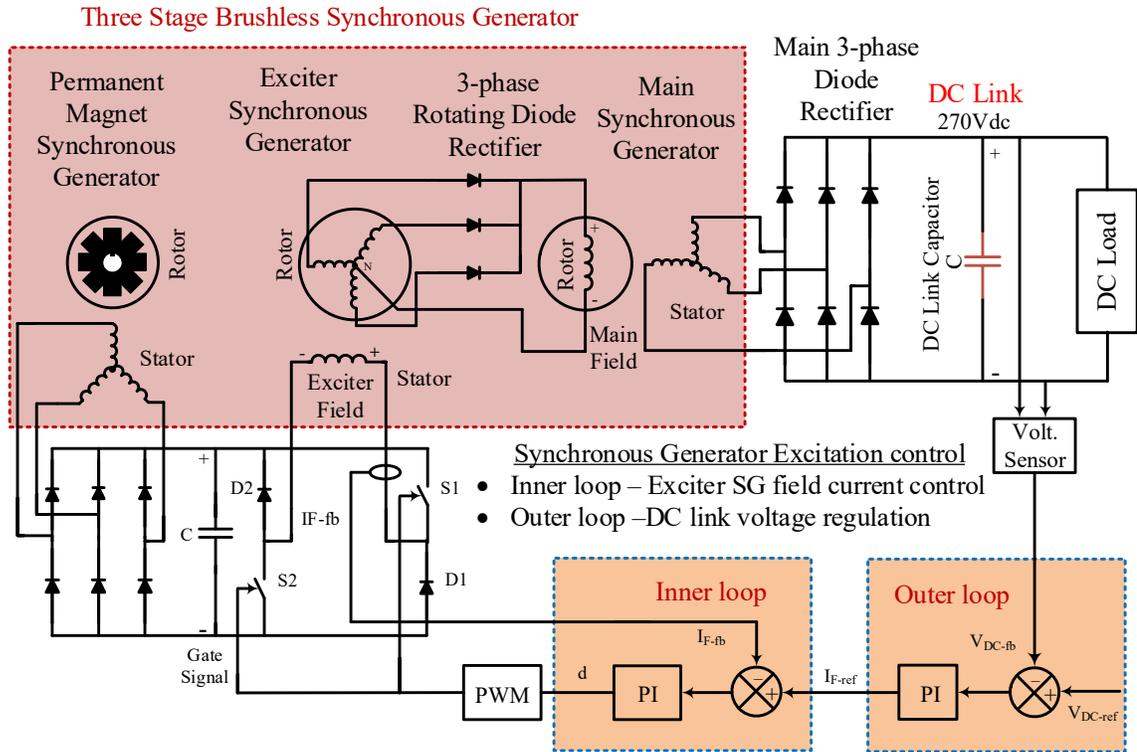
Fig. 2.3: Control block diagram of the DC-link voltage regulation and exciter SG field current control using two-quadrant DC chopper.
