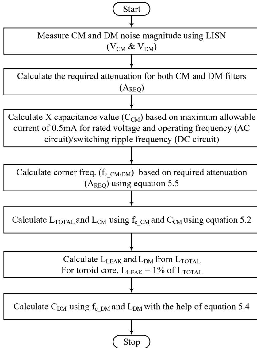
Fig. 5.10: EMI filter design procedure.
