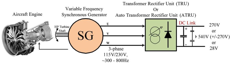
Fig. 1.8: VFG based ATRU/TRU regulated +/-270V DC power system.
