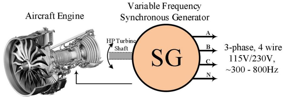
Fig. 1.3: Variable Frequency AC power generation system in MEA.
