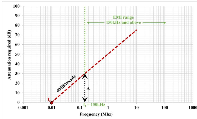
Fig. 5.6: Corner ( $f_c$ ) and cut-off ( $f_1$ ) frequency for a first order CM and DM filter with attenuation rate 40dB/decade for the required attenuation of  $A_{REQ}$ .
