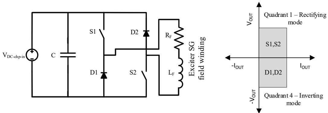
Fig. 2.4: Class D two-quadrant DC chopper.
