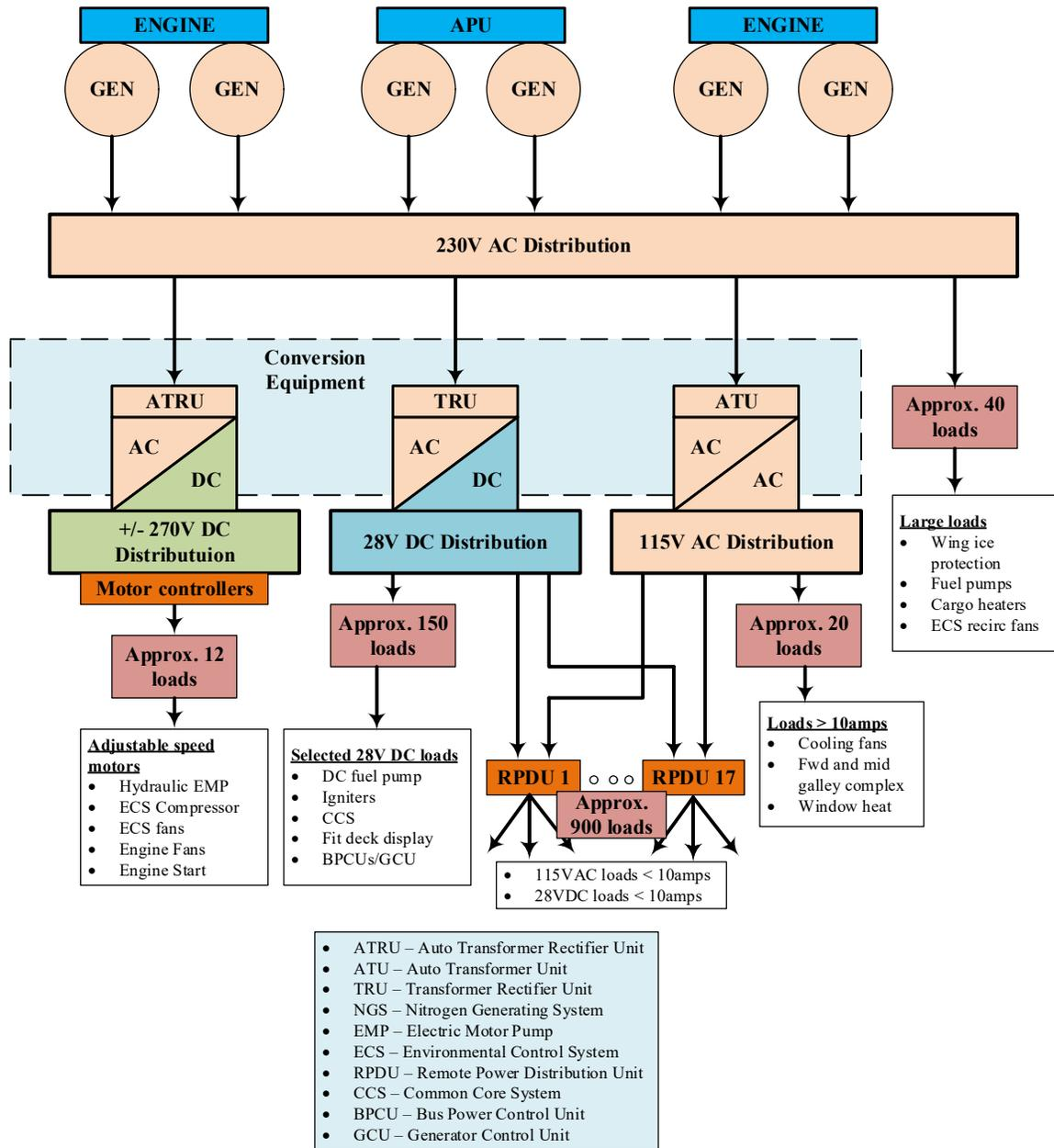
Fig. 1.4: EPS architecture of Boeing 787 [6].
