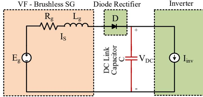
Fig. 3.3: Simplified equivalent circuit model of the VFG connected DRI system with DC-link capacitance.
