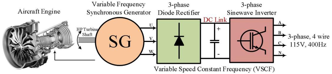
Fig. 1.5: VFG based DRI regulated 115V, 400Hz VSCF system with DC-link.
