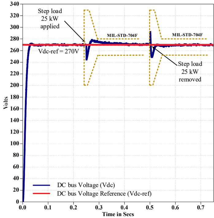
Fig. 2.8: DC-link voltage regulation waveform for 600µF DC-link capacitance when feedforward compensation is enabled for 25kW step load at 7000rpm.
