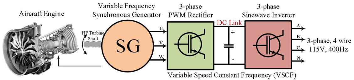
Fig. 1.7: VFG based active rectifier regulated 115V, 400Hz VSCF system with DC-link.
