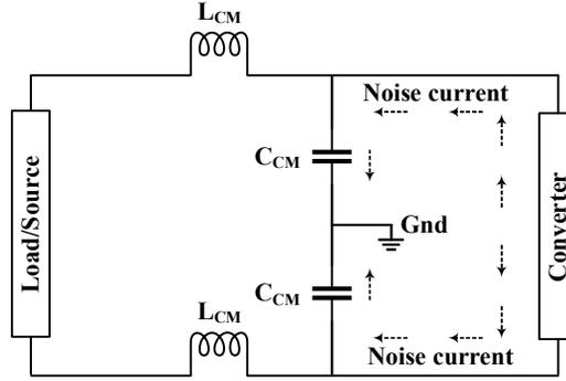
Fig. 5.3: LC common mode noise filter configuration.
