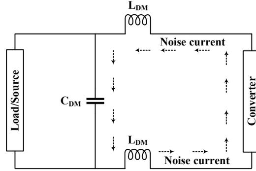
Fig. 5.5: LC differential mode noise filter configuration.
