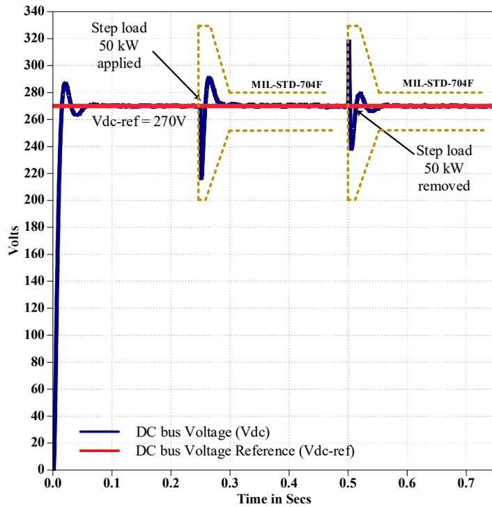
Fig. 2.9: DC-link voltage regulation waveform for 600µF DC-link capacitance when feedforward compensation is enabled for 50kW step load at 14000rpm.
