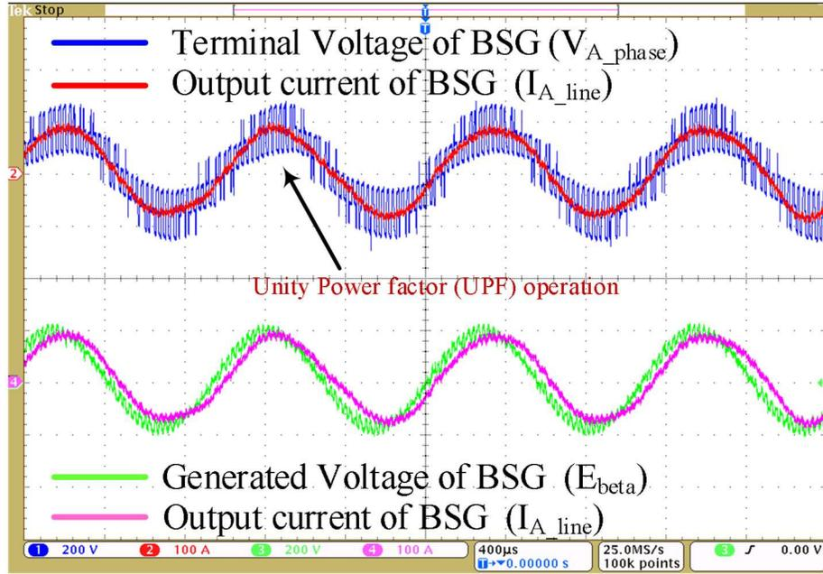
Fig. 4.9: Generated EMF, terminal voltage, and output current of BSG during steady-state operation with UPF for 25kW load at speed 7000rpm with proposed control improvements.
