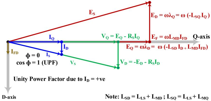
Fig. 4.10: Steady-state phasor diagram during FOC of Main SG when  $I_D$  is positive.
