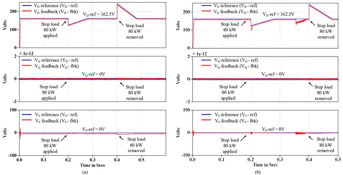
Fig. 5.13: DQO axes four-leg inverter output regulation of BSG based DRI regulated AC VSCF system during 80kW step load: (a) With EMI filters; (b) Without EMI filters.
