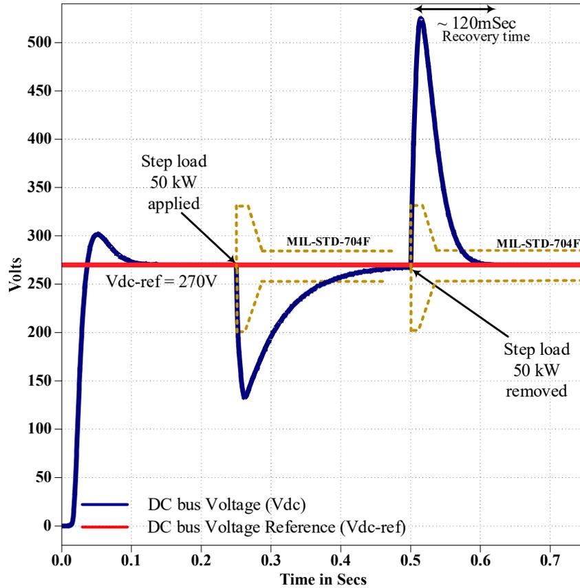
Fig. 2.6: DC-link voltage regulation waveform for 2500 $\mu$ F DC-link capacitance without any control improvements for 50kW step load at 14000rpm.
