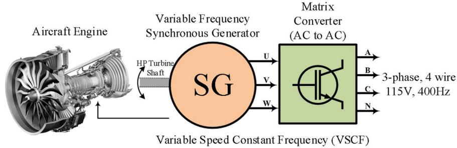
Fig. 1.6: VFG based cycloconverter or matrix converter regulated 115V, 400Hz VSCF system without DC-link.
