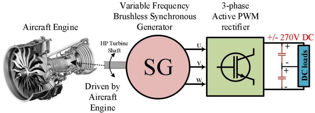
Fig. 4.1: Block diagram of a Brushless SG based Active rectifier regulated aircraft DC power system.
