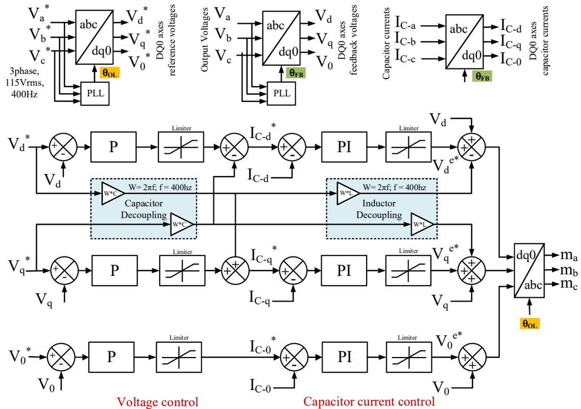
Fig. 3.8: Output voltage control and capacitor current control of four-leg inverter.
