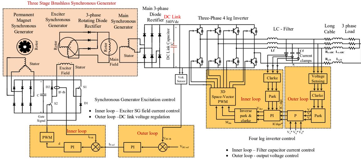
Fig. 3.5: Control block diagram of the DC-link based DRI VSCF system.
