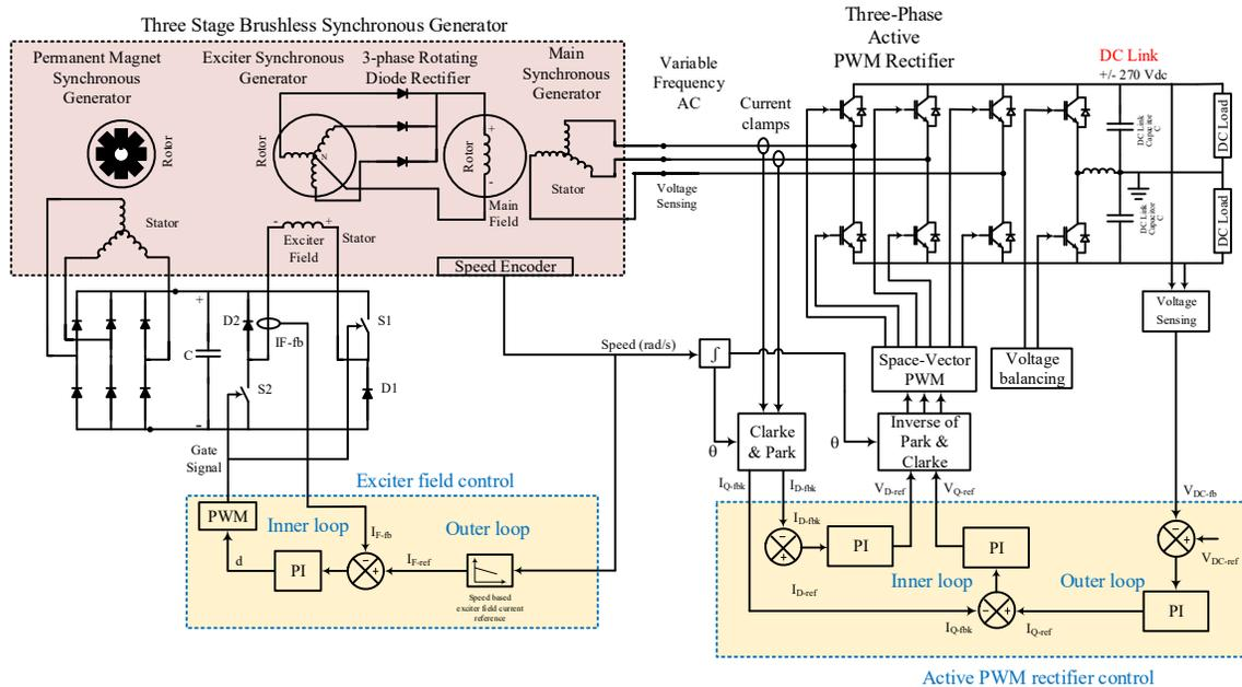
Fig. 4.2: Control block diagram of BSG based active rectifier regulated aircraft DC power system.
