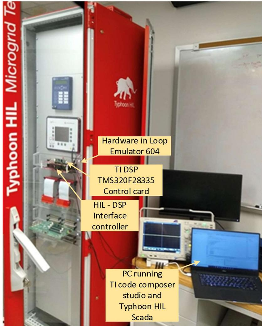
Fig. 2.11: Controller Hardware-In-Loop (C-HIL) real-time simulation testbed.
