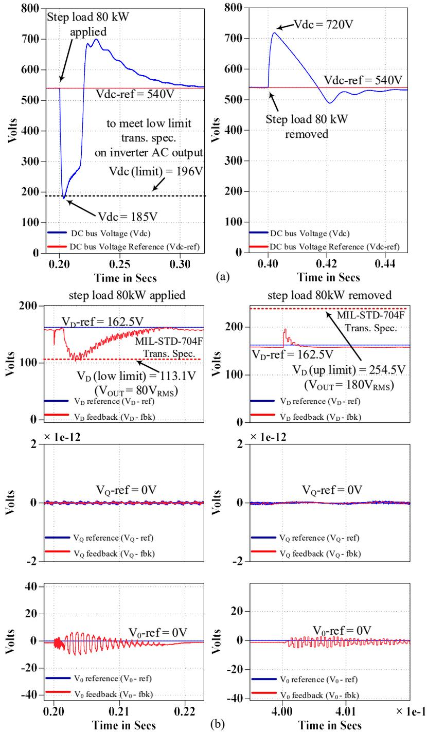
Fig. 3.12: 80kW step load response of the VSCF system with BSG side improvements with 400 $\mu$ F DC-link capacitance: (a) DC-link voltage; (b) Inverter DQO axes voltages.
