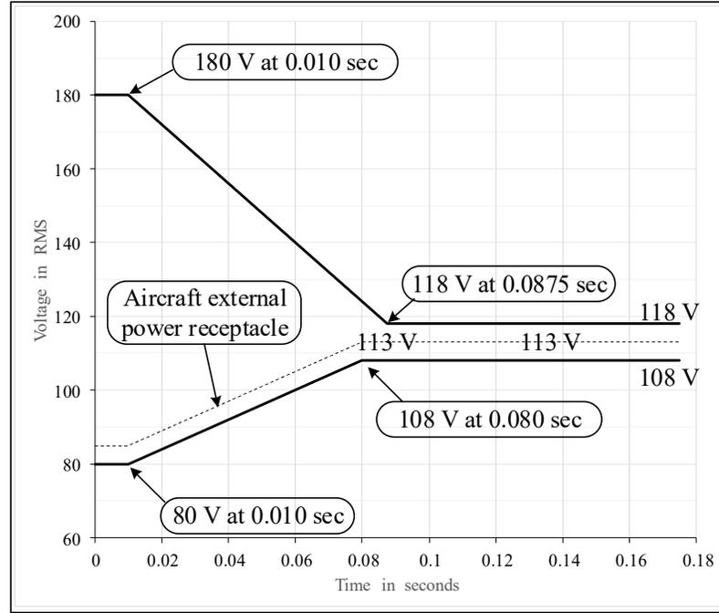
Fig. 3.4: MIL-STD-704F AC voltage transient limits [23].
