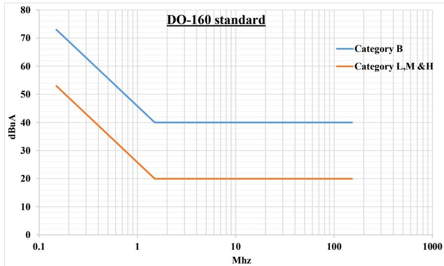
Fig. 5.1: RTCA/DO-160G: Standard test conditions for avionics electronic hardware in airborne systems.
