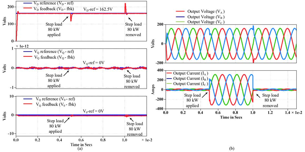
Fig. 3.9: Transient step load response of the four-leg inverter: (a) DQ0 axes voltages; (b) Inverter output voltages and currents.
