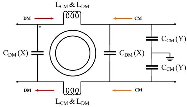
Fig. 5.9: Complete CM and DM EMI filter using toroidal core and XY capacitors.
