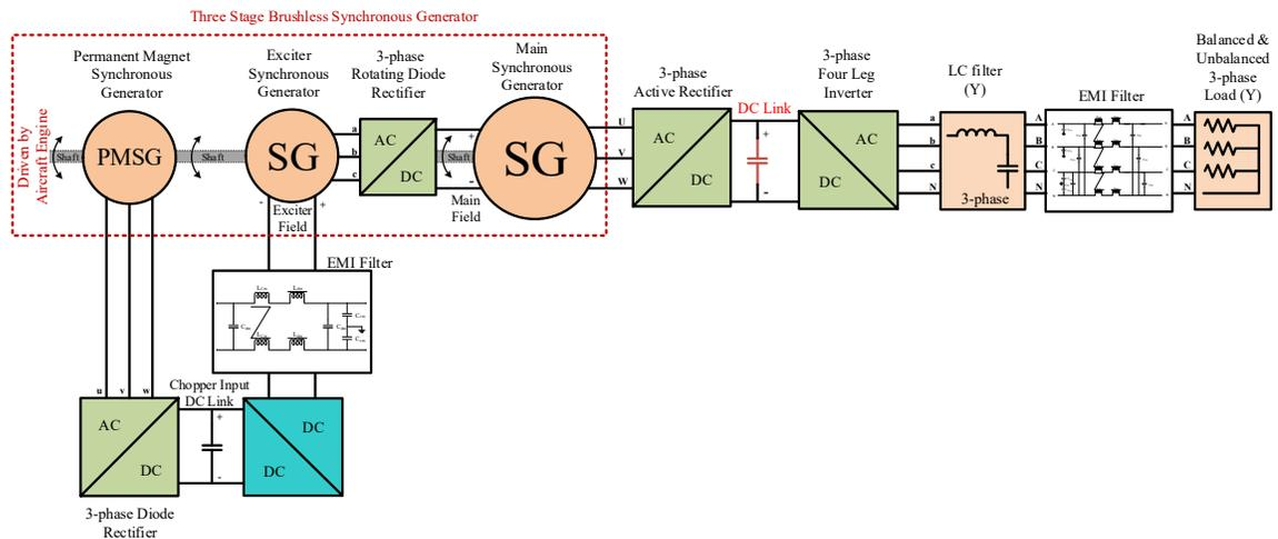
Fig. 5.11: BSG based DRI regulated AC VSCF system along with EMI filters.
