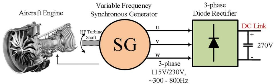
Fig. 1.9: VFG based diode rectifier regulated 270V DC power system.
