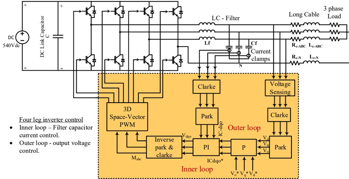
Fig. 3.7: Block diagram of the four-leg inverter and its voltage mode control.
