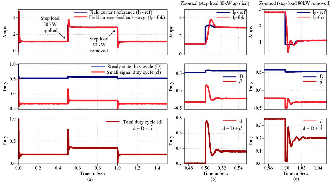
Fig. 2.10: (a) Exciter field current control transient response for 50kW step load during 14000rpm when feedforward compensation is enabled; (b) During step load 50kW is applied; (c) During step load 50kW is removed.
