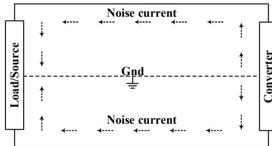
Fig. 5.2: Common mode noise in the PEC system that flows from converter to load/source.
