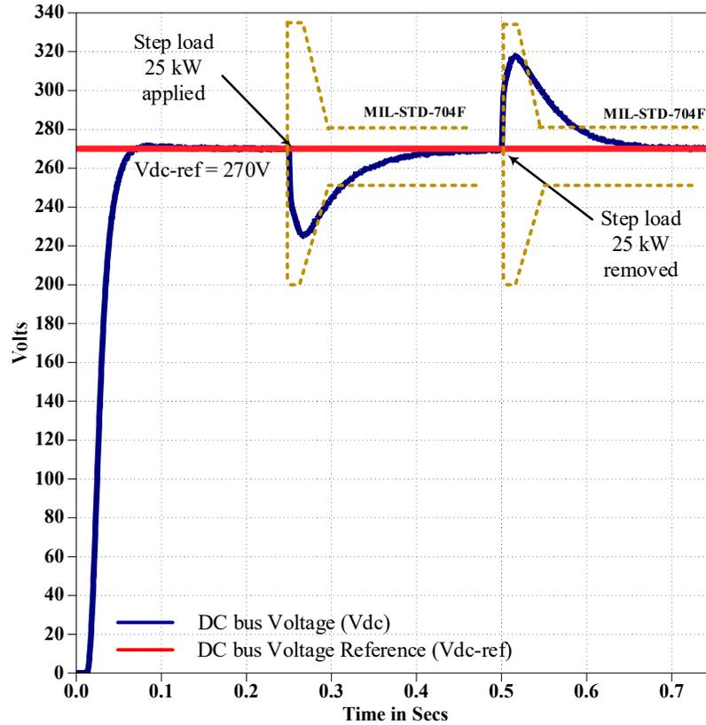
Fig. 2.5: DC-link voltage regulation waveform for 2500 $\mu$ F DC-link capacitance without any control improvements for 25kW step load at 7000rpm.
