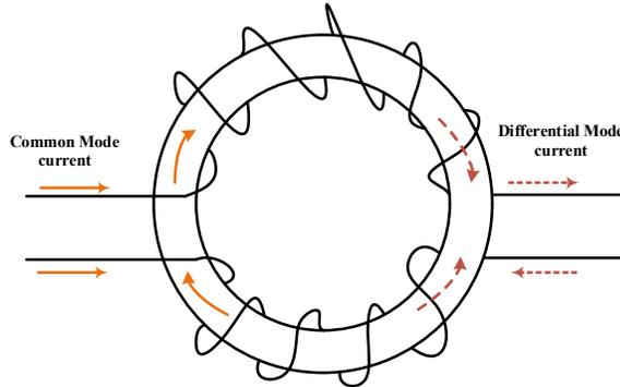
Fig. 5.7: Toroidal inductor core for both CM and DM Filter.
