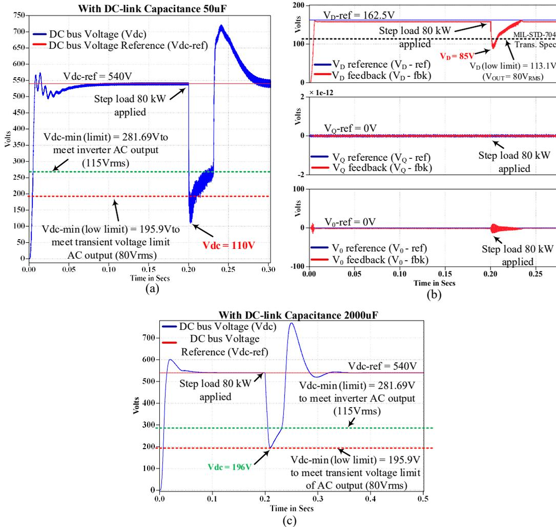
Fig. 3.10: Transient step load response of the VSCF system: (a) DC-link voltage regulation for 50µF DC-link capacitance; (b) Inverter - DQ0 axes voltages for 50µF DC-link capacitance; (c) DC-link voltage regulation for 2000µF DC-link capacitance.
