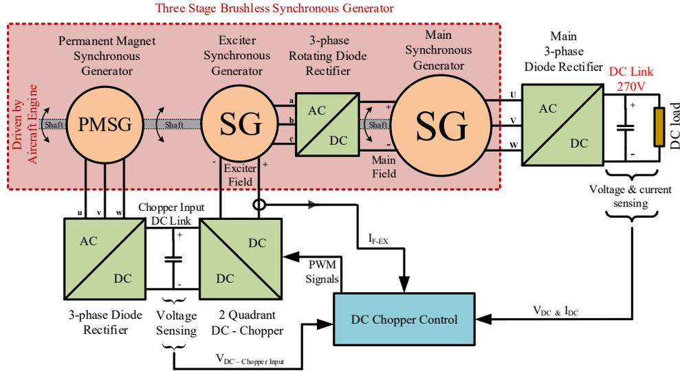
Fig. 2.1: Block diagram of the BSG based 270V DC power system.
