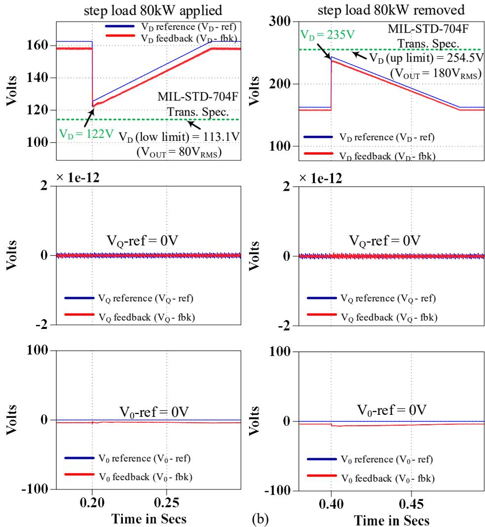
Fig. 3.14: (b) Four-leg inverter DQO axes voltages of the VSCF system during step load 80kW with proposed control improvements on both four-leg inverter and BSG side with  $100\mu\text{F}$  DC-link capacitance.
