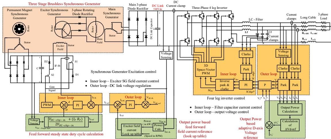
Fig. 3.11: Block diagram of the proposed controller for the DC-link based VSCF system. inverter control to improve the transient response at the DC-link for step loads at the inverter output. The proposed control methods are explained in detail in Section 3.5.
