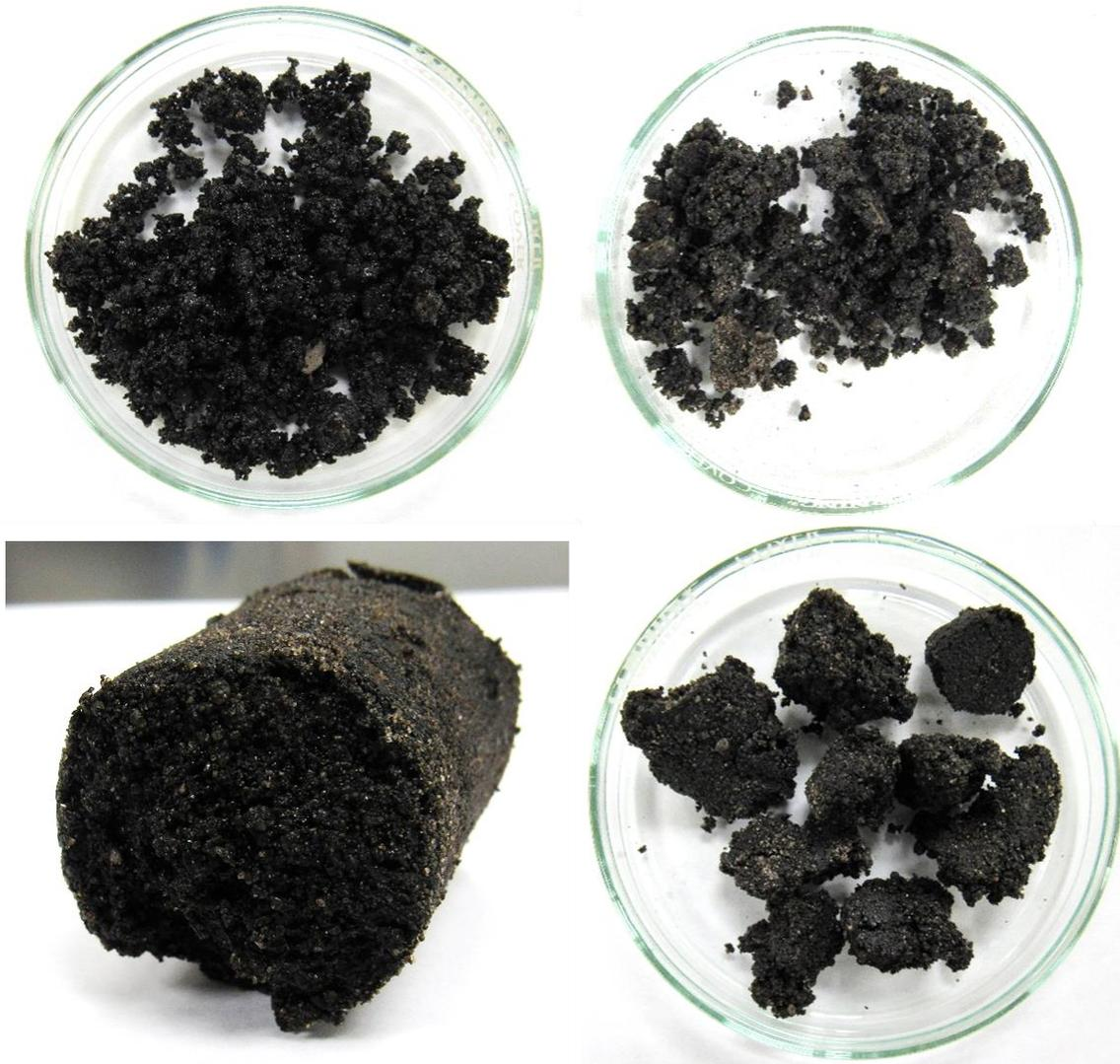
Figure 6-34: Top left – original sand sample, top right – inlet sand sample after test, bottom left – side view of outlet sand sample, and bottom right – top view of outlet sand sample
