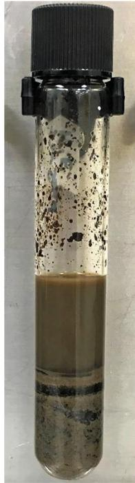
Figure 6-24: Static test result for oil sand mixed with 0.25 wt.% C20-24 IOS, 0.25 wt.% C13 13 PO sulfate, 1 wt.% 2-butanol and 0.5 wt.% sodium carbonate
