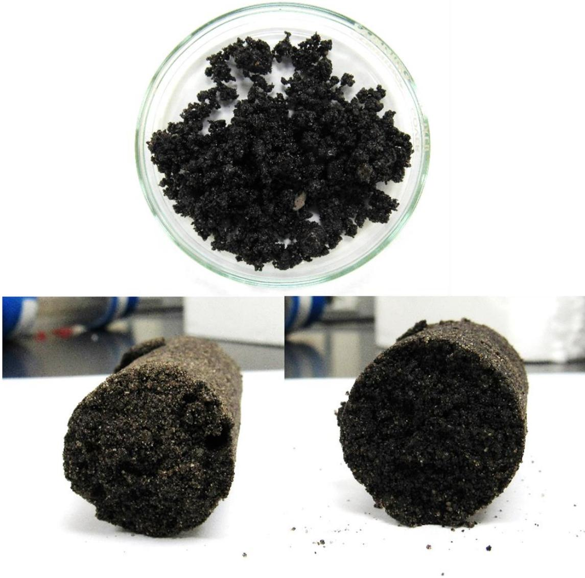
Figure 6-36: Top – Original oil sand, Bottom left – Inlet sand, and Bottom right – Outlet sand
