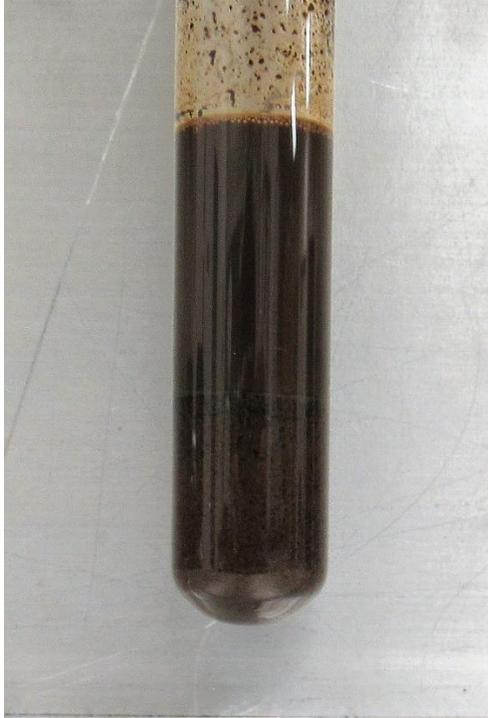
Figure 6-27: Static test for 1 wt.% C20-24 IOS and 1 wt.% C13 13 PO alcoxy sulfate, 1 wt.% TEGMBE, and 4 wt.%  $\text{Na}_2\text{CO}_3$
