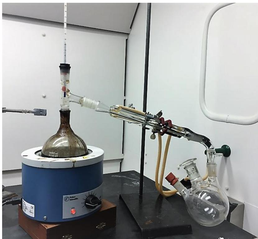
Figure 5-3: Solvent recovery setup
