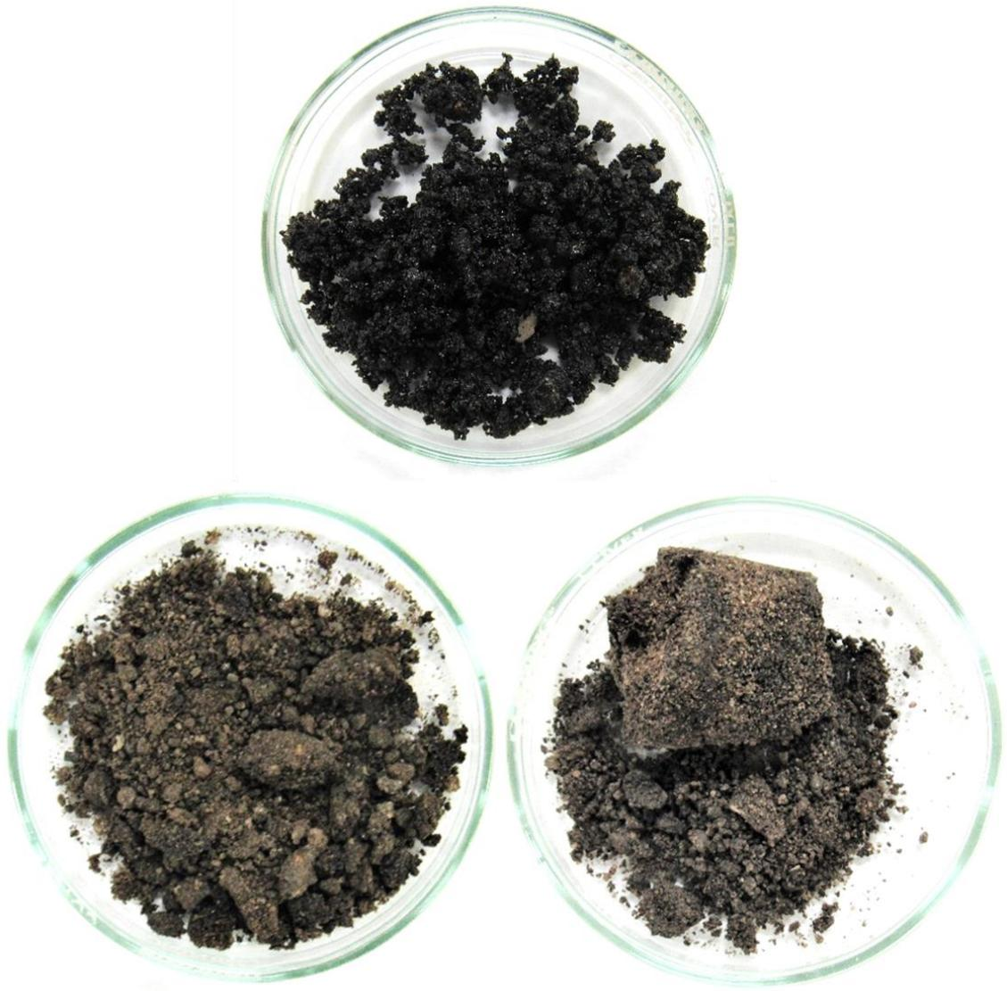
Figure 6-32: Top – Original sand sample, bottom left – Inlet sand sample after test, and bottom right outlet sand sample after test
