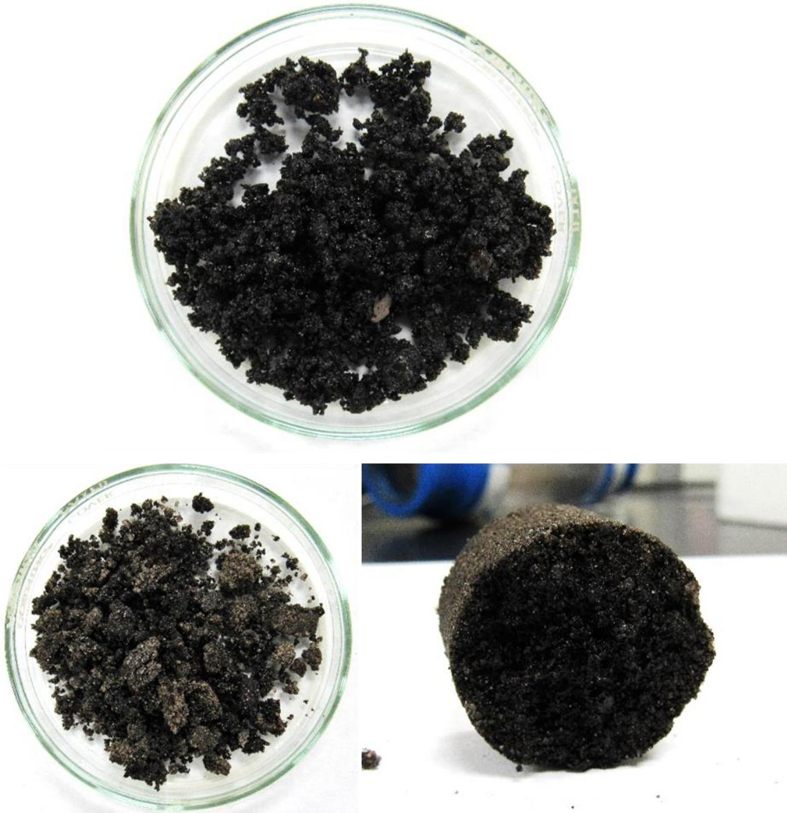
Figure 6-37: Top - original oil sand, bottom left – Inlet sand, and bottom right – outlet sand
