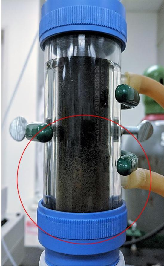
Figure 6-29: Picture of the flow setup during the test. Notice the microemulsion moving through the column, circled in red
