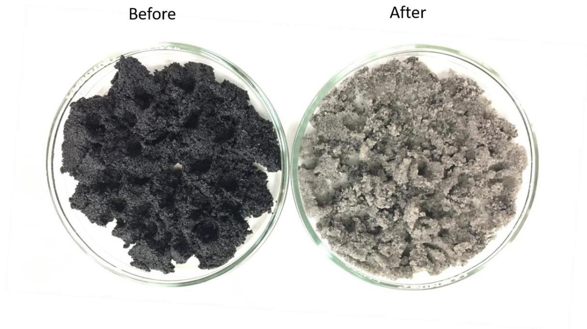
Figure 6-13: Comparison of sand (OK-75) before and after the flow experiment
