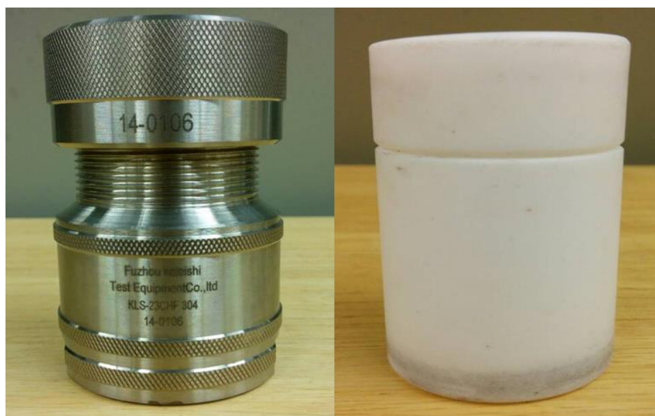
Figure 2.1. Left : Stainless steel autoclave. Right : Teflon liner.
