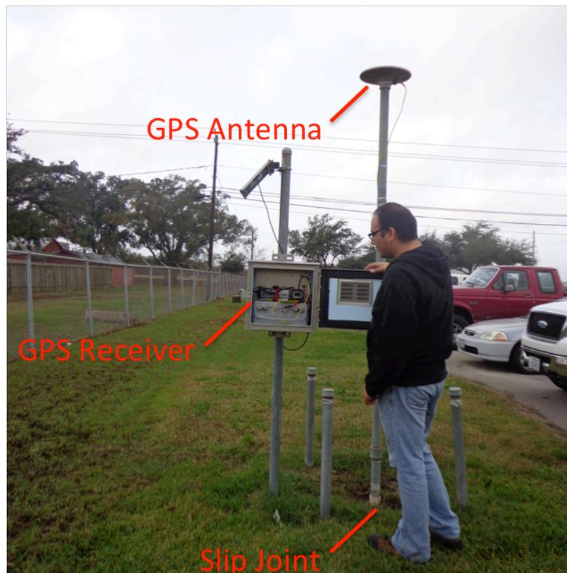
**Figure 4-1 PAM Station Set-up.**
