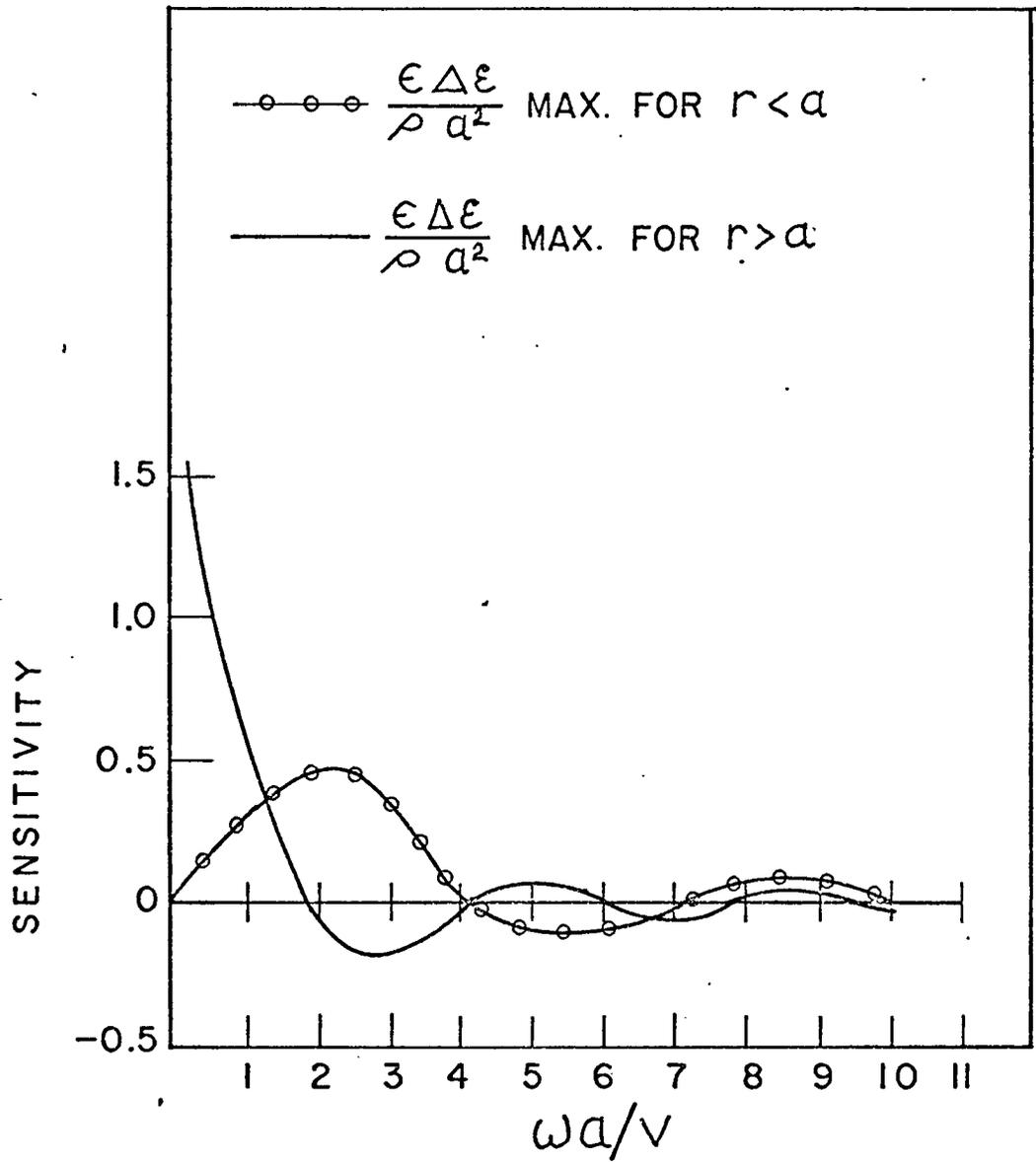
Figure 5. The sensitivity of the test ion energy to the electric fields in the regions  $r > a$  and  $r < a$  vs  $x$ .
