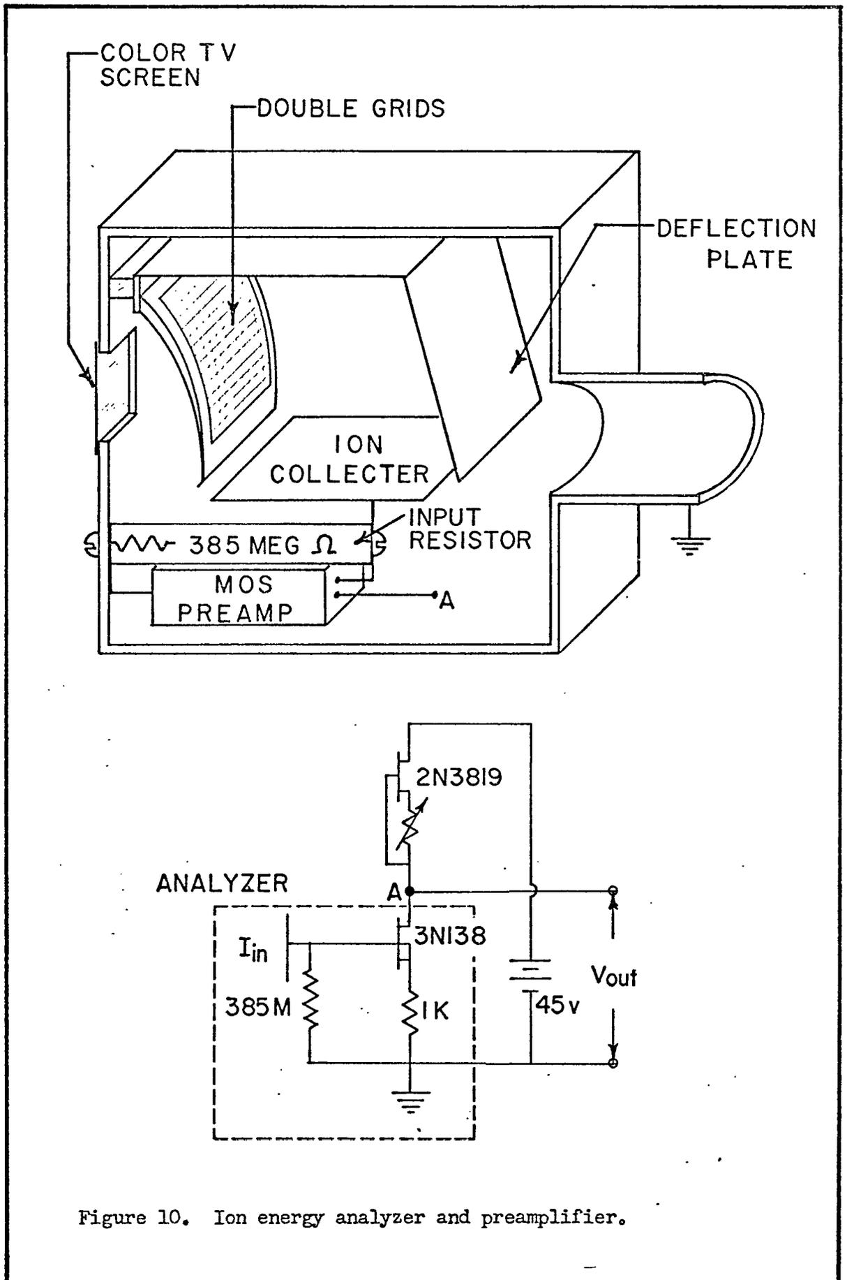
Figure 10. Ion energy analyzer and preamplifier.
