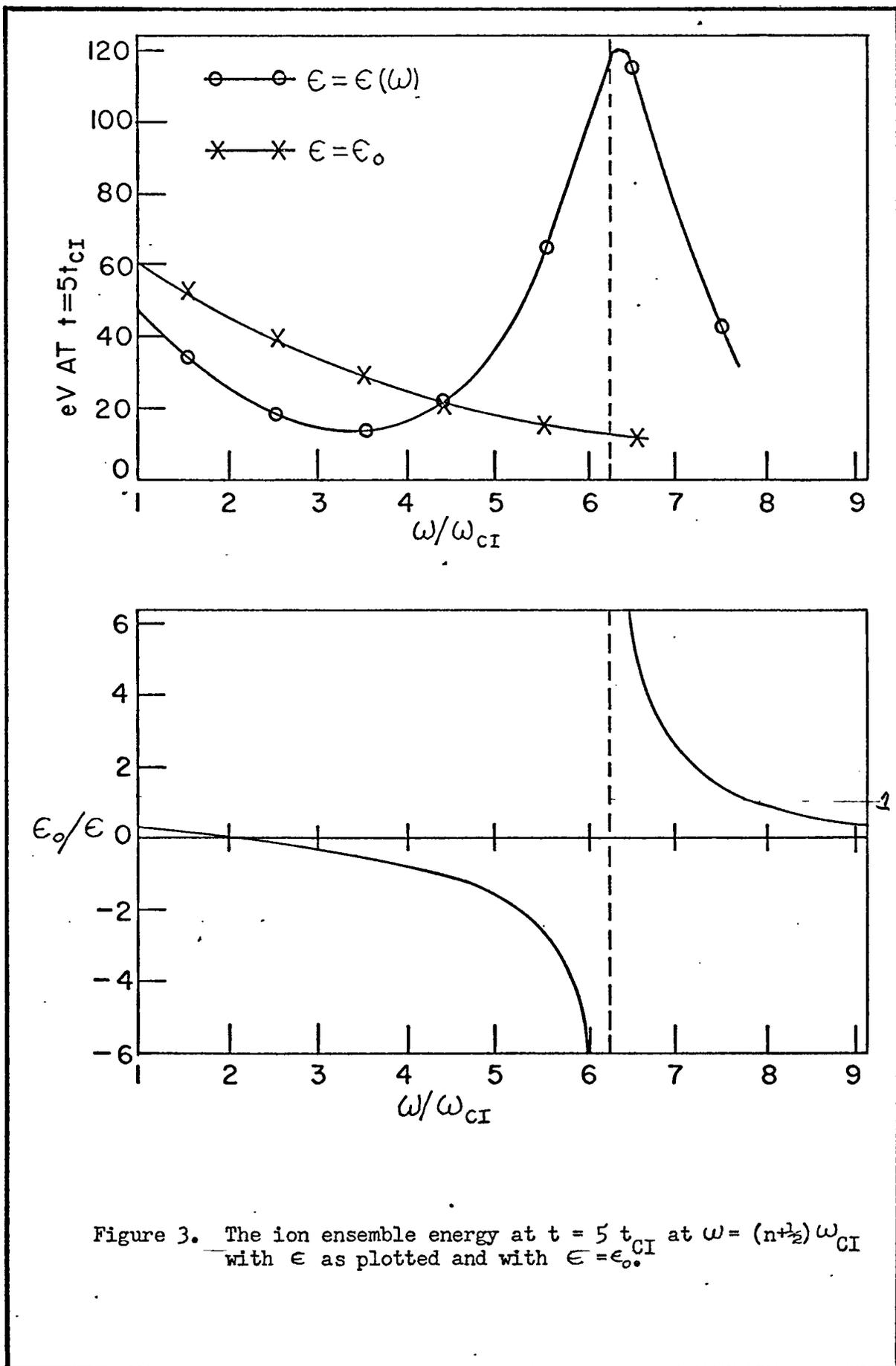
Figure 3. The ion ensemble energy at  $t = 5 t_{CI}$  at  $\omega = (n + \frac{1}{2}) \omega_{CI}$  with  $\epsilon$  as plotted and with  $\epsilon = \epsilon_0$ .
