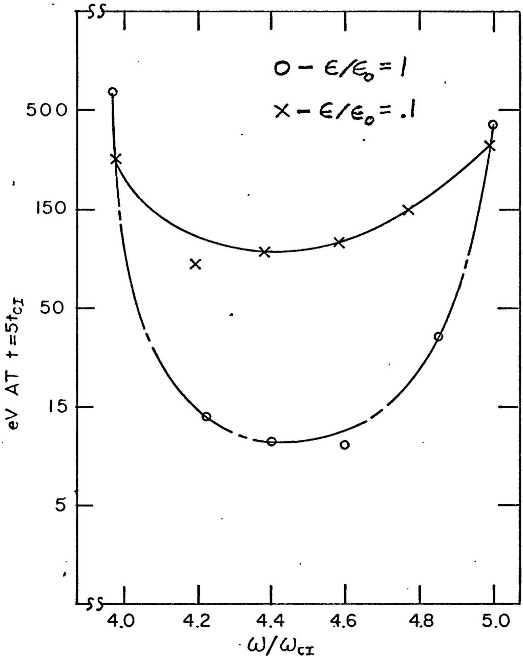
Figure 1. The ion ensemble energy at  $t=5t_{CI}$  for a 60 ma, 0.3 cm radius electron beam for modulation frequencies from  $4\omega_{CI}$  to  $5\omega_{CI}$  with two dielectric values.
