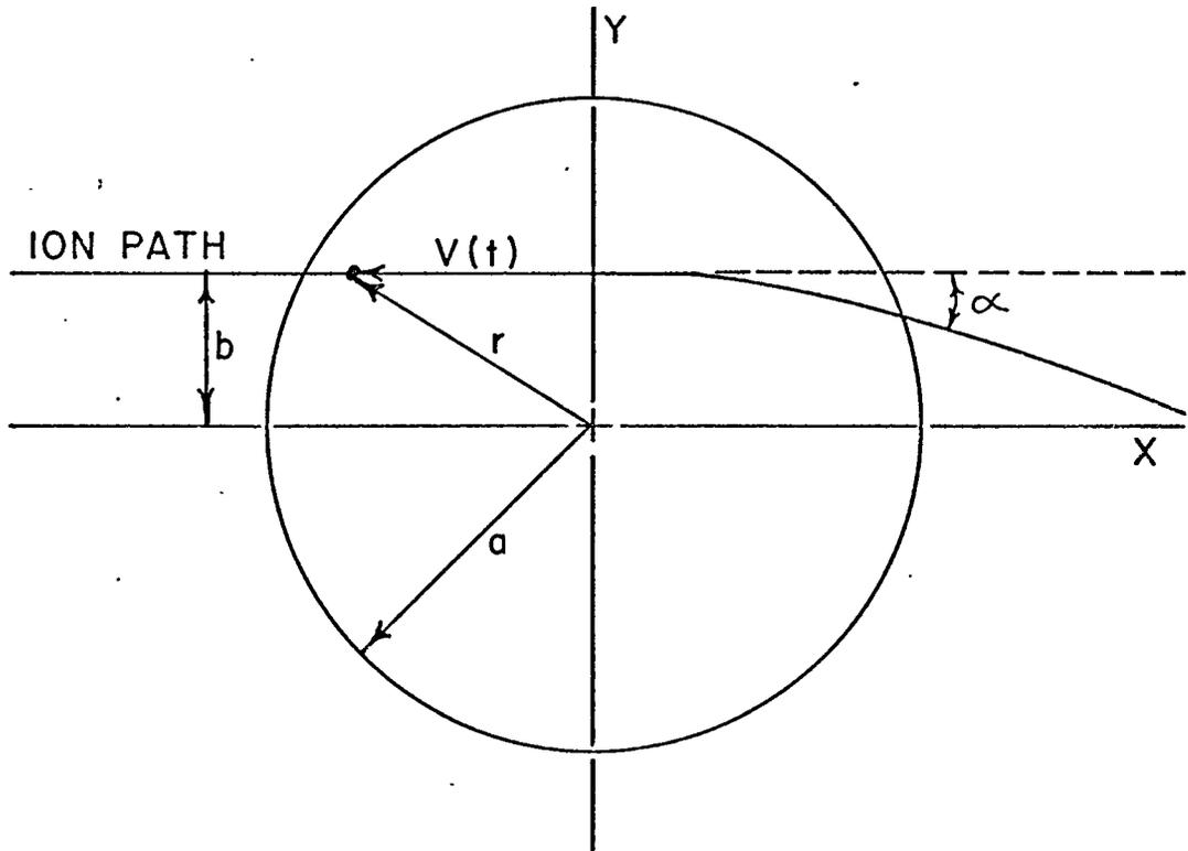
Figure 7. Coordinate frame used in calculation of ion deflection,  $\alpha$ .
