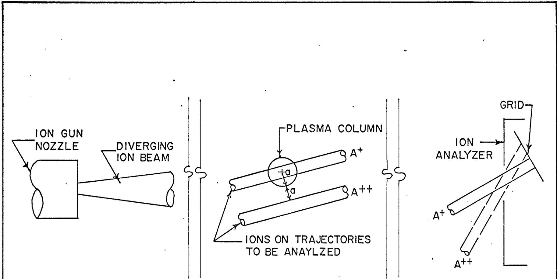
Figure 13. Geometry of ion gun, plasma column and ion analyzer. The deflection angles have been exaggerated.
