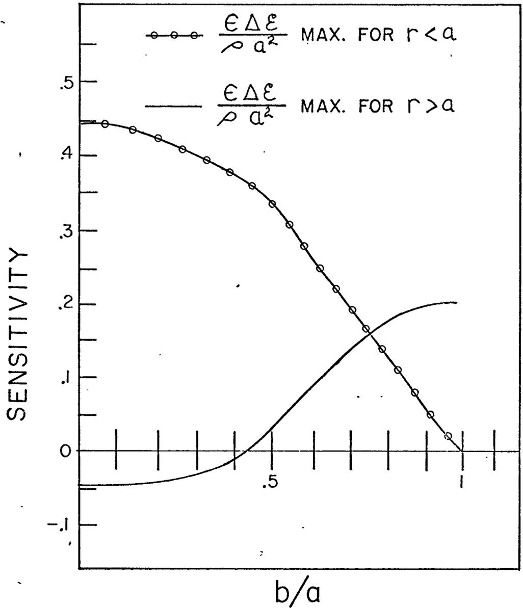
Figure 8. The sensitivity of the test ion energy to the electric fields in the regions  $r < a$  and  $r > a$  vs  $b$ , for  $x = 2$ .
