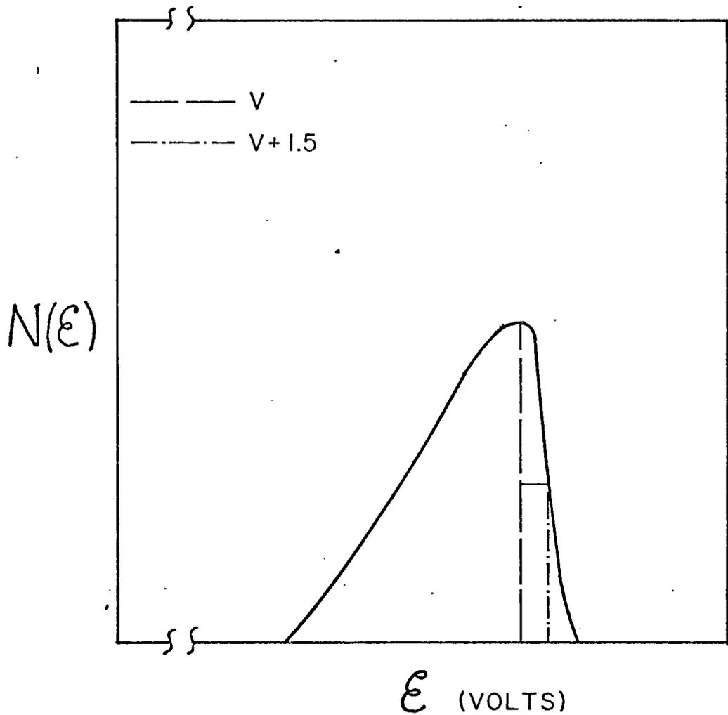
Figure 12. Typical test ion energy spectrum without plasma or electron beam.
