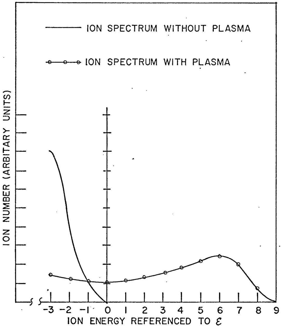
Figure 6. The test ion energy spectrum before and after passing through the plasma column.
