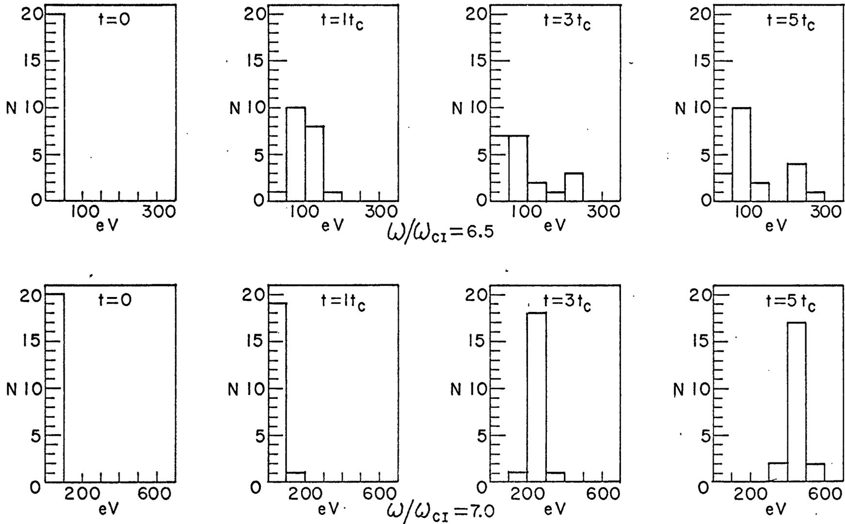
Figure 2. The time evolution of the ion energy distribution for  $\omega/\omega_{CI} = 6.5$  with  $\epsilon/\epsilon_0 = .14$  and for  $\omega/\omega_{CI} = 7$  with  $\epsilon/\epsilon_0 = .25$ .
