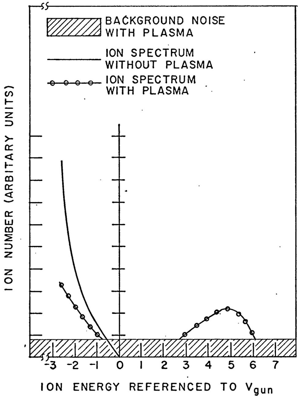
Figure 14. Test ion energy with 2.4 ma electron beam and  $f = 7$  MHz.
