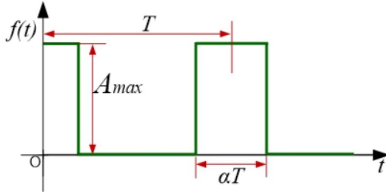
**Figure 5-8 Simplified input current of conventional topology.**
