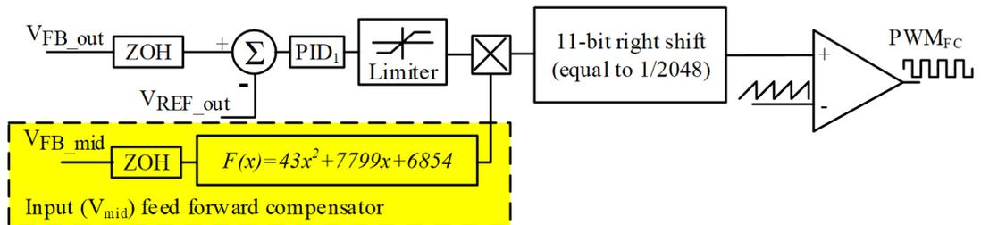
Figure 2-11 Fast converter control loop.
