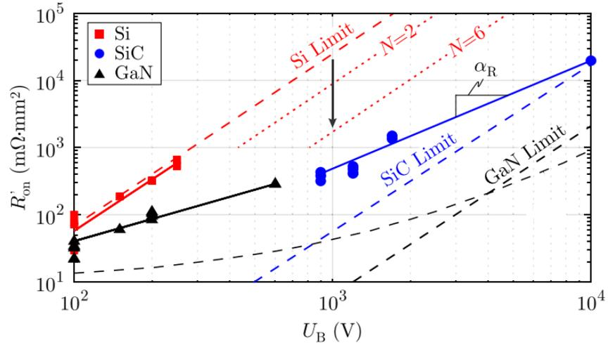
**Figure 1-9** Specific  $R_{dson}$  at 25 °C junction temperature ( $T_j$ ) for a selection of commercial power semiconductors. The Si, SiC and GaN theoretical limits from [29]–[31] are shown (dashed) together with the power function fits ( $k_R \cdot U_B^{\alpha_R}$ ) given in Table 1.1.
