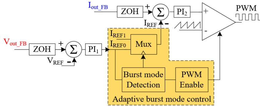
Figure 3-8 Adaptive burst mode control loop.
