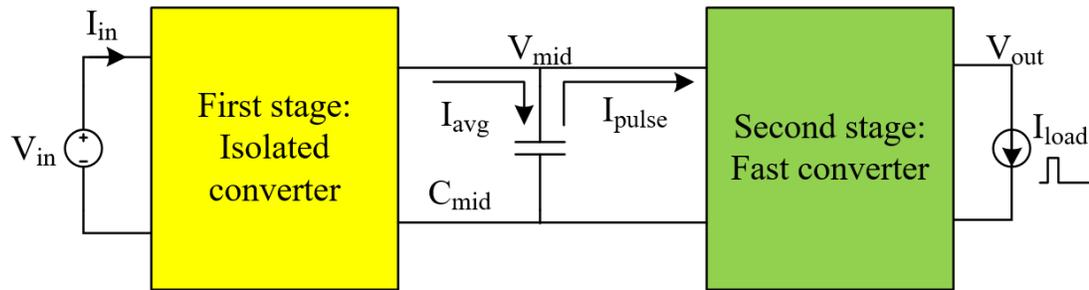
**Figure 2-2 Block diagram of proposed converter.**
