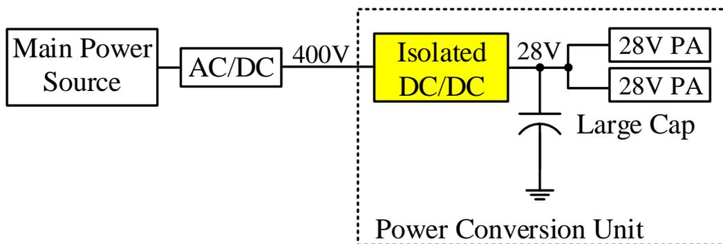
**Figure 6-1 Power supply structure in a typical pulsed application with PAs.**
