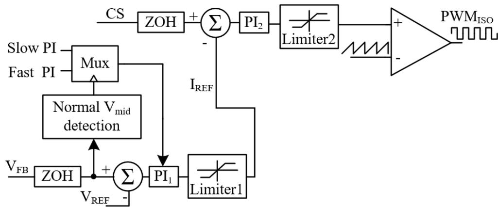
Figure 2-7 Average current control loop in isolated converter.
