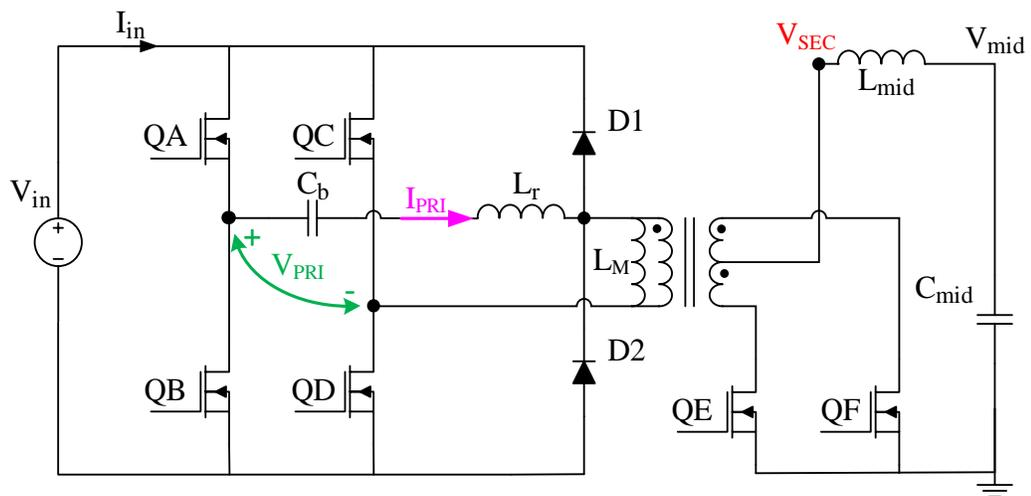
Figure 2-5 Proposed isolated converter schematic.
