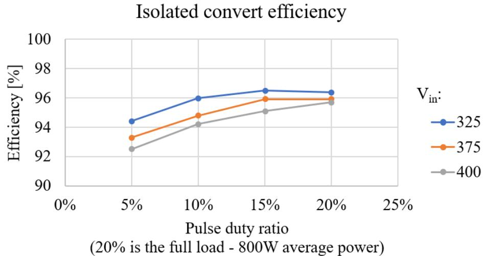
**Figure 2-16 Isolated converter efficiency with different input voltage.**
