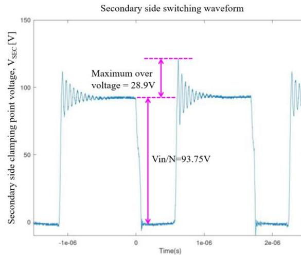
**Figure 3-13 Secondary side clamping point,  $V_{SEC}$  waveform.**
