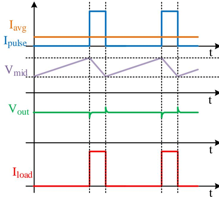
**Figure 2-4 Ideal main operating waveforms of proposed converter.**
