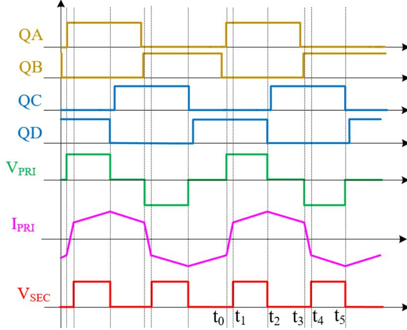
Figure 2-6 Isolated converter main operating waveforms.
