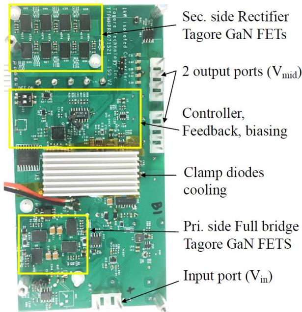
(b) isolated converter bottom view
