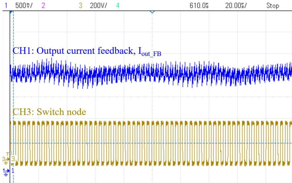
(c) Continuous mode operation with 8 A load current
