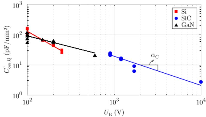
**Figure 1-10 Specific charge-equivalent output capacitance  $C_{oss}$  for a selection of commercially-available power devices. The power function fits ( $k_C \cdot U_B^{\alpha_C}$ ) are given in Table 2.**
