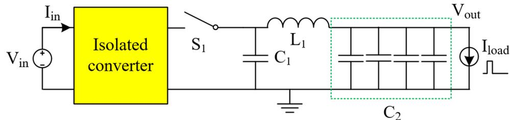
Figure 2-1 Block diagram of the conventional converter.
