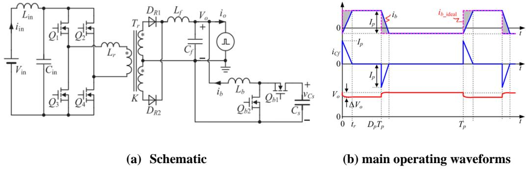
**Figure 1-7 Schematic and main operating waveforms of active capacitor converter.**
