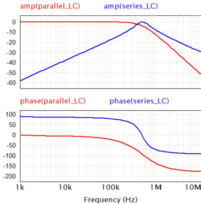
**Figure 5-5 Different resonant tanks amplitude and phase response.**
