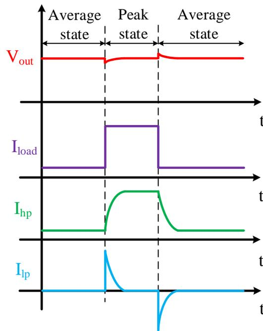
Figure 6-3 Idealized operating waveform.
