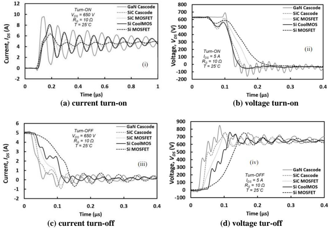
Figure 1-11 The transients of the silicon, SiC & GaN devices. It can be seen that the GaN device is the fastest in all switching.
