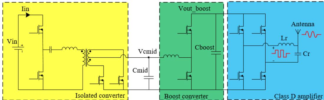
Figure 5-2 Simplified schematic of the proposed power converter for pulsed power in NMR application and operating waveforms.
