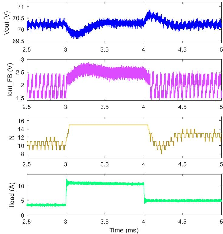
**Figure 3-15** Prototype converter load transients (3.5 A to 11 A to 5 A) operating waveforms with adaptive burst mode control. ( $N$  waveform is the real time value calculated in the microcontroller,  $N = 15$  means prototype operates in continuous mode)
