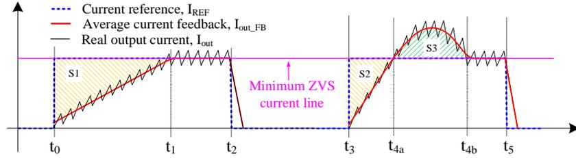
(b) Fast current loop PI calculation (fast output current increasing but inherent current overshoot S3)
