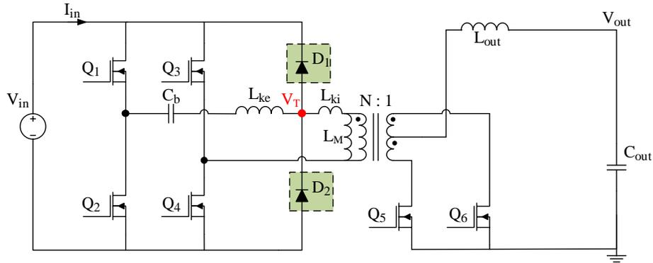
(a) PSFB converter with diode clamping
