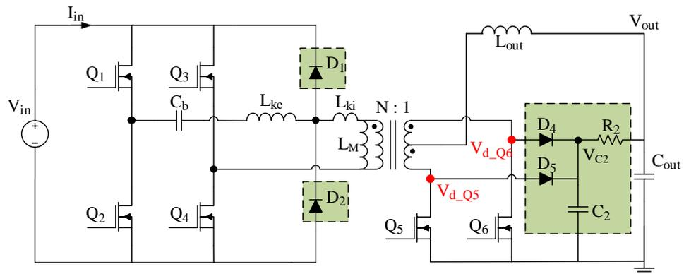
(c) PSFB converter with diode clamping + dual RCD clamping
