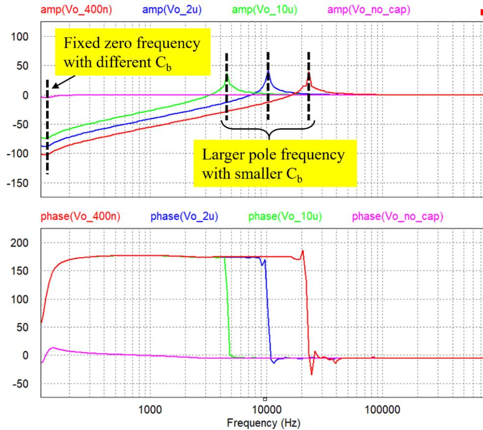
Figure 3-4 AC sweep results with different  $C_b$  (red-  $C_b=400\text{nF}$ , Blue- $C_b=2\ \mu\text{F}$ , Green- $C_b=10\ \mu\text{F}$  and Pink- $C_b=0\ \mu\text{F}$ ).
