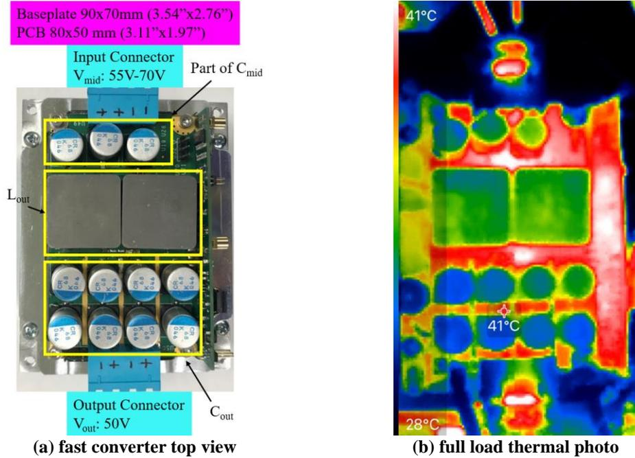
**Figure 2-17 Hardware of second stage fast converter.**
