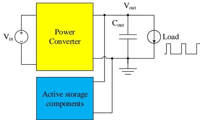
**Figure 1-6 Block diagram of active-controlled storage components PPSs.**
