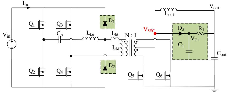
(b) PSFB converter with diode clamping + RCD clamping
