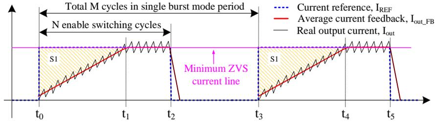
(a) Conventional current loop PI calculation (slow output current increasing)
