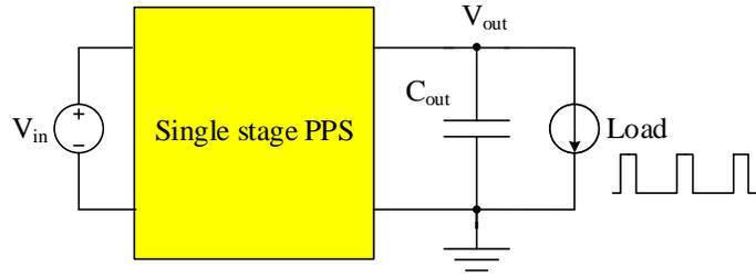
**Figure 1-3 Block diagram of single stage PPSs.**
