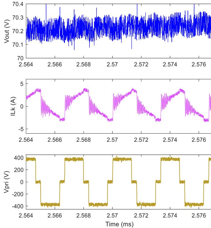
**(b) Zoomed in waveforms of primary side operating. ( $I_{Lk}$  is the leakage inductor current and  $V_{pri}$  is the voltage difference between the switching nodes of two legs)**
