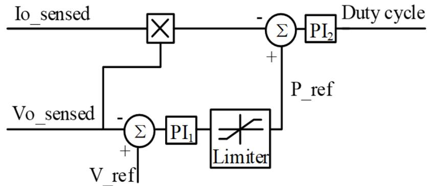
Figure 5-6 Isolated converter close loop controller.
