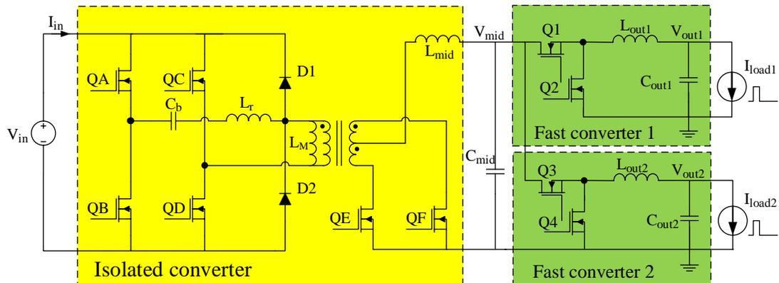
Figure 2-3 Schematic of proposed converter.
