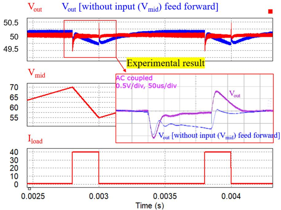
Figure 2-19 Simulation and experimental waveforms of line regulation comparison with/without input (Vmid) feed forward.
