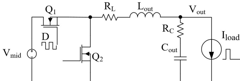
Figure 2-10 Second stage fast converter schematic.
