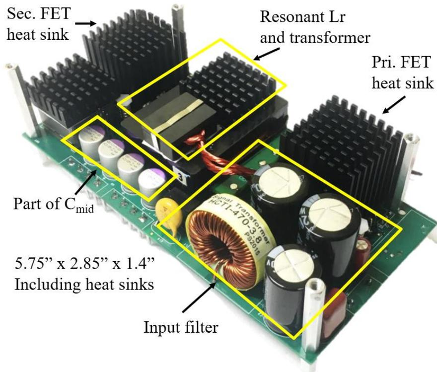
(a) isolated converter top view
