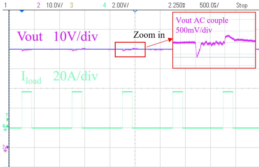
Figure 2-18 Fast converter experimental waveforms of transient response with pulsed load.
