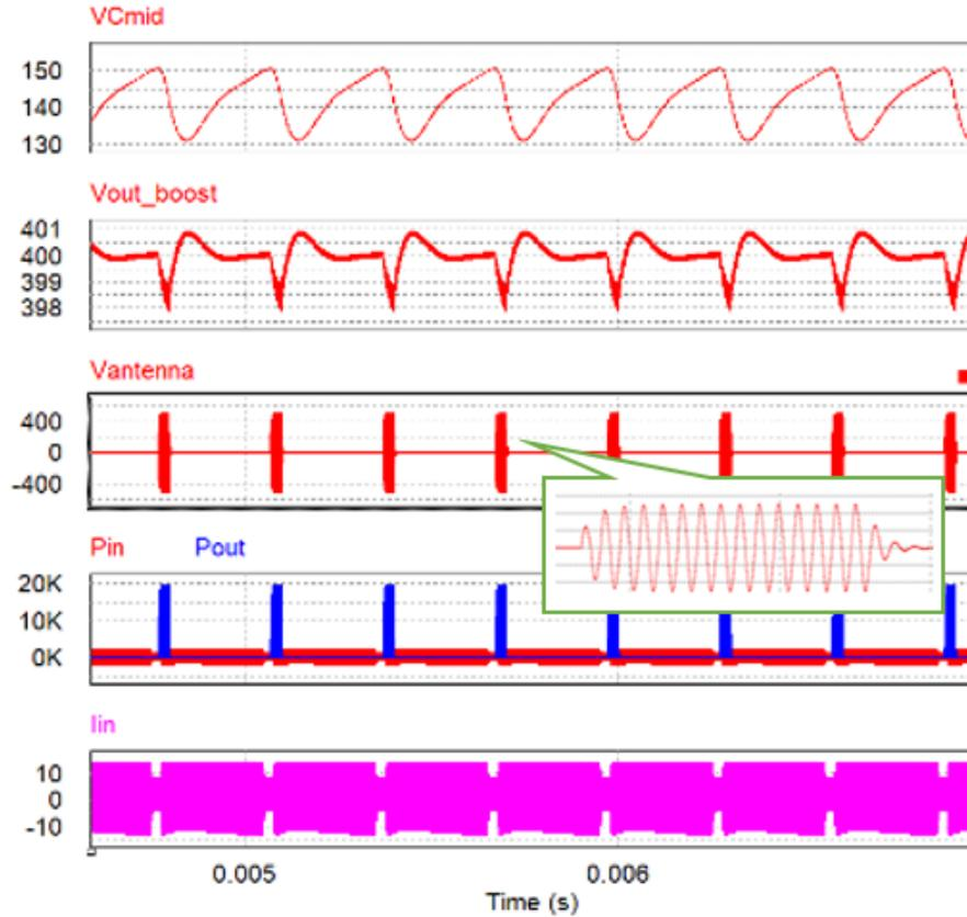
**Figure 5-9** PSIM simulation results--(a) Mid-point capacitor voltage [V], (b) Output voltage of boost converter [V], (c) Antenna output voltage [V], (d) Proposed converter input power and output power [W], (e) Input current after input capacitor [A].
