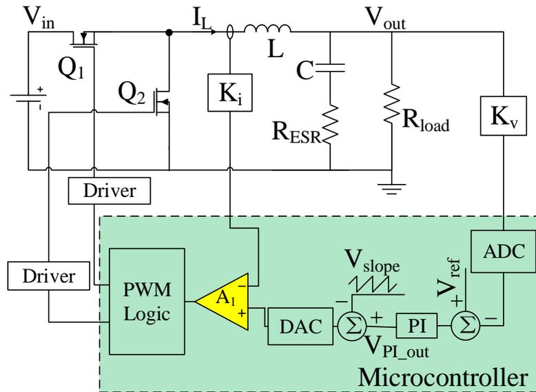
Figure 4-1 Digital peak current control buck converter.
