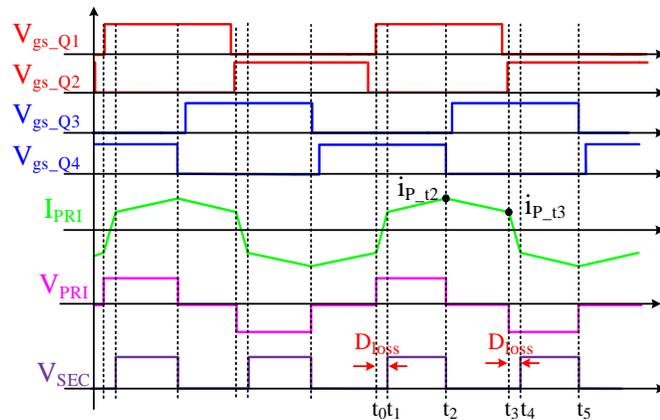
**Figure 3-2 PSFB converter’s main operational waveforms.**
