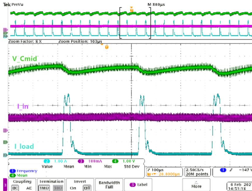
Figure 5-10 Scaled down pulsed load test results—(Ch. 2) Pulsed mode load current [A], (Ch. 3) Input current before input capacitor, (Ch. 4) Mid-point capacitor voltage [V].
