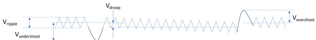
**Figure 1-1 Ideal PPS output voltage waveform.**
