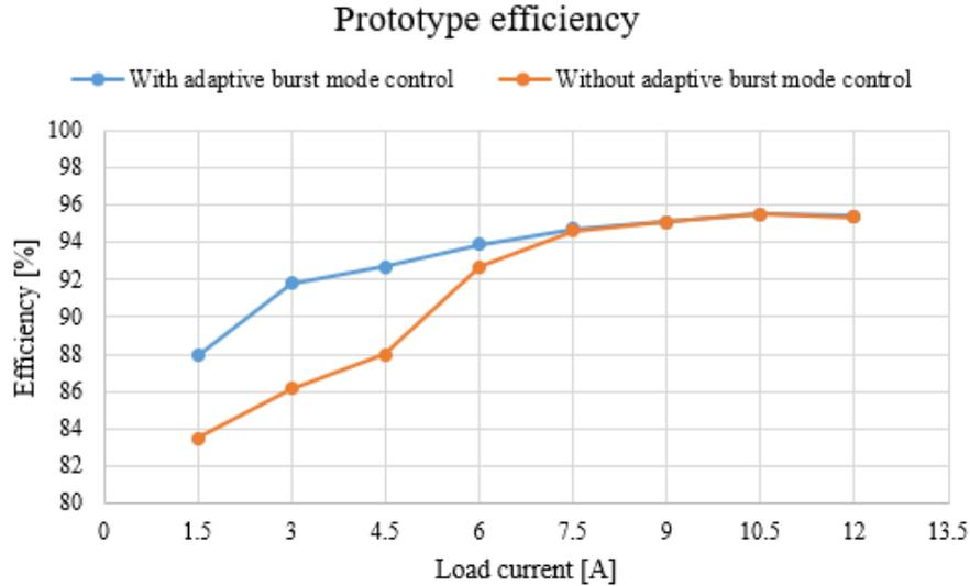
**Figure 3-17 Prototype efficiency with and without adaptive burst mode control. (DC biasing power loss is 9 W at no load condition)**
