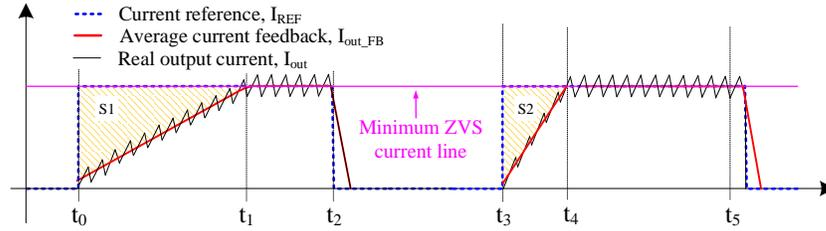
(c) Adaptive current loop PI calculation (fast output current increasing and no inherent current overshoot)
