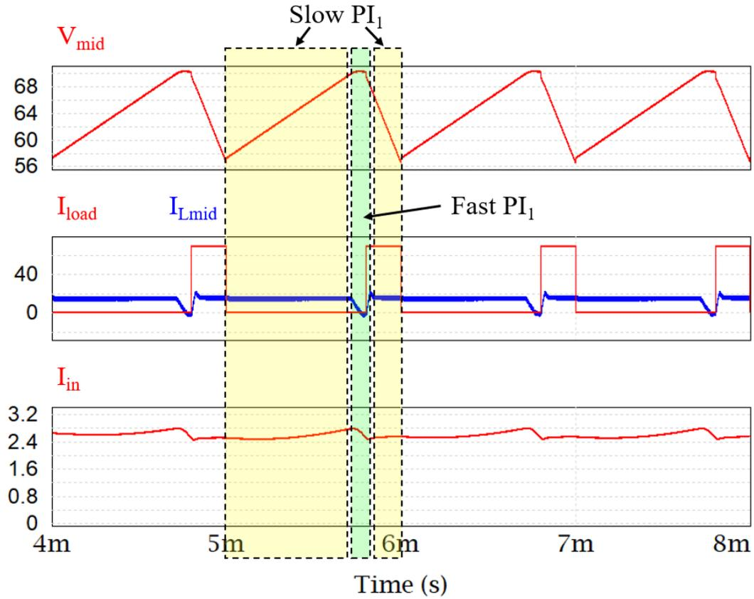
**Figure 2-8 Simulation waveforms of fast/slow PI<sub>1</sub> switching.**
