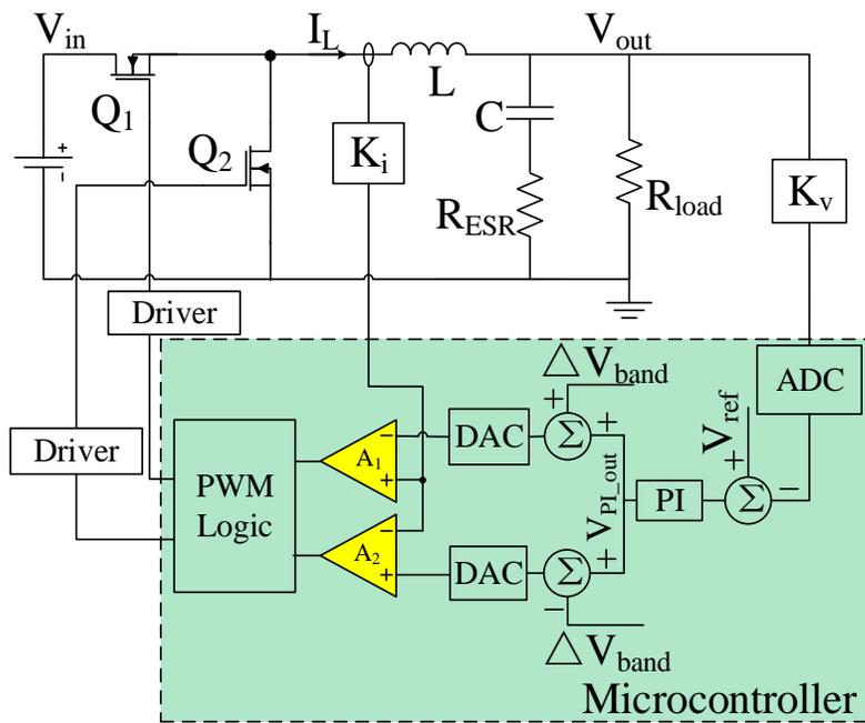
Figure 4-4 Digital hysteresis current control buck converter.
