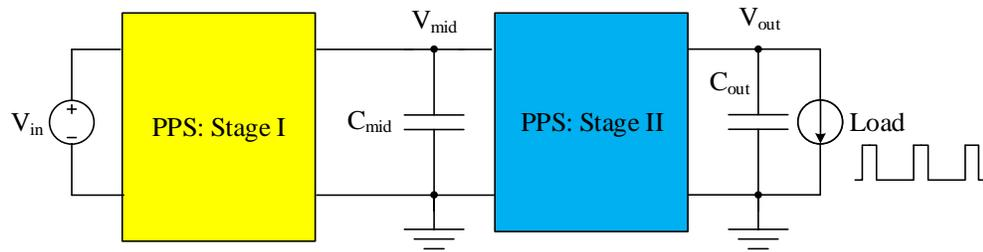
Figure 1-4 Block diagram of series connected two stage PPSs.
