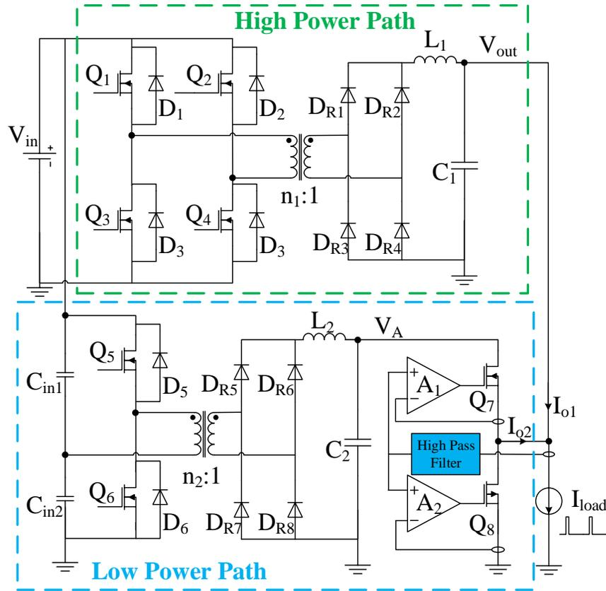
Figure 6-4 Schematic of proposed topology.
