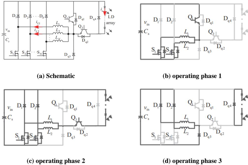
**Figure 1-8 Schematic and main operating phases of active inductor converter.**
