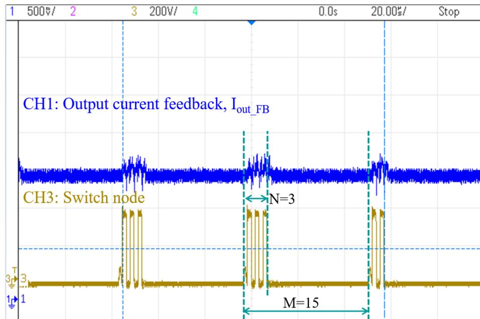
(a) Burst mode operation with 300 mA load current (single burst mode period consists of M switching cycles and N cycles are enabled)
