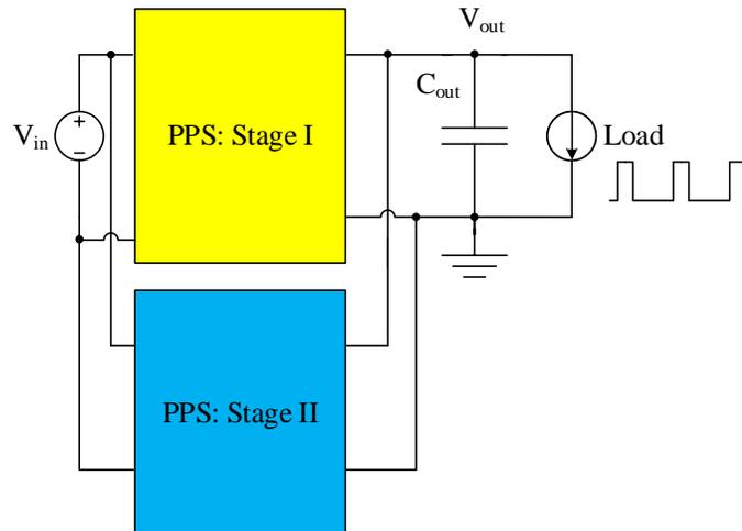
**Figure 1-5 Block diagram of parallel connected two stage PPSs.**
