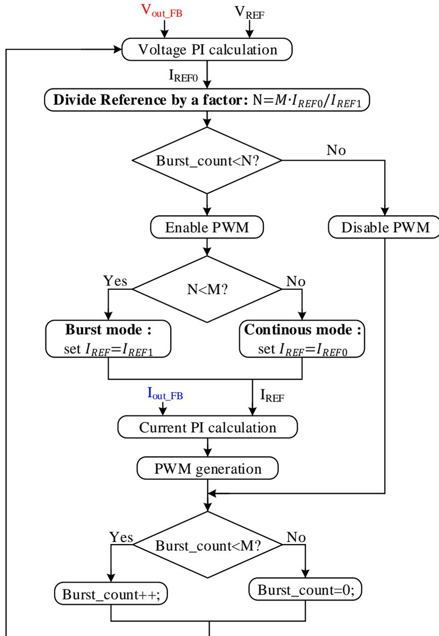
Figure 3-9 Controller flowchart of adaptive burst mode control loop.
