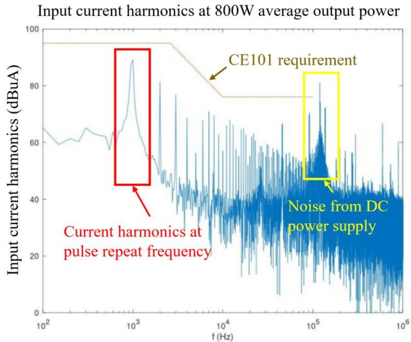
Figure 2-15 Input current FFT under full load condition.
