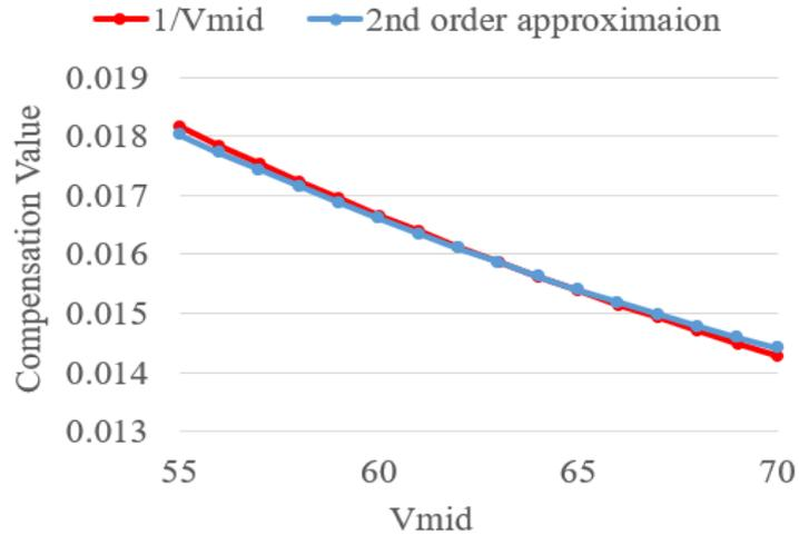
**Figure 2-12 1/V<sub>mid</sub> and 2nd order approximation comparison.**
