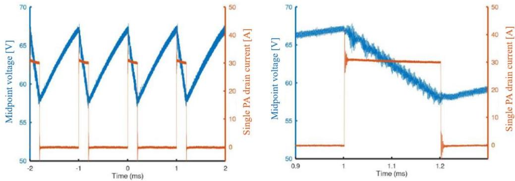
(a) isolated converter output voltage with single pulsed load
