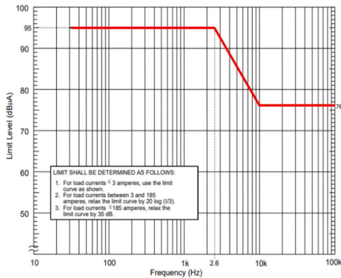
**Figure 1-2 Conducted emissions test standard (CE101) for low frequency (LF) noise.**
