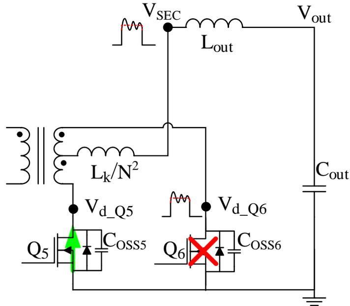
Figure 3-5 The ringing equivalent circuit referred to the secondary side.
