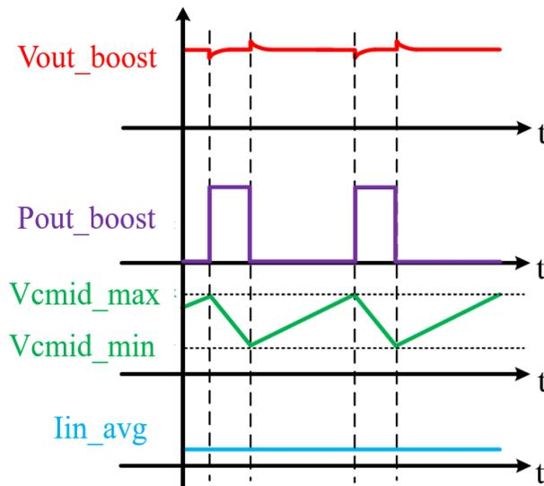
**Figure 5-3 Proposed power converter operating waveforms.**
