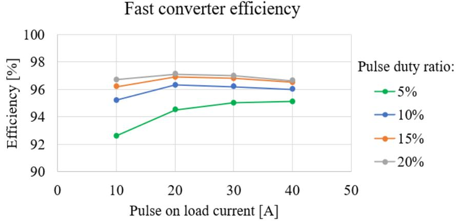
**Figure 2-20 Fast converter efficiency with different pulse on current and different pulse duty ratio.**
