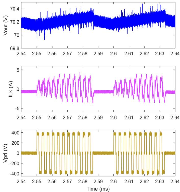
(a) Primary side operating waveforms for continuous two burst mode periods. ( $I_{Lk}$  is the leakage inductor current and  $V_{pri}$  is the voltage difference between the switching nodes of two legs)
