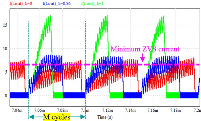
**Figure 3-11 Results comparison of different current loop PI calculations. (k=0: conventional PI calculation; k=1: fast PI calculation; k=0.86: adaptive current loop PI calculation)**
