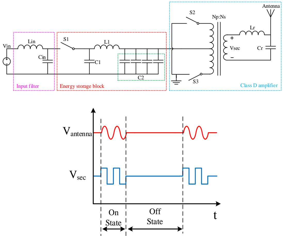
**Figure 5-1 Typical power converter for antenna in NMR application and operating waveforms.**
