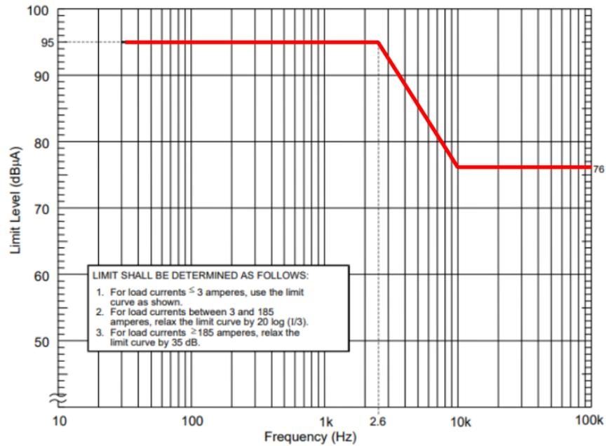
**Figure 5-7 Harmonics requirement for conducted emissions test.**
