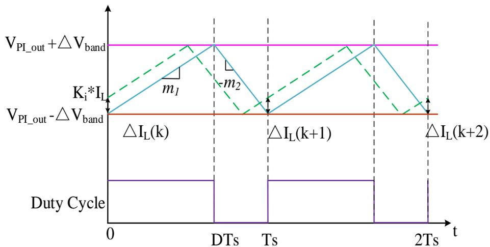
Figure 4-5 Operating waveforms of DHC control.
