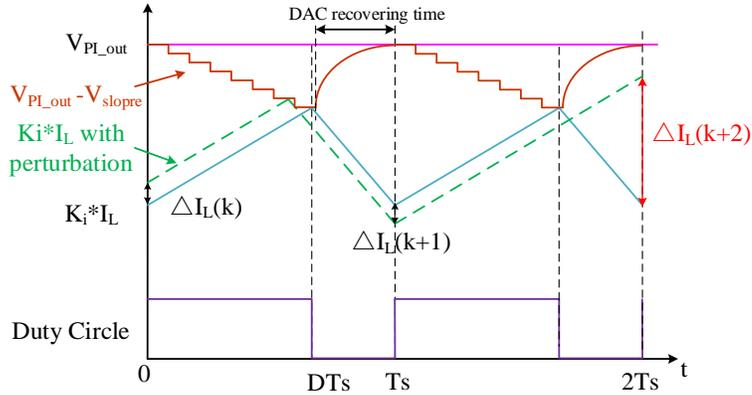
**Figure 4-3 Practical operating waveforms of DPC control.**
