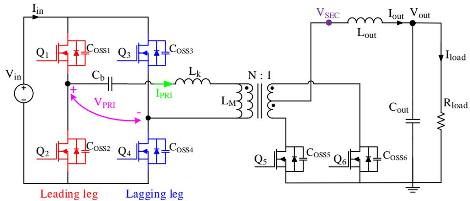
**Figure 3-1 Phase shifted full bridge (PSFB) converter schematic.**
