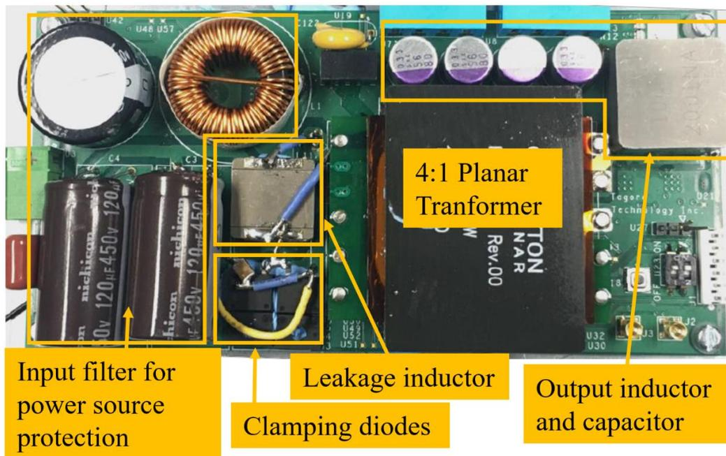
(a) Experimental prototype top view
