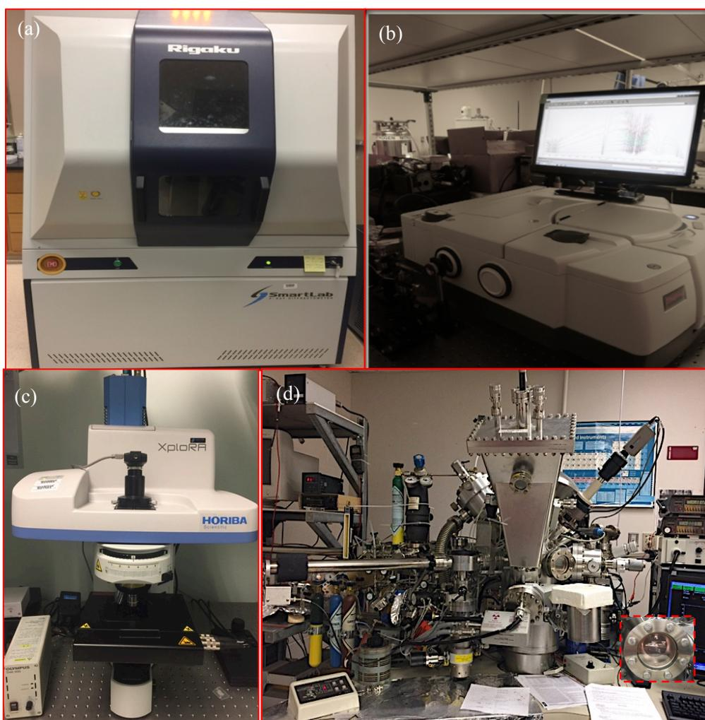
Figure 31 The characterization instruments (a) XRD (b) FTIR (c) Raman (d) XPS
