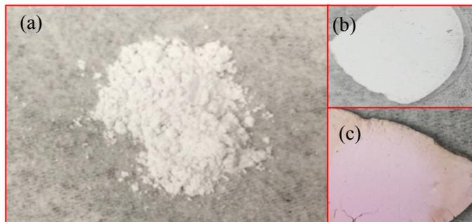
Figure 33 (a) Synthesized pseudoboehmite (b) sapphire pellet (c) ruby pellet
