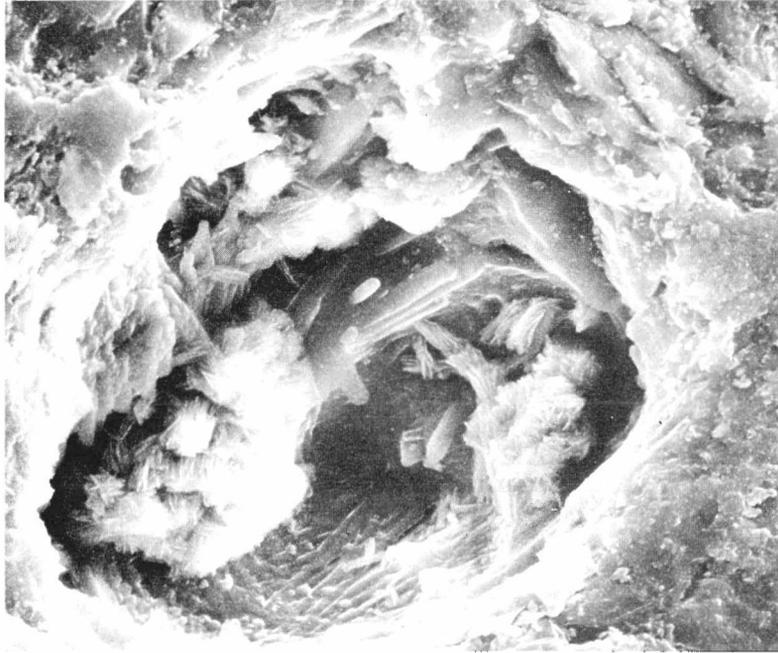
FIGURE 39: Iron weathering products in partially glass-lined, partially-devitrified vesicle. Field of view 62  $\mu\text{m}$ .
