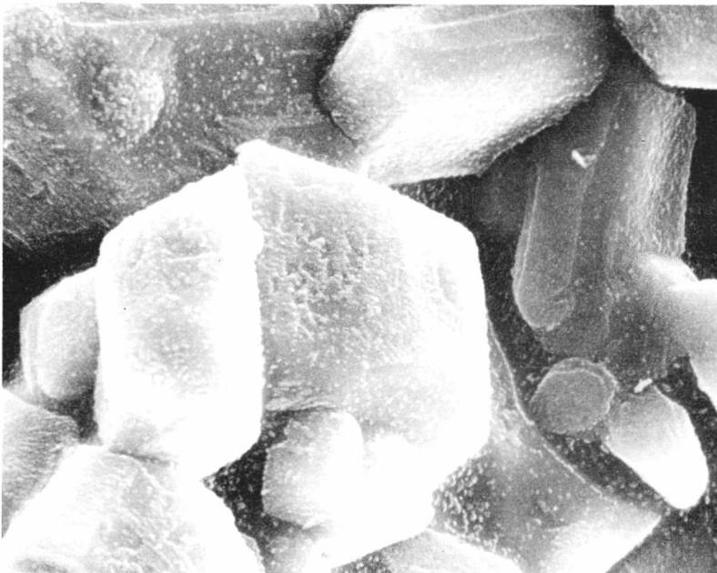
FIGURE 32B: Equant crystal, center of photograph. High Mg, Fe silicate (EDX analysis). Probably olivine because of high Fe+Mg/Si ratio. Field of view, 15  $\mu\text{m}$ .
