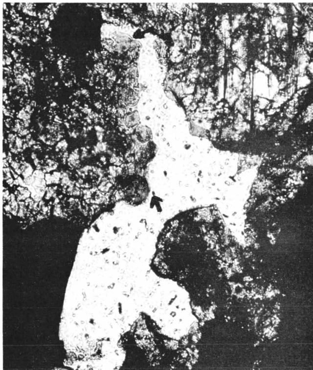
FIGURE 9: Olivine crystals (2-3  $\mu\text{m}$  in diameter) lining irregular vug 40  $\mu\text{m}$  in length. Note doubly-terminated crystal at top of vug, next to round (black) opaque.
