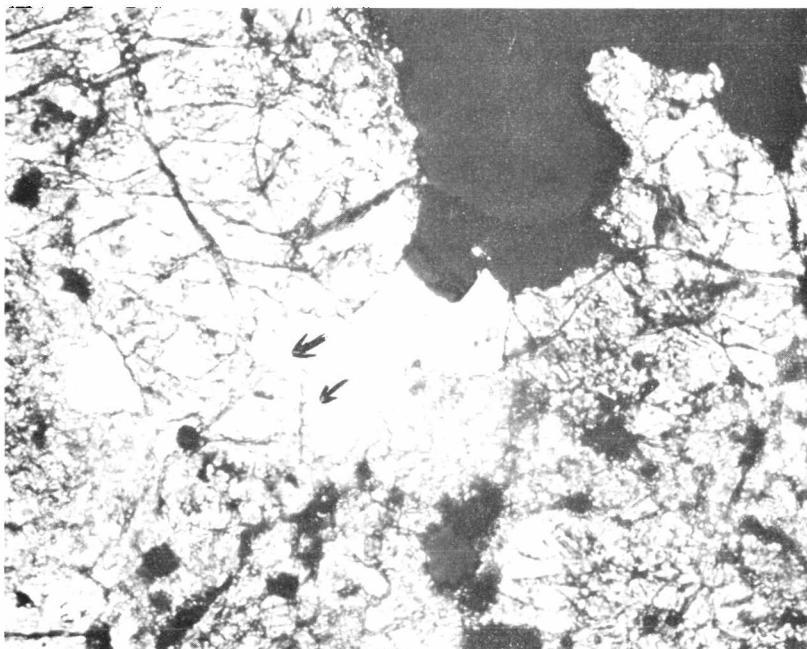
FIGURE 7: Width of vug is  $13.5\ \mu\text{m}$ . Note micron-sized crystals on vug wall which is a coarse-grained matrix silicate. Transmitted light.
