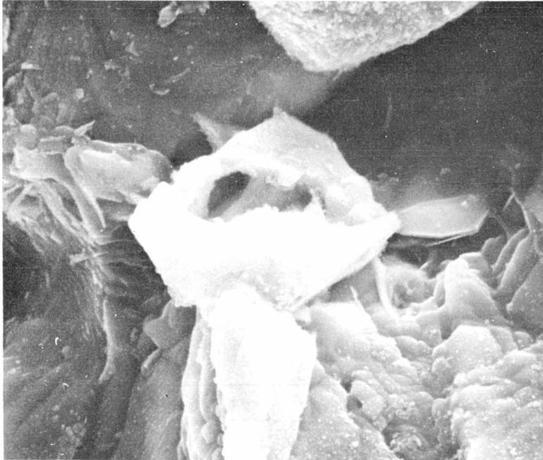
FIGURE 36C: The grain in the center is composed of Fe and Cr (EDX) and is 16  $\mu\text{m}$  in diameter.
