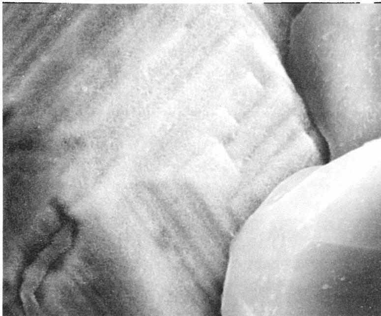
FIGURE 41B: High magnification of cubic iron crystal. Growth steps are evident. "Fuzzy" texture of surface attributed to etching, alteration of iron by weathering. Field of view 15  $\mu\text{m}$ .
