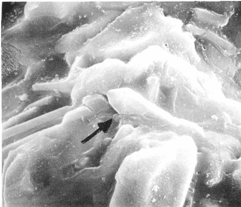
FIGURE 36H: Needle-like crystal is a Ca- P- Si-bearing mineral, measures 3 x 8  $\mu\text{m}$ .
