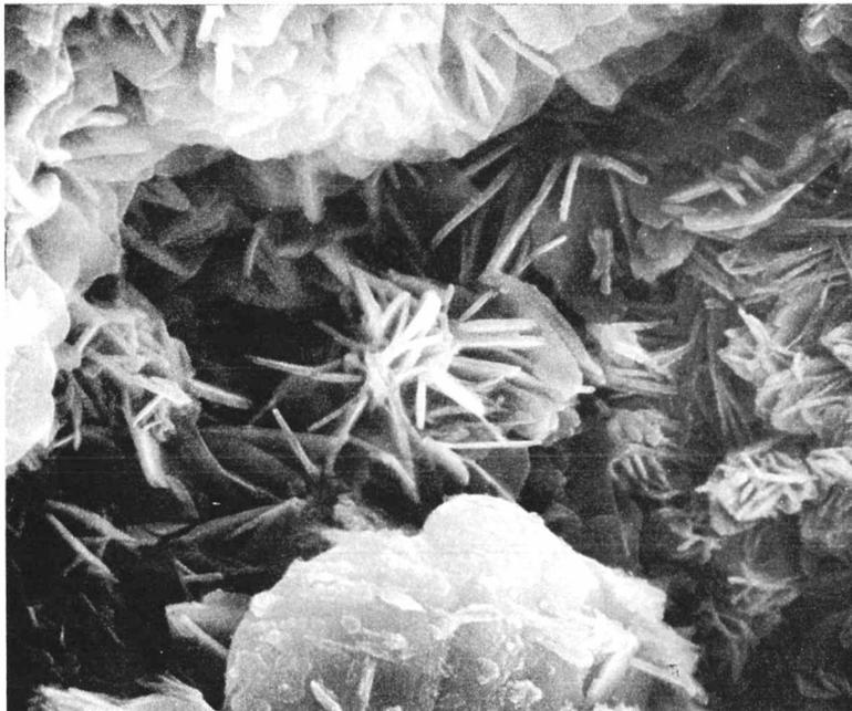
FIGURE 40A: Bladed iron alteration product in Rose City meteorite. Field of view, 25  $\mu\text{m}$ .
