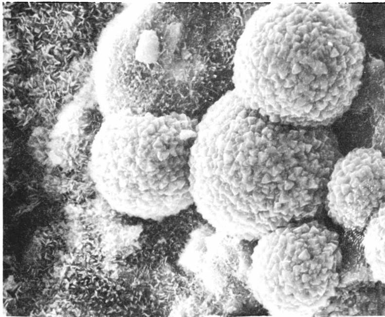
FIGURE 37B: Note floor of cavity is covered with bladed forms of oxidized iron. Largest sphere is 20  $\mu\text{m}$ .
