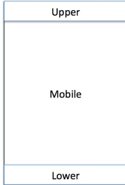
**Figure 4.2:** Different regions defined in the GB specimens. The lower region was held fixed and shear was applied on the upper region.
