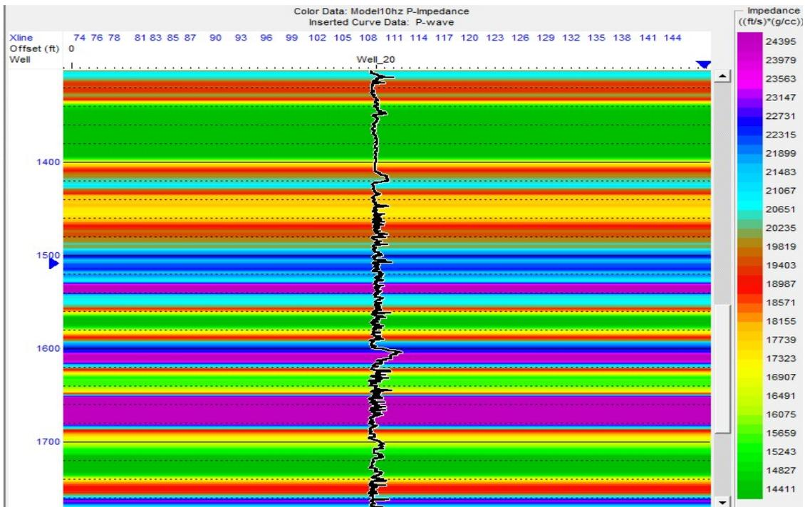
Figure 5-6: Pre-stack inversion model, 10Hz.
