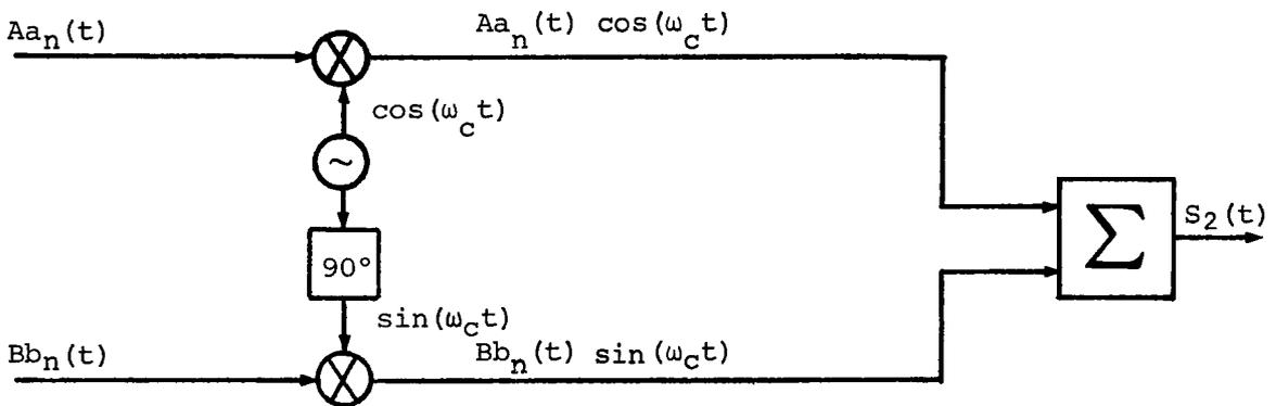
(b) Addition of DSB-modulated quadrature carriers  $[a_n(t) = \pm 1, b_n(t) = \pm 1]$
