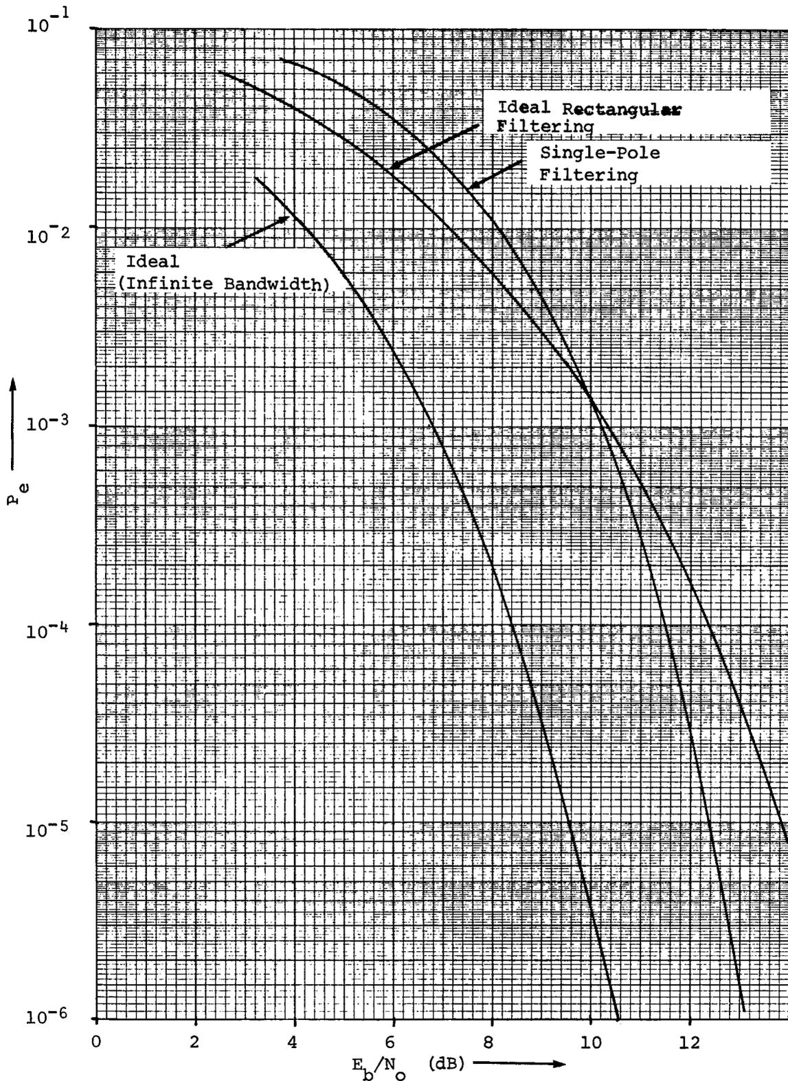
Fig. 4.17. - Comparison of Error probability results for single-channel QPSK transmission ( $f_c T_A = 10$ ,  $T_A/T_B = 1$ ,  $B_{IF} T_A = 1$ )
