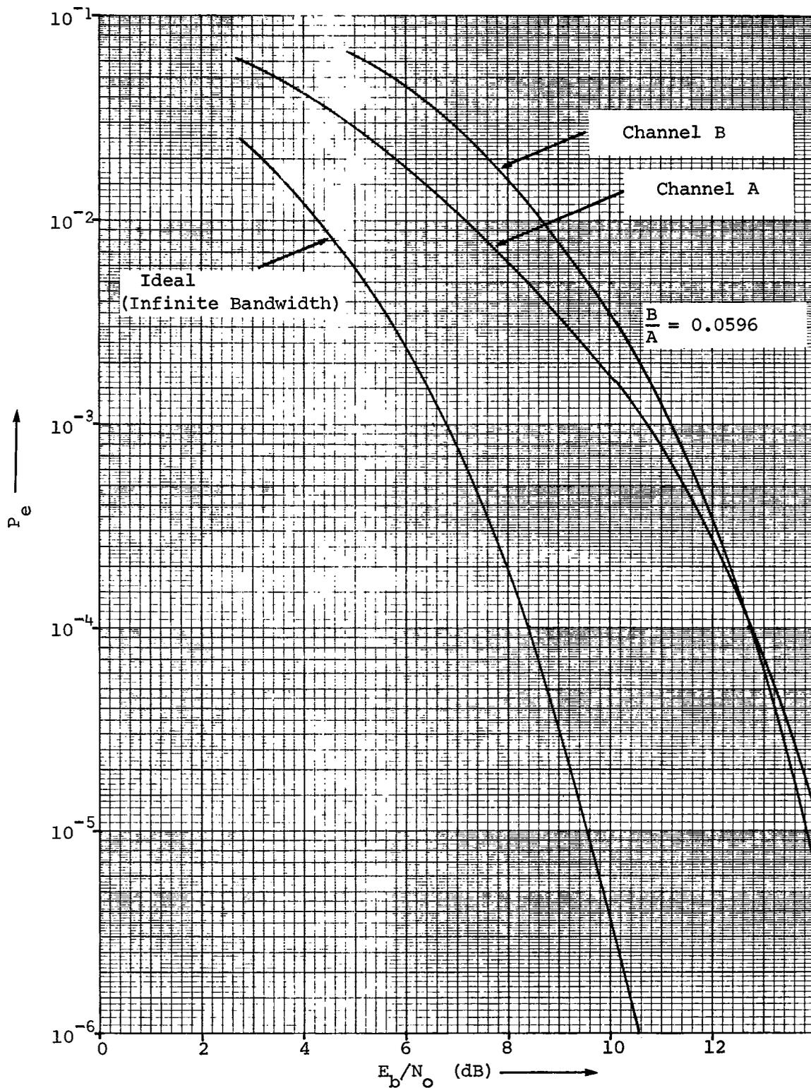
Fig. 4.13. - Iterated error probability results for dual-channel QPSK transmission with ideal rectangular filtering ( $f_c T_A = 1$ ,  $T_A/T_B = 0.01$ ,  $B_{IF} T_A = 1$ )
