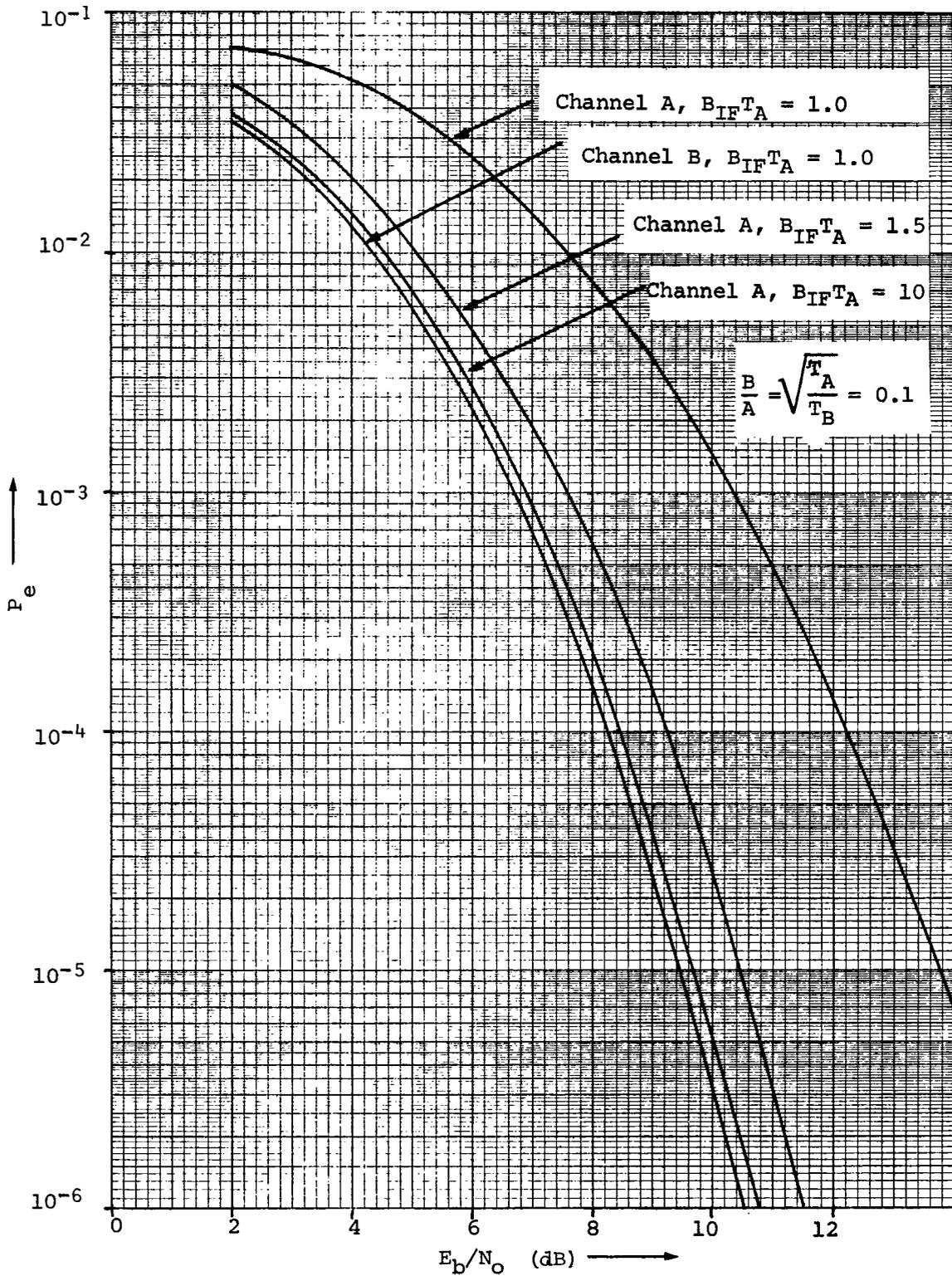
Fig. 4.7. - Error probability results for dual-channel QPSK transmission with ideal rectangular filtering
