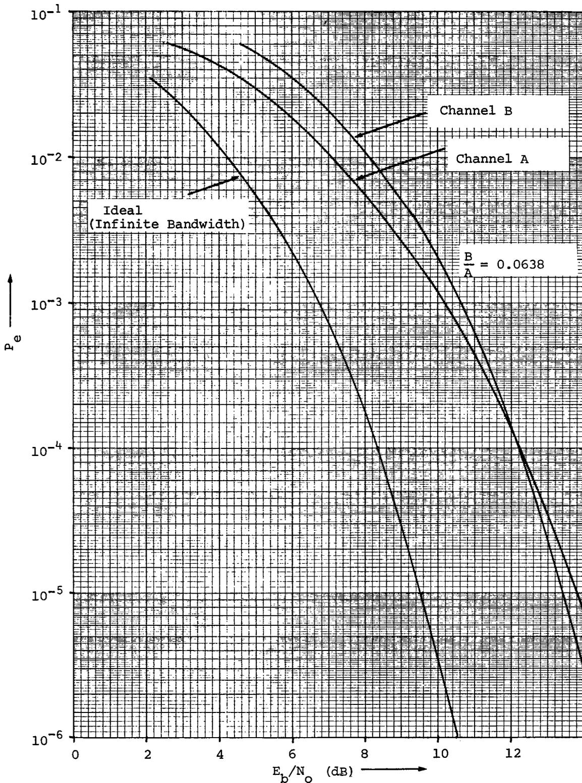
Fig. 4.11. - Iterated error probability results for dual-channel QPSK transmission with ideal rectangular filtering ( $f_c T_A = 10$ ,  $T_A/T_B = 0.01$ ,  $B_{IF} T_A = 1$ )
