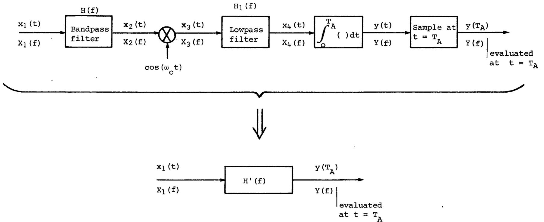
Fig. C.1. - Combination of bandpass filter with Channel A detector components
