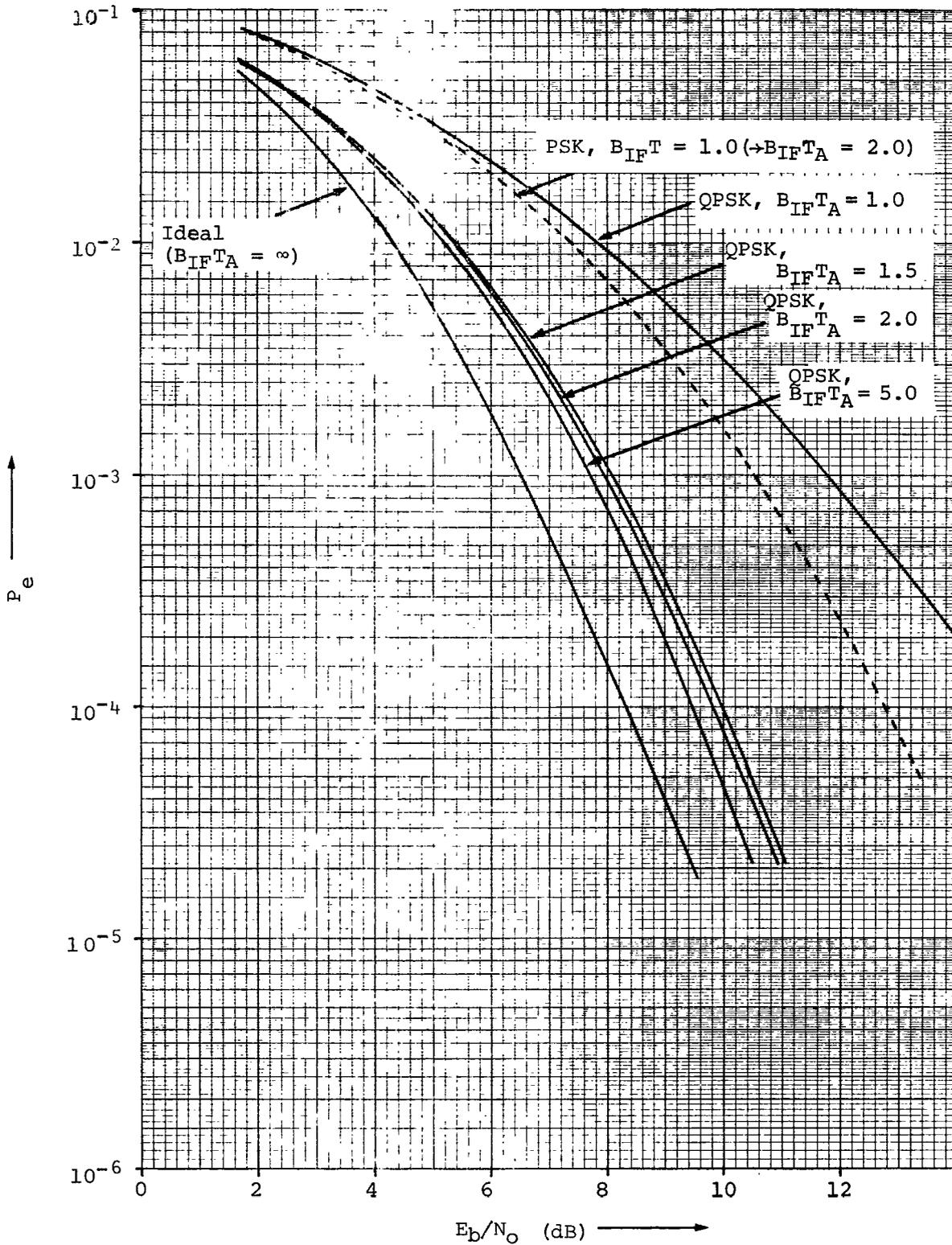
Fig. 4.6. - Error probability results for single-channel QPSK transmission with ideal rectangular filtering ( $f_c T_A = 1$ )
