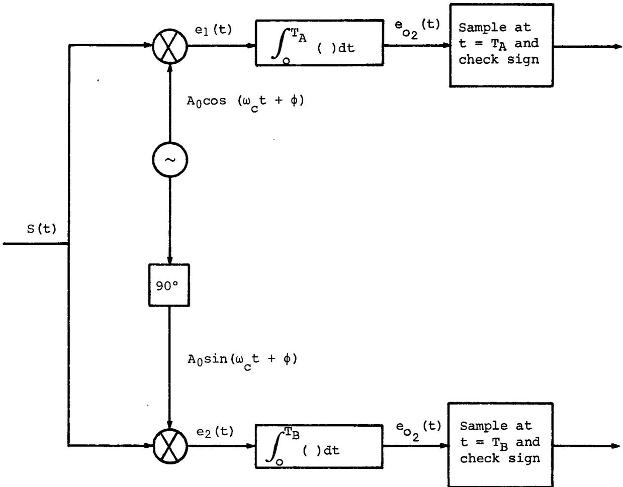
Fig. 3.2. - Detection of a QPSK signal
