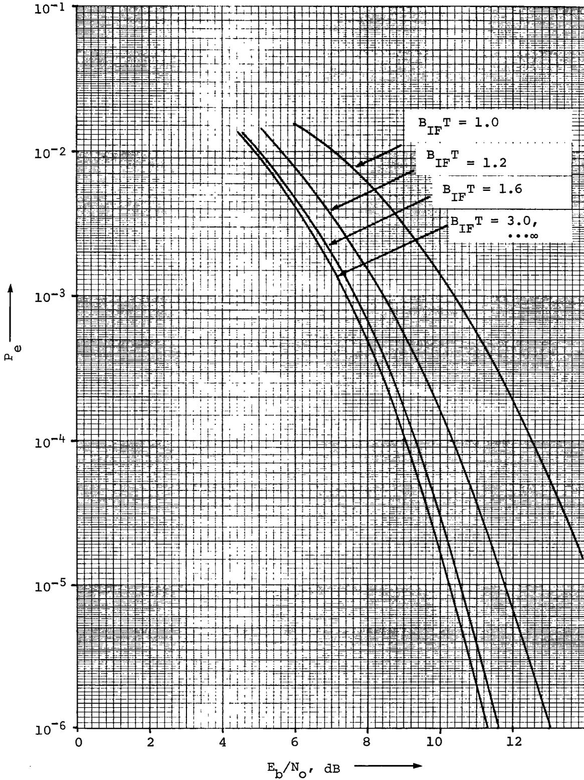
Fig. 2.5. -  $P_e$  vs.  $E_b/N_0$  for ideal bandlimited PSK with  $f_cT = 2$
