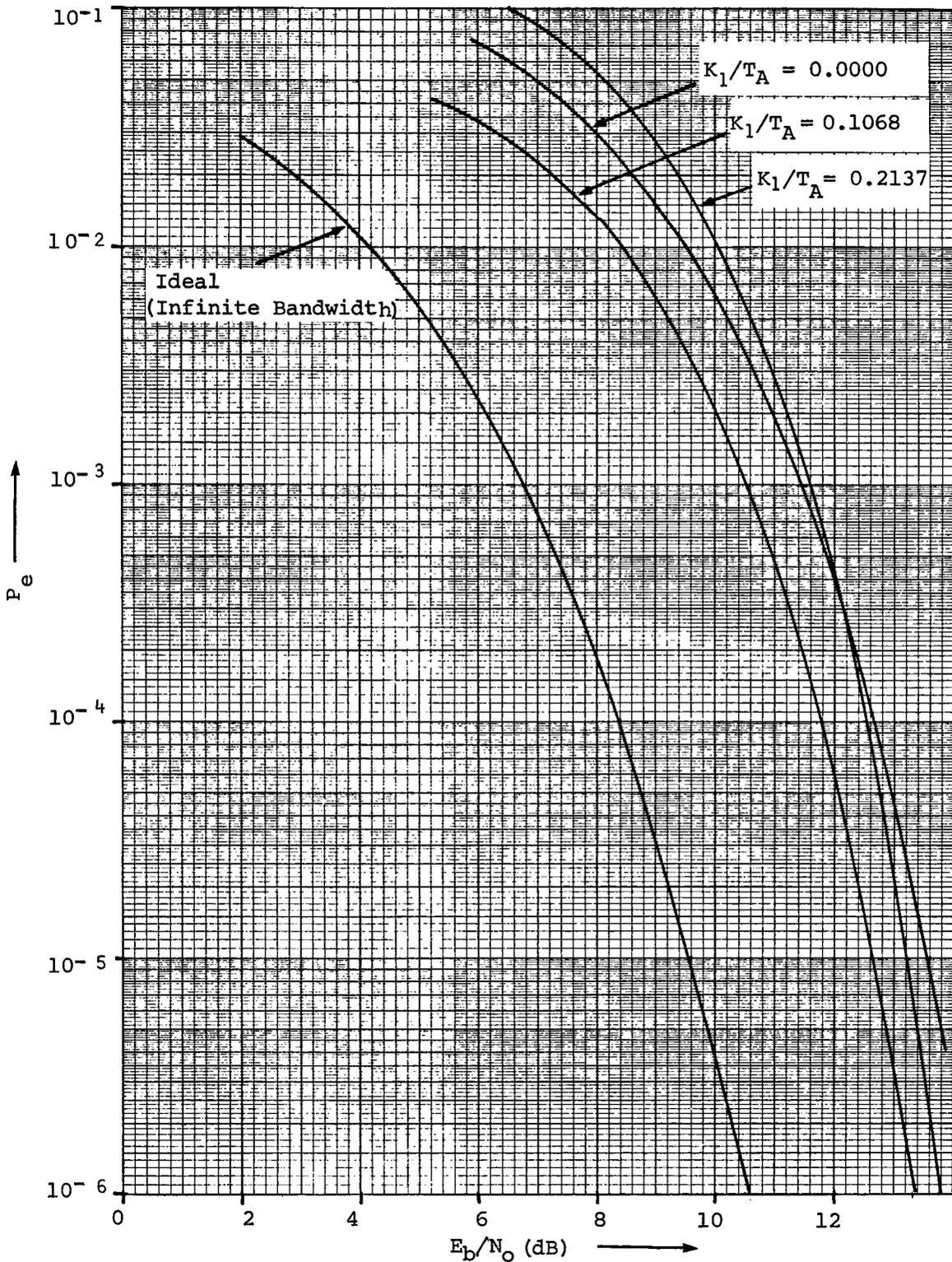
Fig. 4.16. - Error probability results for single-channel QPSK transmission with practical filtering ( $K_1/T_A$  varying,  $f_c T_A = 1$ ,  $B_{IF} T_A = 1$ ,  $T_A/T_B = 1$ )
