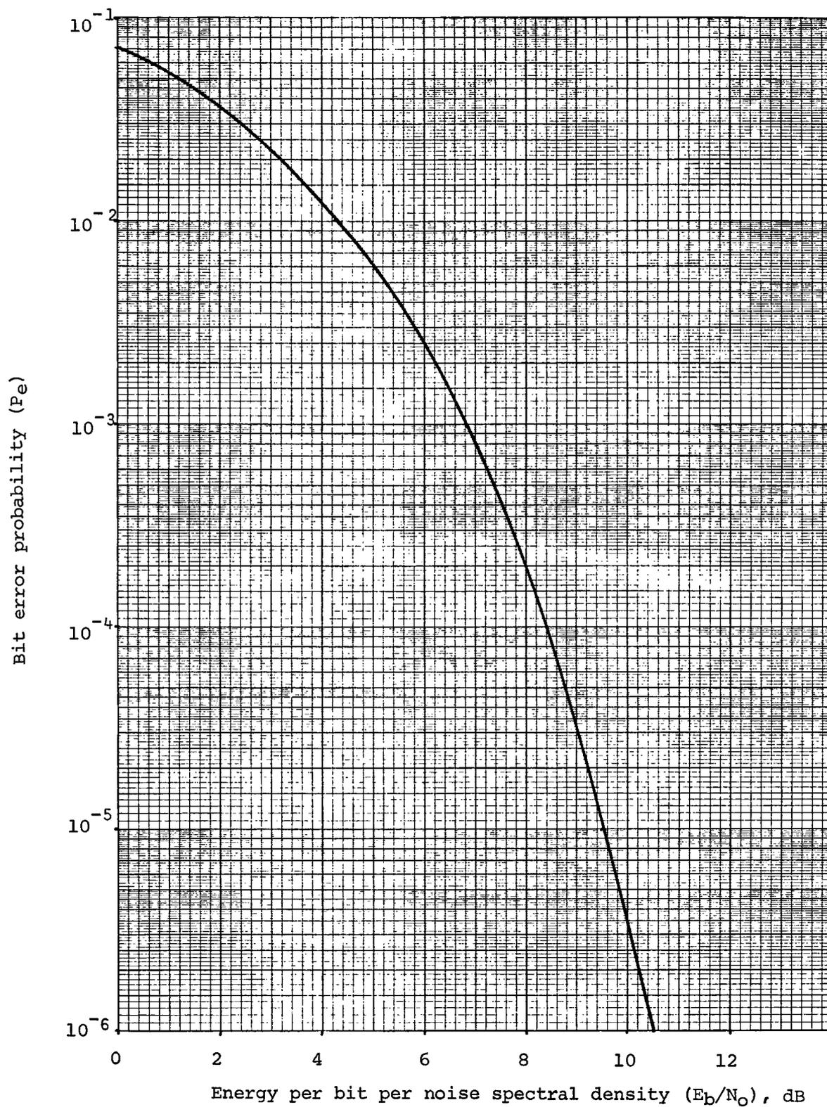
Fig. 1.5. - Probability of error for optimum binary signaling
