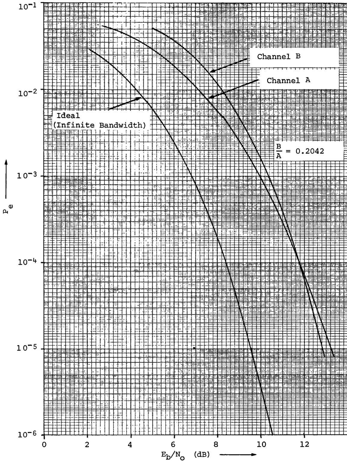
Fig. 4.12. - Iterated error probability results for dual-channel QPSK transmission with ideal rectangular filtering ( $f_c T_A = 10$ ,  $T_A/T_B = 0.1$ ,  $B_{IF} T_A = 1$ )
