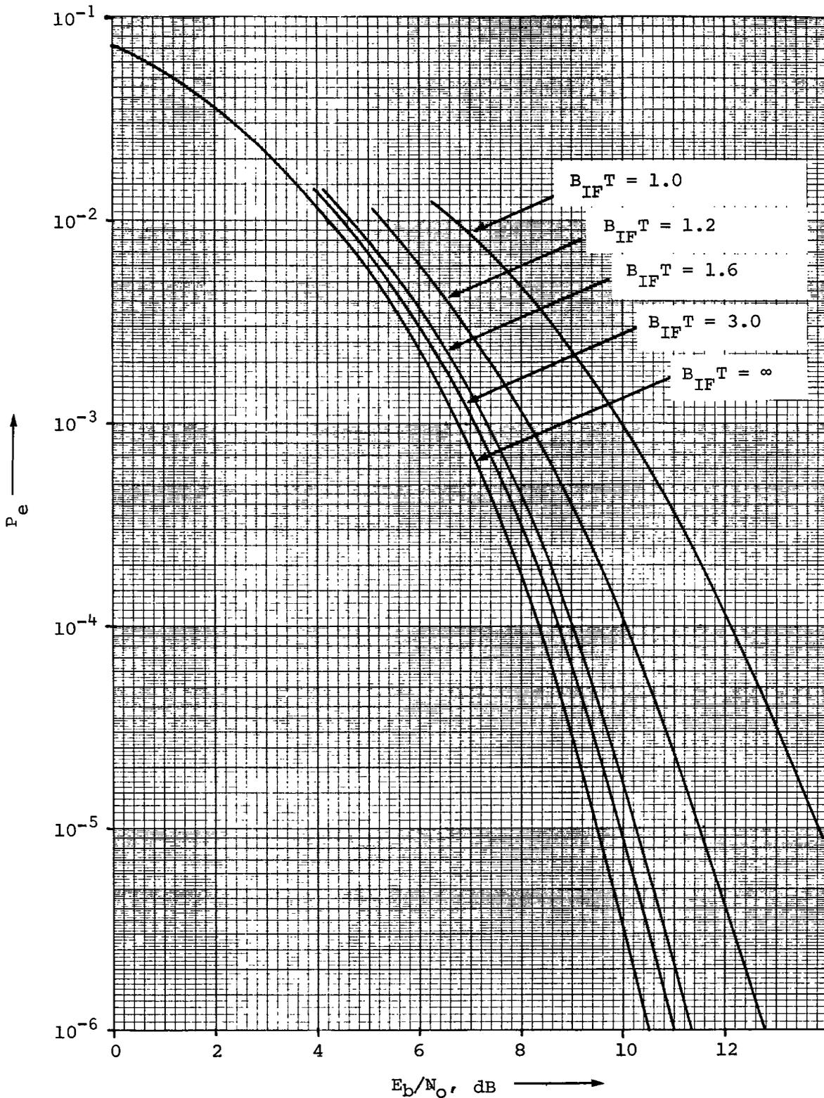
Fig. 2.6. -  $P_e$  vs.  $E_b/N_0$  for ideal bandlimited PSK with  $f_c T = \infty$
