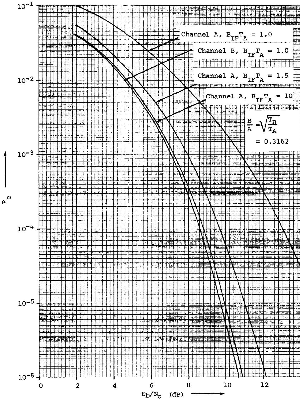
Fig. 4.10. - Error probability results for dual-channel QPSK transmission with ideal rectangular filtering ( $f_c T_A = 1$ ,  $T_A/T_B = 0.1$ )
