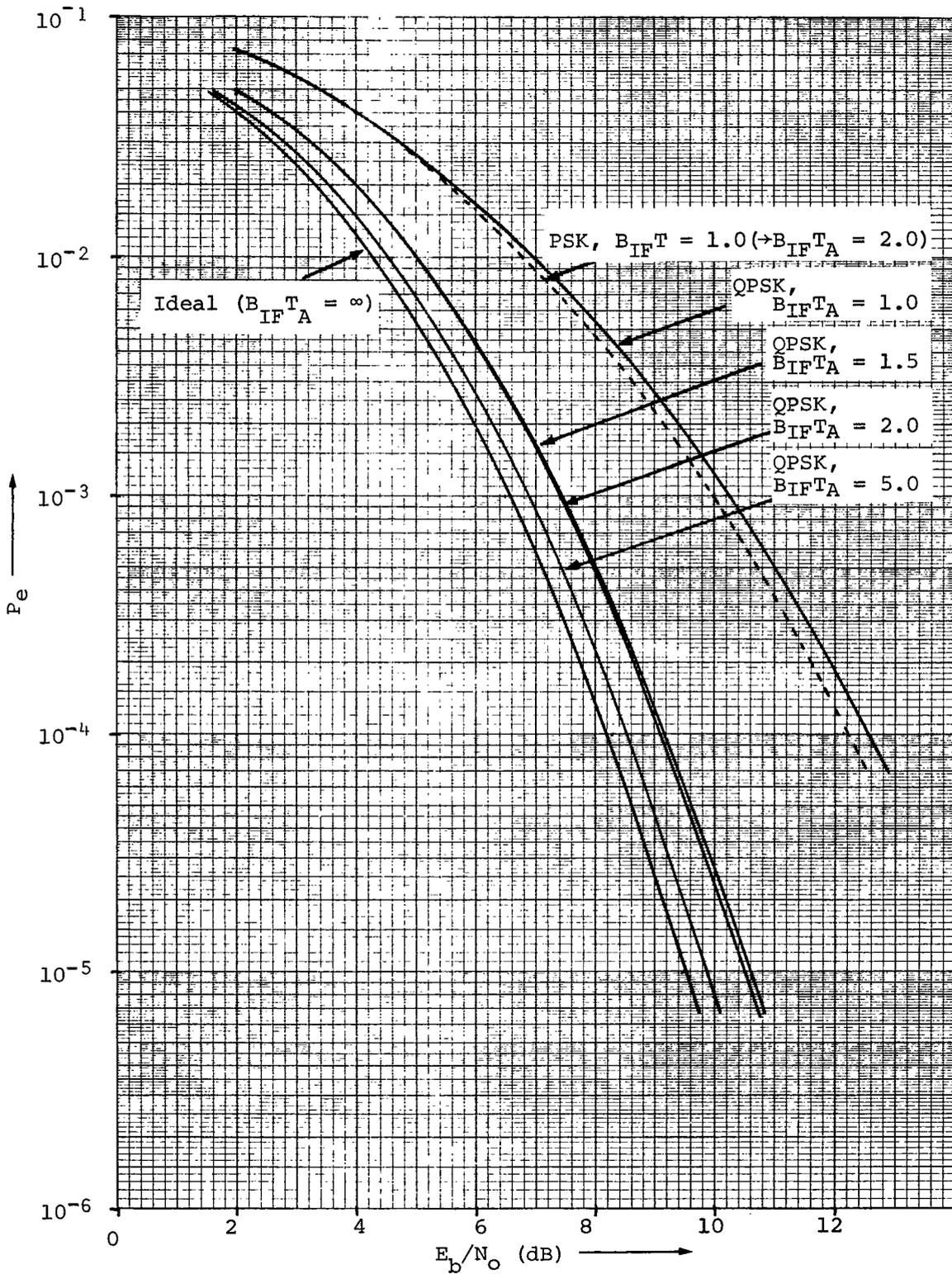
Fig. 4.5. - Error probability results for single-channel QPSK transmission with ideal rectangular filtering ( $f_c T_A = 5$ )
