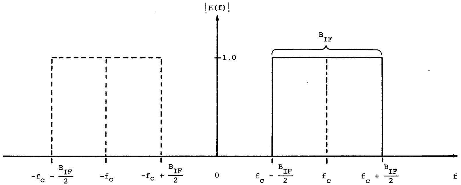
Fig. 4.2 - Bandpass filter characteristic for ideal rectangular filter
