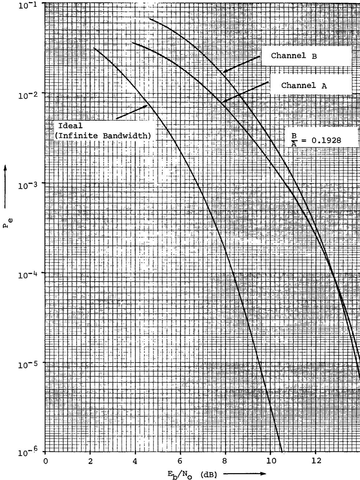
Fig. 4.14. - Iterated error probability results for dual-channel QPSK transmission with ideal rectangular filtering ( $f_c T_A = 1$ ,  $T_A/T_B = 0.1$ ,  $B_{IF} T_A = 1$ )
