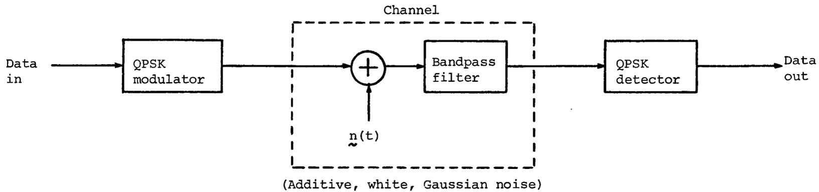
Fig. 4.1. - Bandlimited QPSK model
