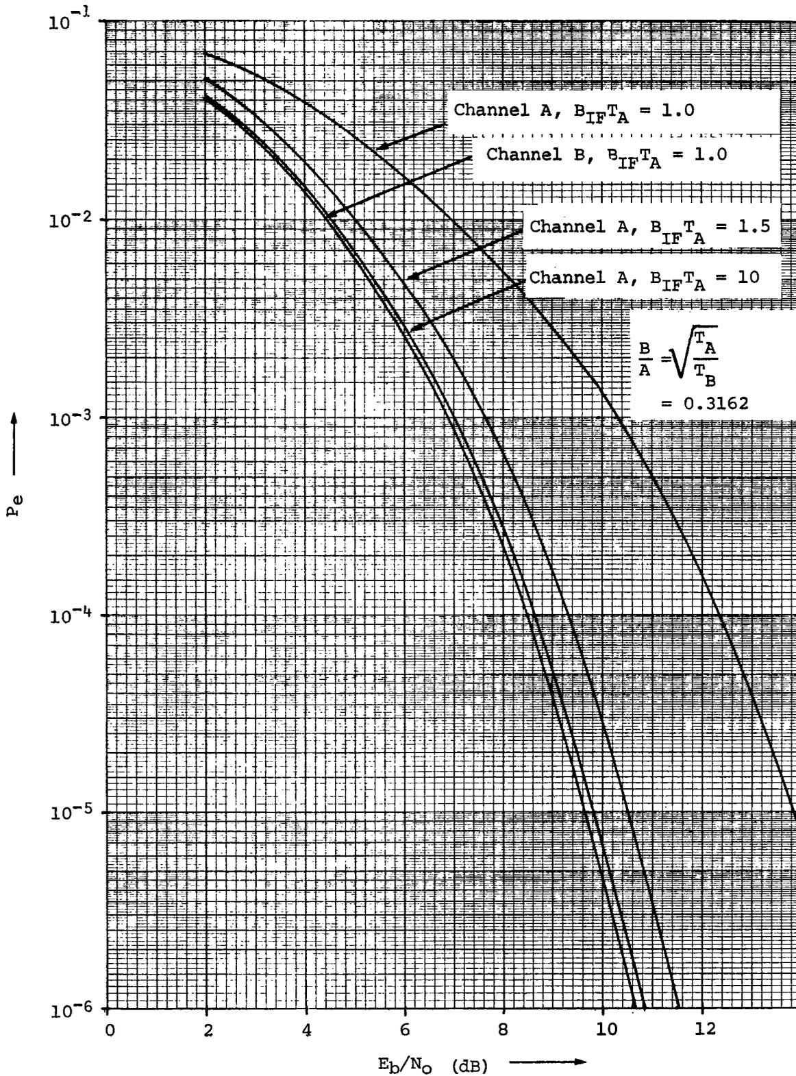
Fig. 4.8. - Error probability results for dual-channel QPSK transmission with ideal rectangular filtering ( $f_c T_A = 10$ ,  $T_A/T_B = 0.1$ )
