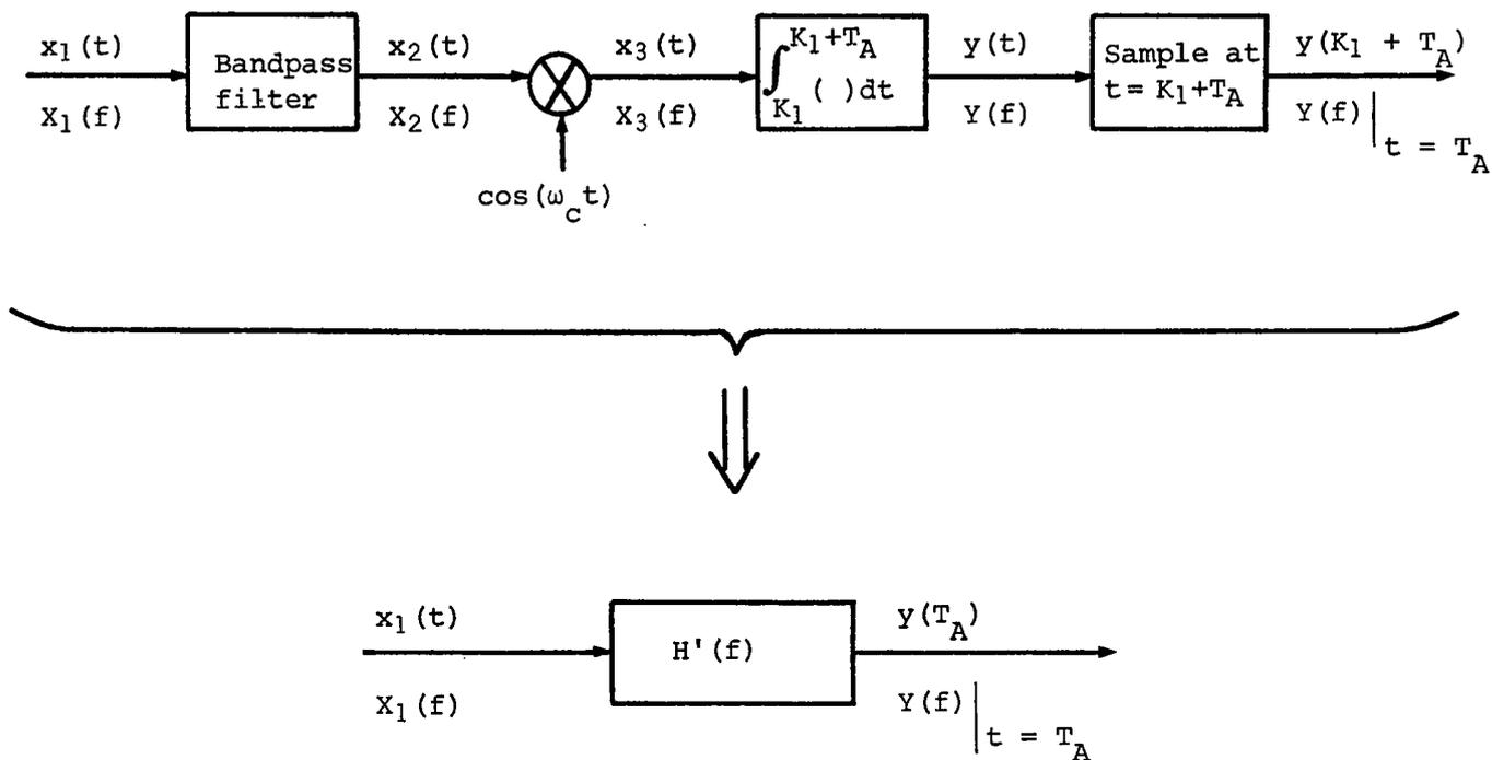
Fig. F.1. - Combination of single-pole filter with Channel A detector components
