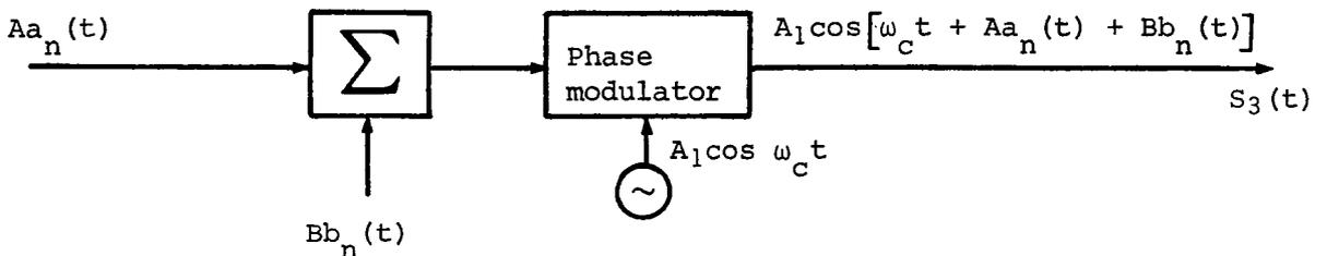
(c) Phase modulation of a single carrier by a quaternary (four-level) signal  $[Aa_n(t) + Bb_n(t)]$  is four-level for  $a_n(t) = \pm 1, b_n(t) = \pm 1,$  and  $A \neq B]$
