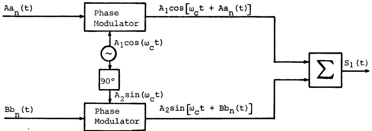
(a) Addition of phase-modulated quadrature carriers  $[a_n(t) = \pm 1, b_n(t) = \pm 1]$
