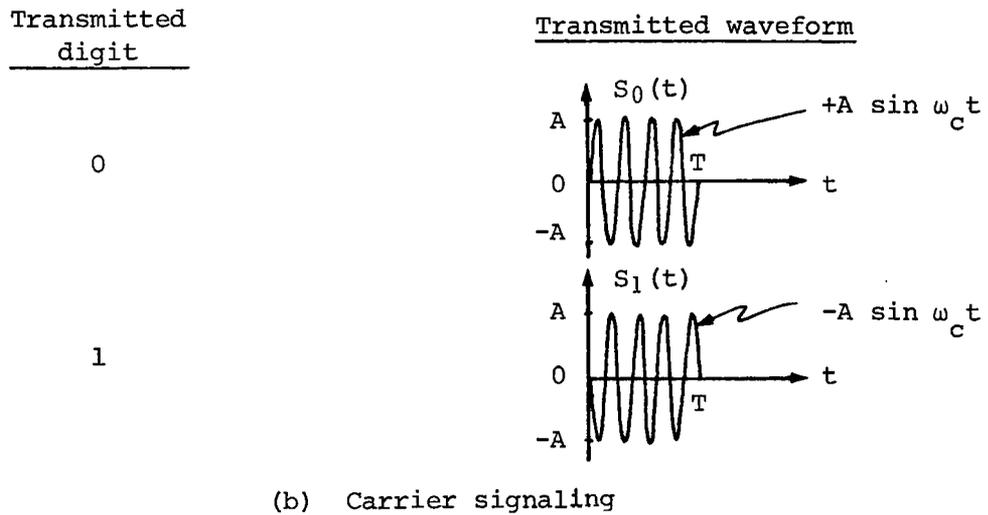
Fig. 1.3. - Optimum waveforms for binary transmission over the additive, white, Gaussian noise channel
