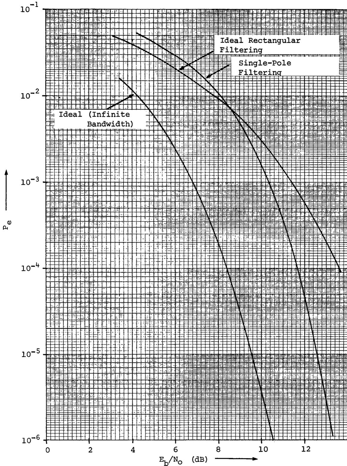
Fig. 4.18. - Comparison of error probability results for single-channel QPSK transmission ( $f_c T_A = 1$ ,  $T_A/T_B = 1$ ,  $B_{IF} T_A = 1$ )
