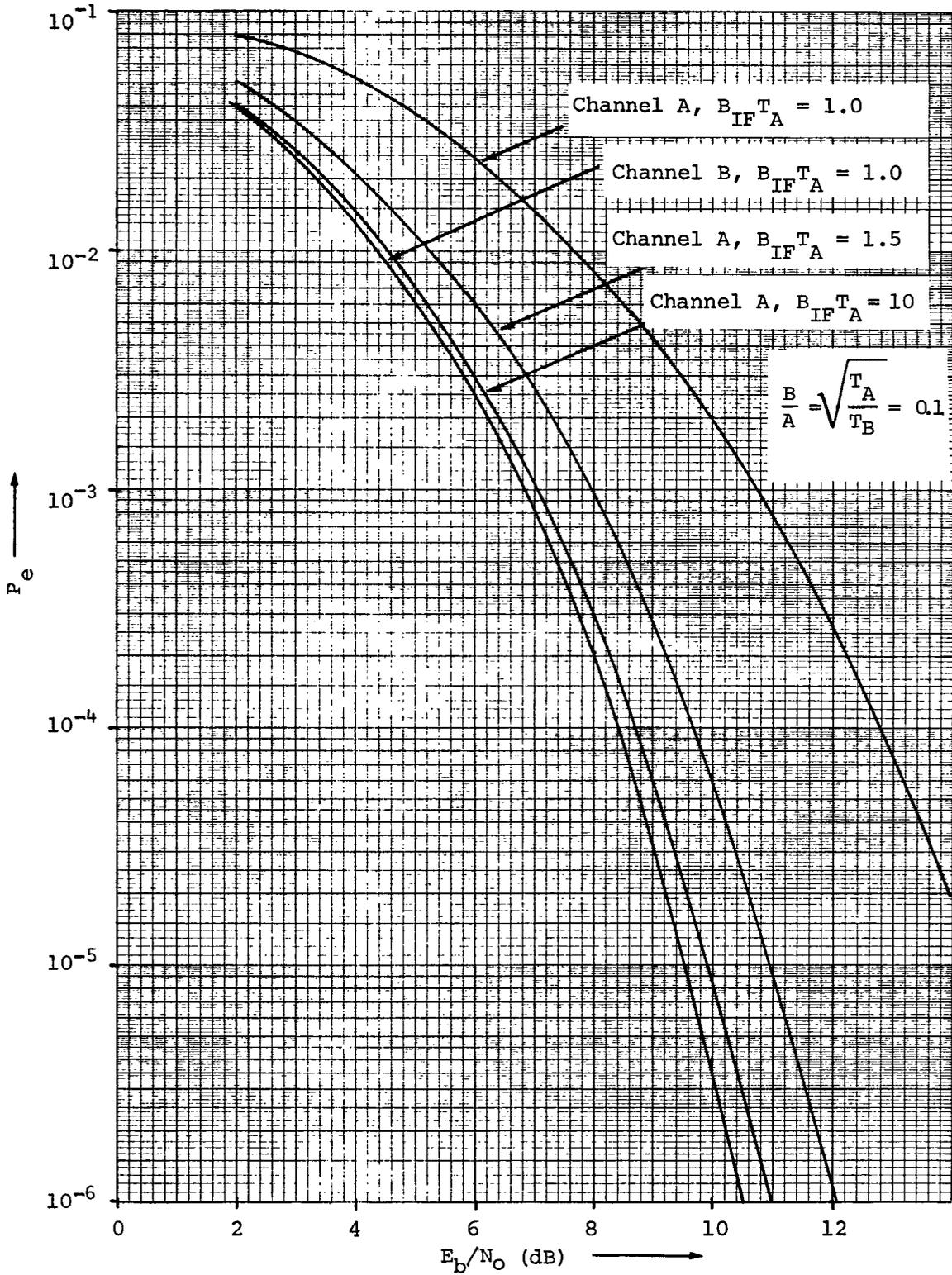
Fig. 4.9. - Error probability results for dual-channel QPSK transmission with ideal rectangular filtering ( $f_c T_A = 1, T_A/T_B = 0.01$ )
