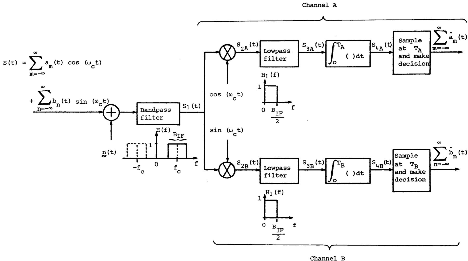
Fig. 4.3. - QPSK detection model for ideal rectangular filtering
