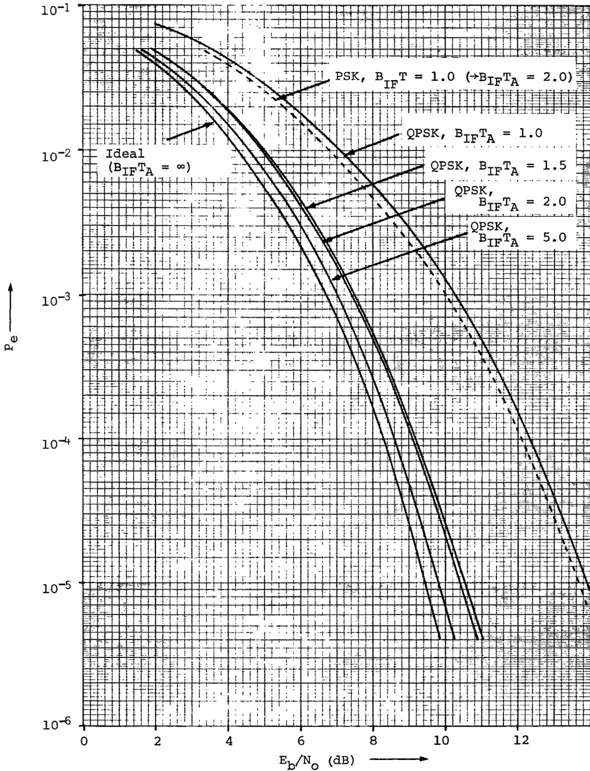
Fig. 4.4. - Error probability results for single-channel QPSK transmission with ideal rectangular filtering ( $f_c T_A = 10$ )
