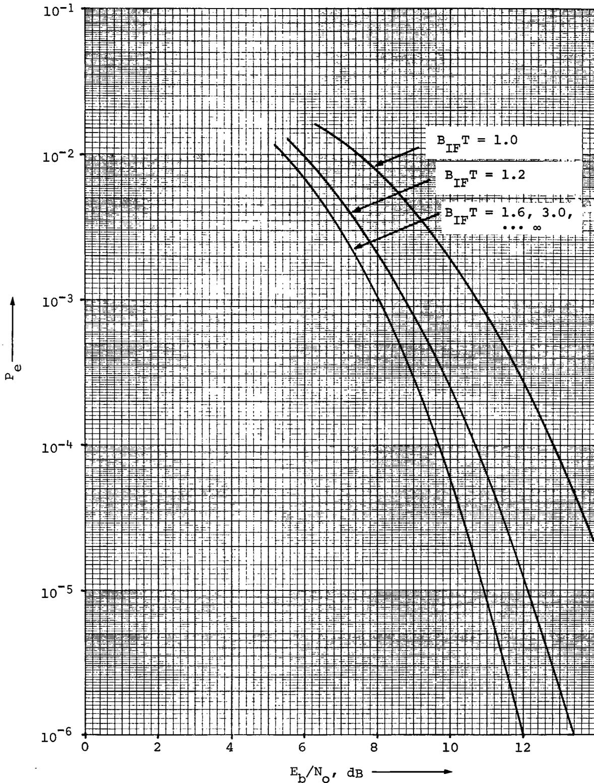
Fig. 2.4. -  $P_e$  vs.  $E_b/N_0$  for ideal bandlimited PSK with  $f_c T = 1$
