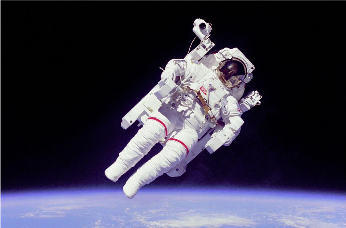
Figure 9. Bruce McCandless uses a Manned Maneuvering Unit during the STS-41-B mission, 1984, NASA
