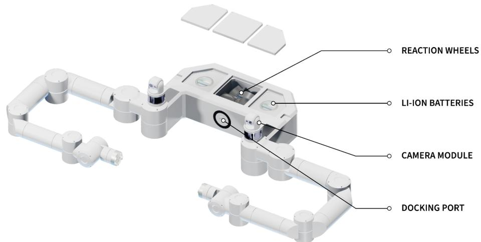
Figure 14. Exploded diagram of the Robot Module, author
