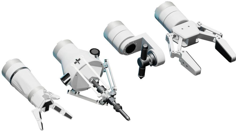
Figure 17. The four interchangeable MMEVR tools
