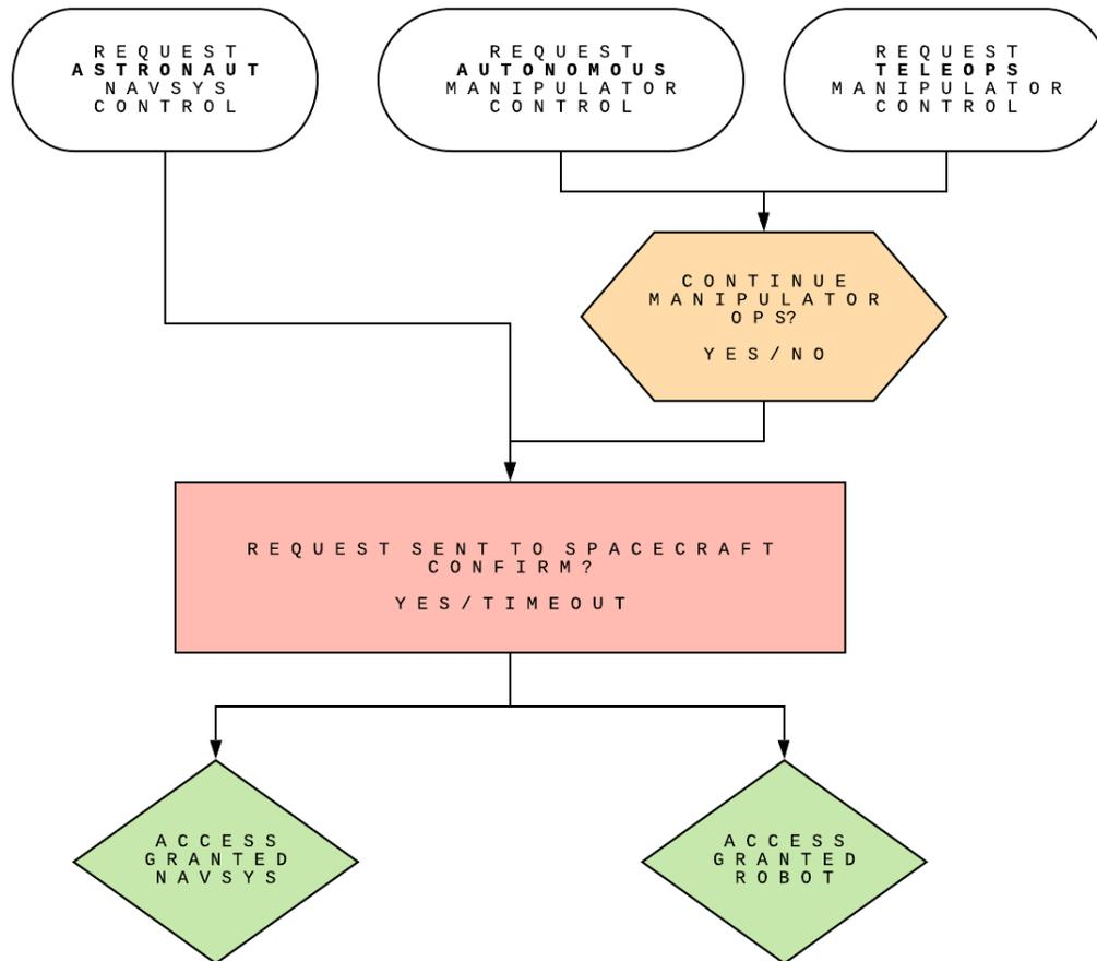
Figure 23. Control Mode Transfer Diagram, author
