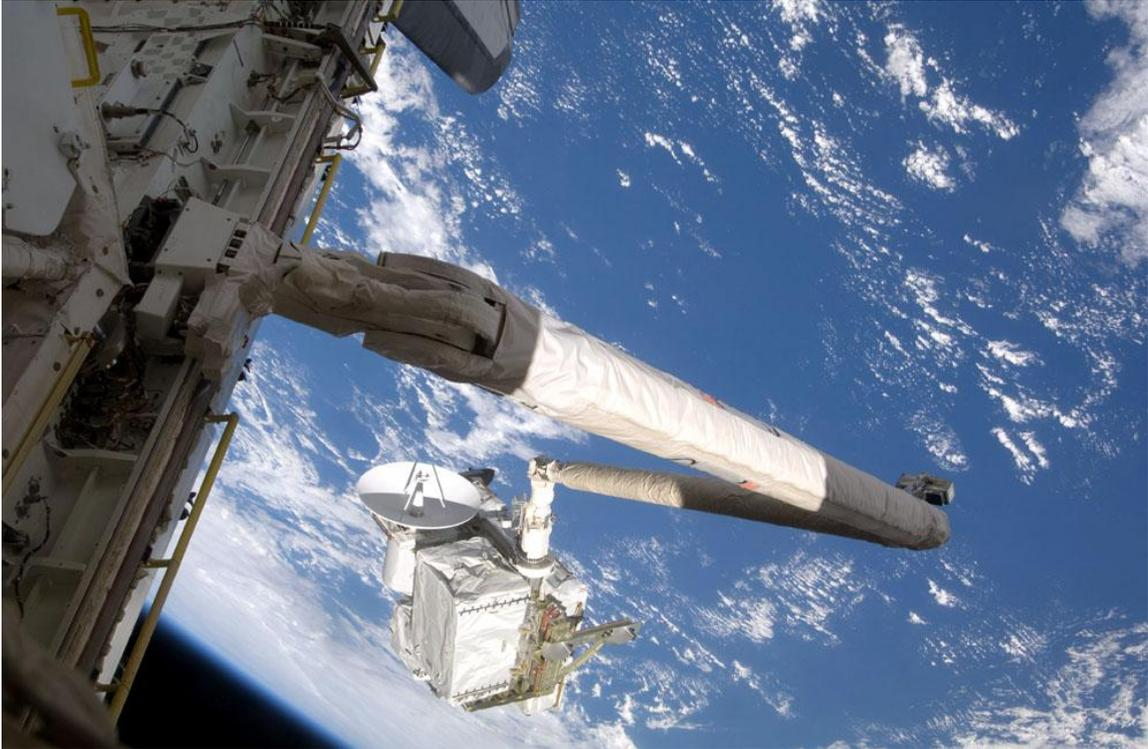
Figure 6. The Canadarm during a payload transfer operations between the Endeavour and the ISS, 2009 NASA
