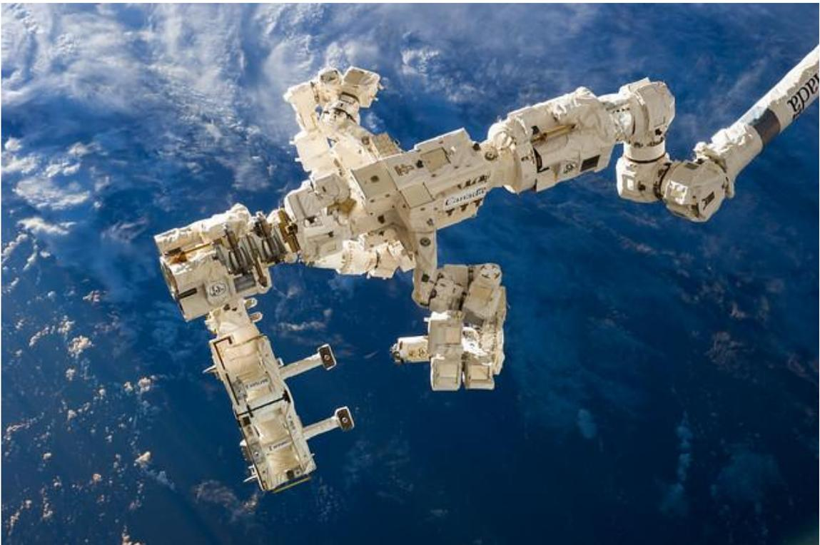
Figure 11. DEXTRE grappled to the end effector of the Canadarm2, 2019, NASA
