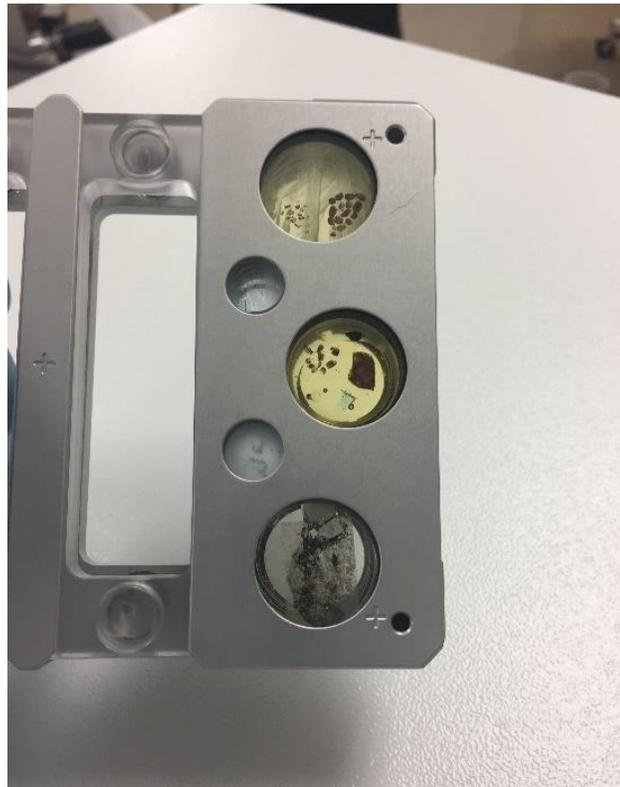
**Figure 27.** Samples before loading into the ICP-MS. The bottom sample is LEW 85300-46, the middle sample are the standards that were used, and the top sample was for another study, unrelated to this paper.
