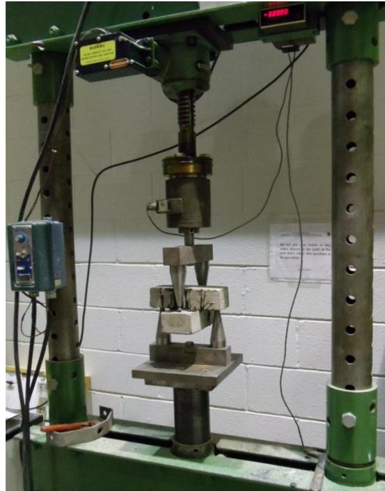
**Figure 3-4: Experimental setup of tensile bonding strength test**
