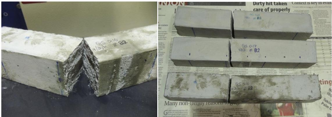
**Figure 5-6: Failed Geospray beams after subjected to four point flexural loading**
