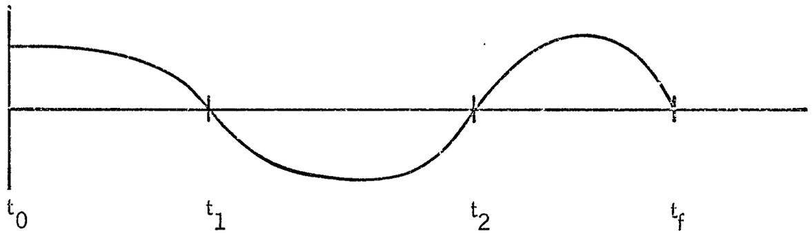
Figure 3.2.- Switch function corresponding to the thrust program of figure 3.1.
