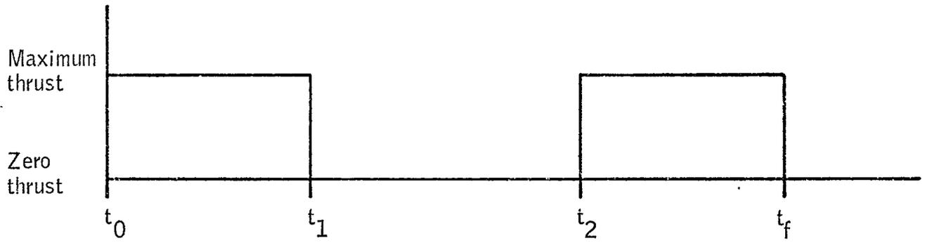
Figure 3.1.- Typical thrust program for bang-bang control.
