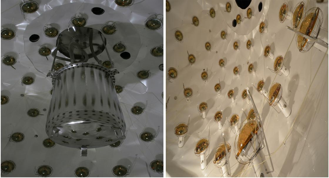
Figure 2.8: (Left) The Liquid Scintillator Veto (LSV). The picture shows the cryostat of the DarkSide-50 LAr TPC hanging from the top. (Right) The picture shows the internal surface of the LSV, covered with Lumirror, with PMTs evenly distributed inside. Figure taken from [58].
