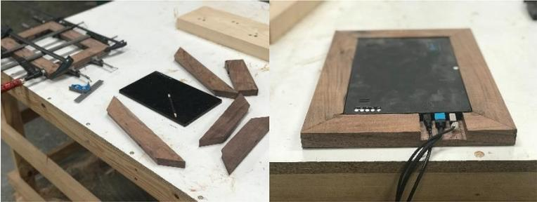
Fig. 54: Picture frame construction for the video monitor.
