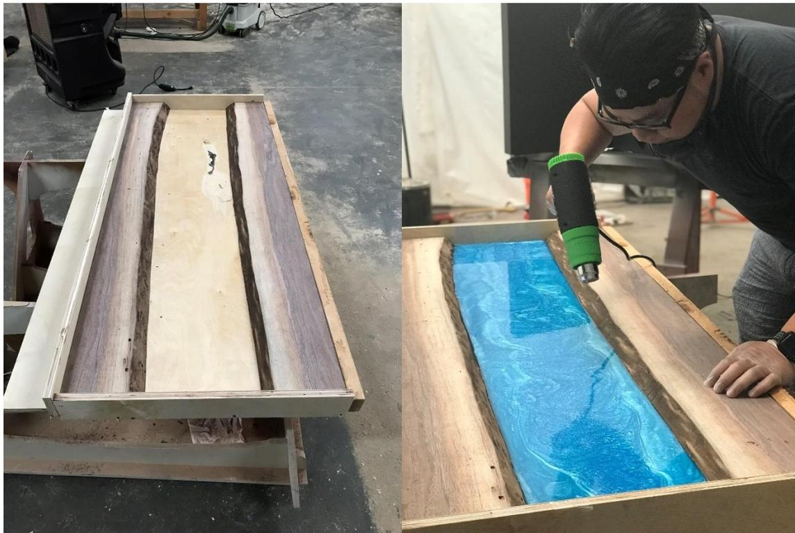
Fig. 45: Containment box and pouring process. Facilitating the release of bubbles.
