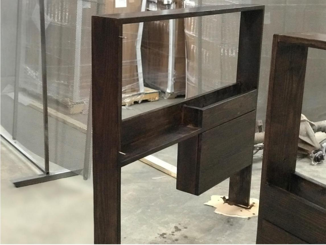
Fig. 53: Cam-lock is visible after staining the workstation.
