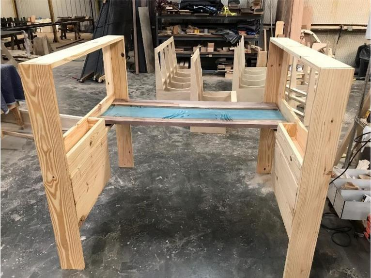
Fig. 51: Frames and desk ready for staining.
