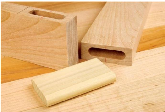
Fig. 33: Loose tenon joinery. Image Source:
