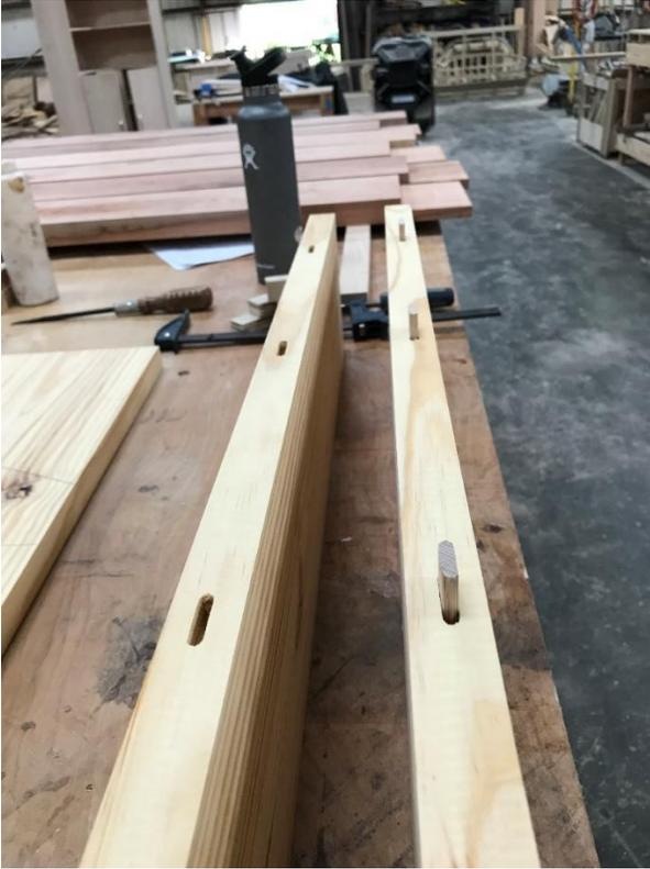
Fig. 48: Loose-tenon joinery using a Festool Domino tenon.
