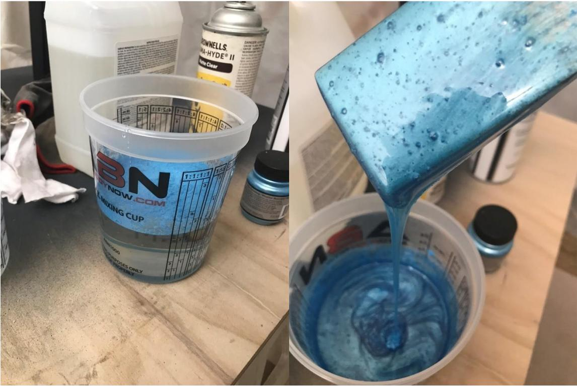
Fig. 44: Epoxy-resin mixing with metallic blue particles.
