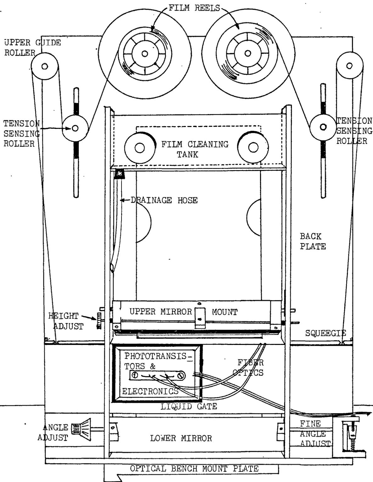
FIGURE 4. Schematic Diagram of Film Transport - Front Side
