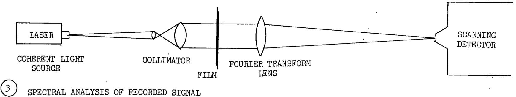
Figure 2. Fourier Optical Multichannel Analog Signal Processing System.
