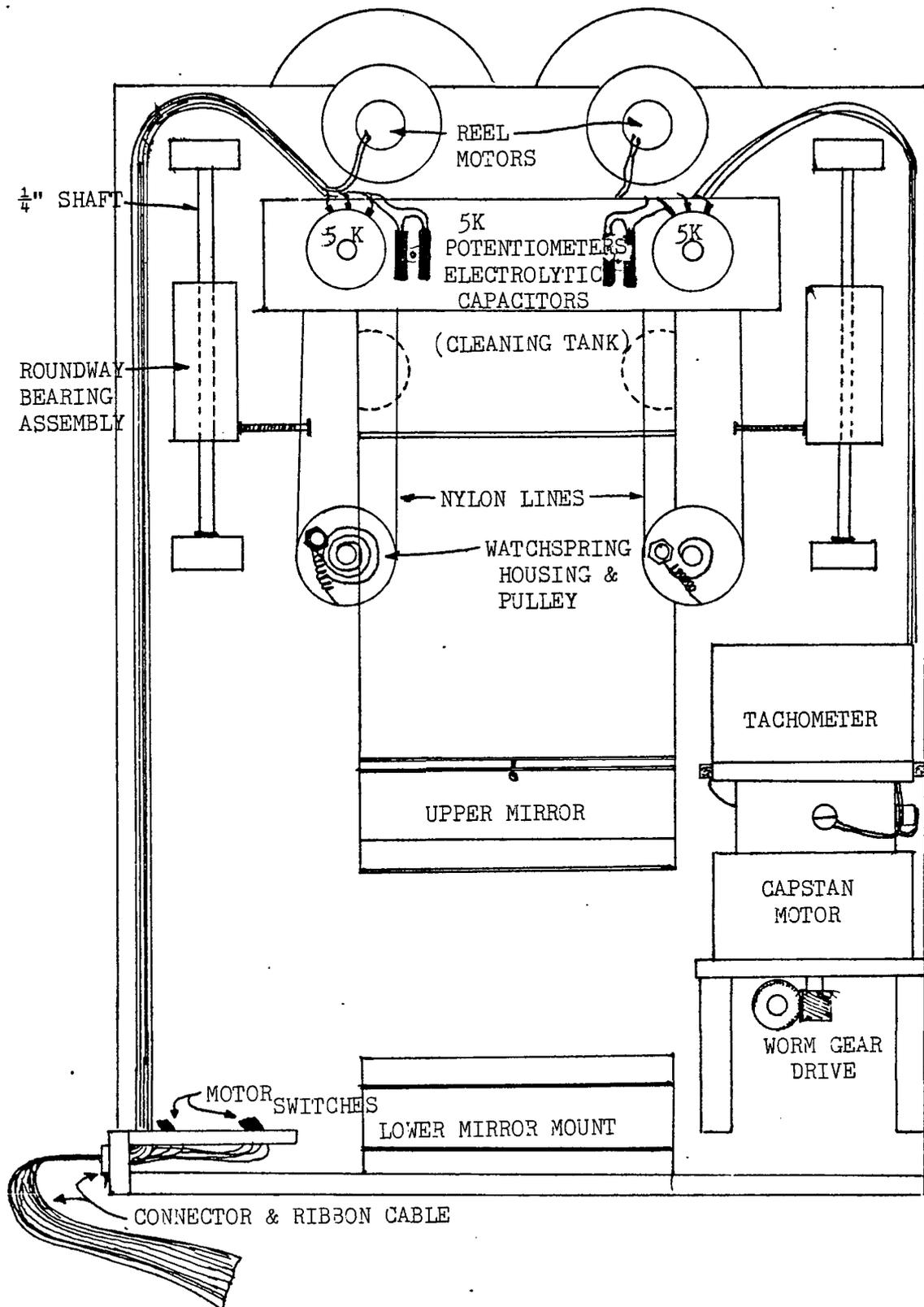
FIGURE 6 Schematic Diagram of Film Transport- Back Side
