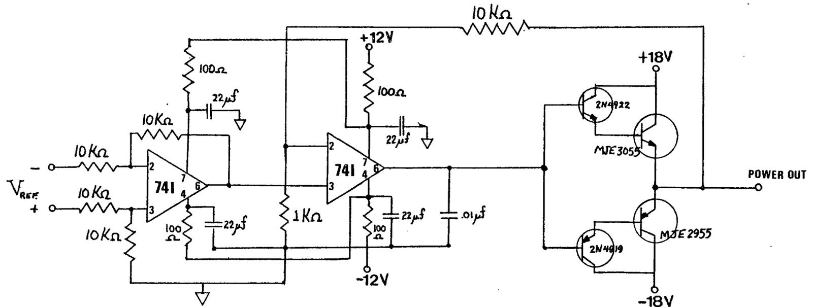
Figure II. Reference Voltage Power Amplifier
