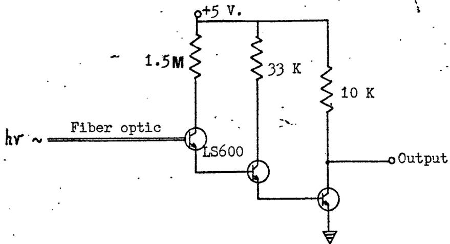
Figure 16. TTL Compatible Light-to-Voltage Transducer Electronics.
