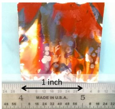
Figure 4.7 Photo of graphene domains on oxidized Cu foil.
