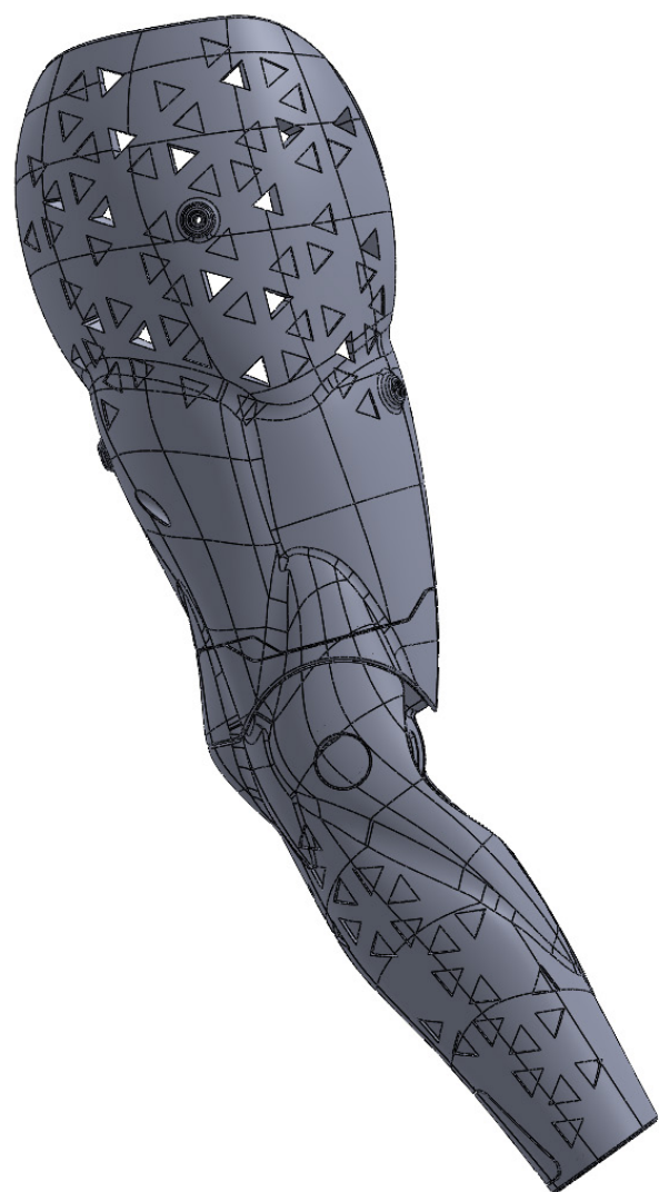
Third and final design iteration of the prosthetic arm
