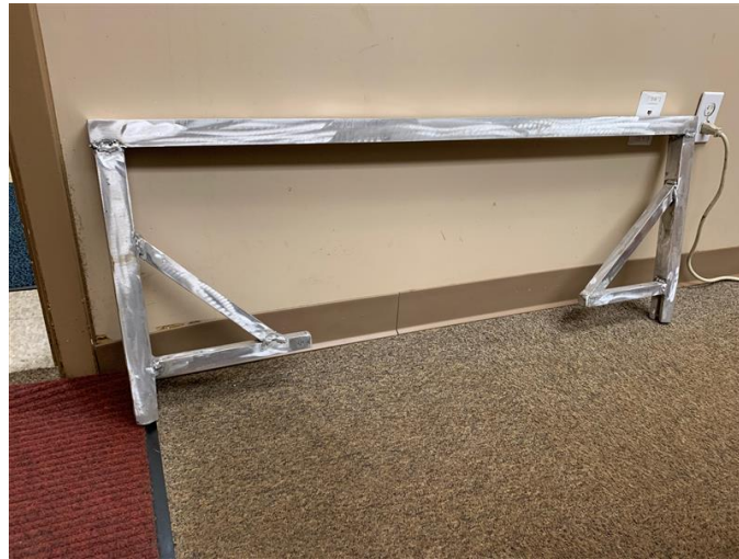
Figure 6: Photograph of the bridge stand structure used to hold the camera in place
