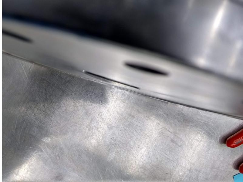
**Figure 2.19.** Silicon substrate with mung paste applied entirely on its back.
