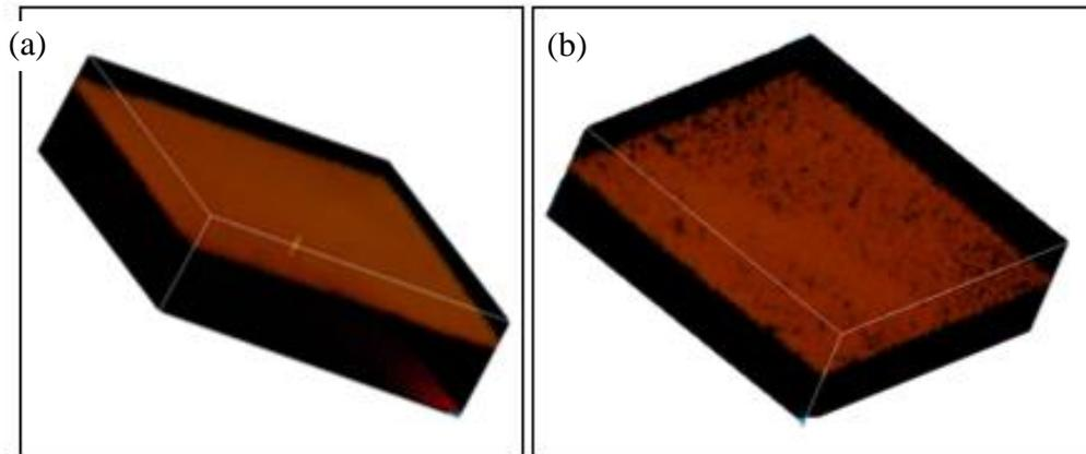
*Figure 16: Confocal spectroscopy for the red channel for an ESPA2 membrane modified with polydopamine and graphene oxide.*
