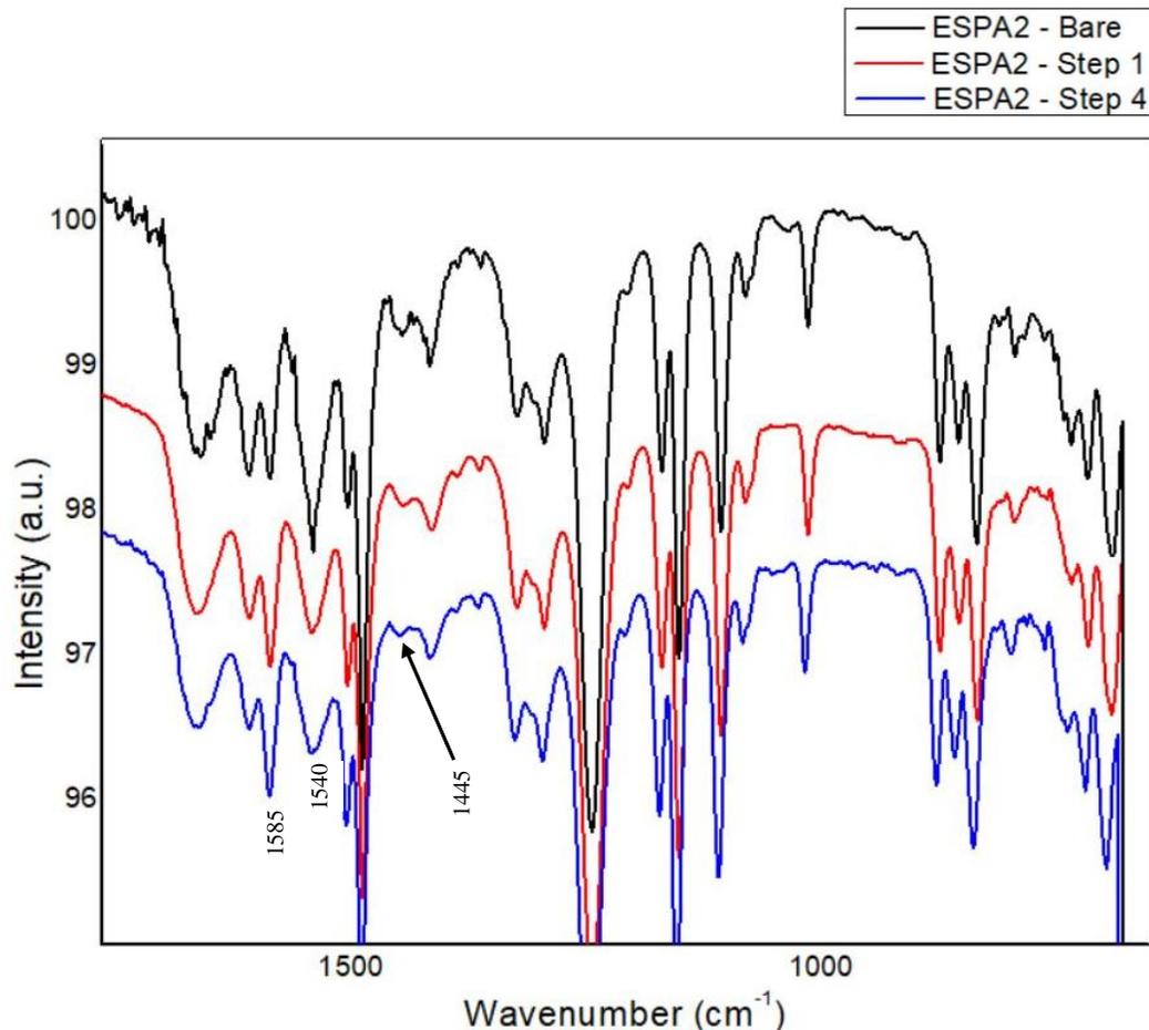
Figure 10: FTIR spectroscopy of the low wavenumber portion of the spectrum for Synthesis One. The bare membrane is compared with the modified membrane after two different reaction steps using a two-minute NaOCl reaction time.
