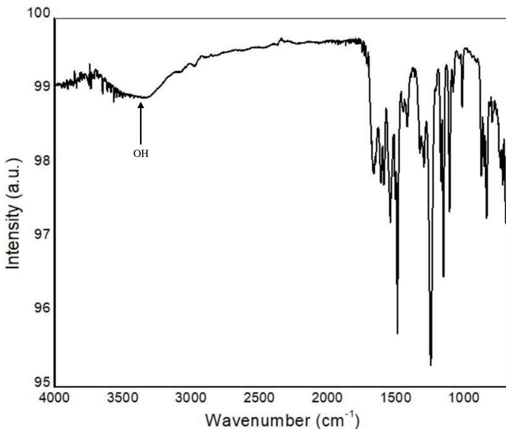
Figure 6: FTIR spectroscopy for the bare ESPA2 membrane as a reference measurement.
