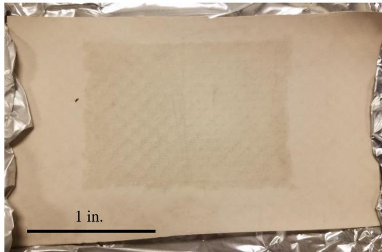
Figure 5: PA-TFC membrane after step 2 of Synthesis One.
