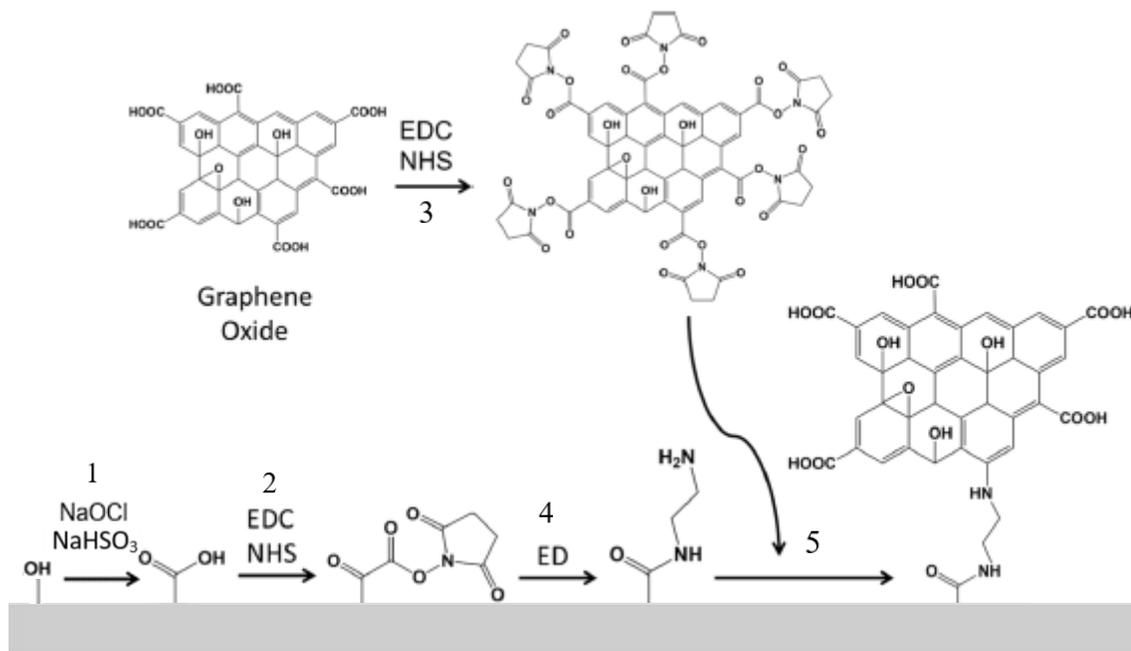
Figure 1: Reaction steps for Synthesis One. Step 1 adds NaOCl, rinses, and adds NaHSO<sub>3</sub>. Step 2 functionalizes the membrane with EDC and NHS. Step 3 activates the graphene oxide (GO) with EDC and NHS. Step 4 functionalizes the membrane with ED. Step 5 attaches the activated GO to the ED functionalized membrane.
