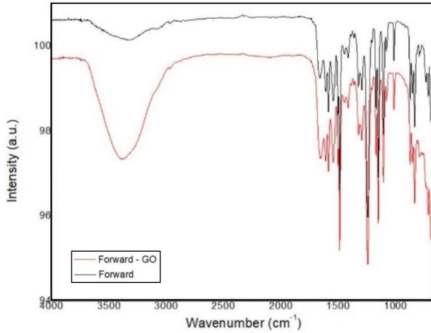
Figure 19: FTIR spectroscopy for Synthesis One using a forward osmosis membrane.
