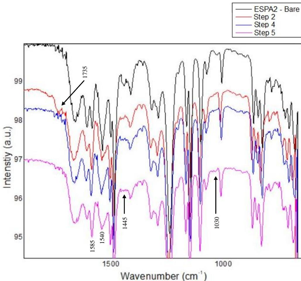
Figure 11: FTIR spectroscopy of the low wavenumber portion of the spectrum for Synthesis One. The bare membrane is compared with the modified membrane after completing 3 different reaction steps using a 5-minute NaOCl reaction time.
