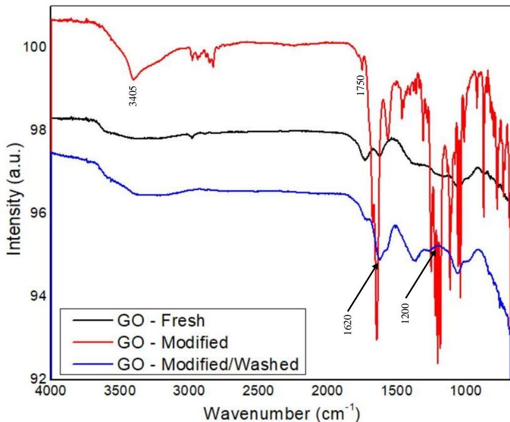
Figure 9: FTIR spectroscopy of fresh graphene oxide (GO), GO modified with NHS/EDC, and modified/washed GO.
