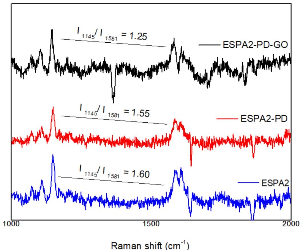
Figure 14: Raman spectroscopy data for the ESPA2 membrane bare and modified with PDA and PDA/GO.
