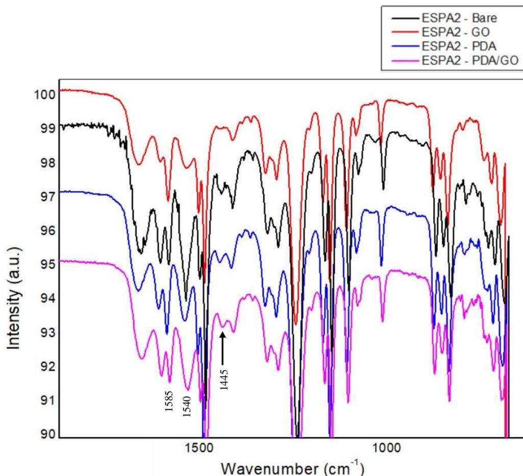
Figure 13: FTIR for the low wavenumber portion of the spectrum for the ESPA2 membrane bare and modified with graphene oxide (GO), polydopamine (PDA), and PDA/GO.
