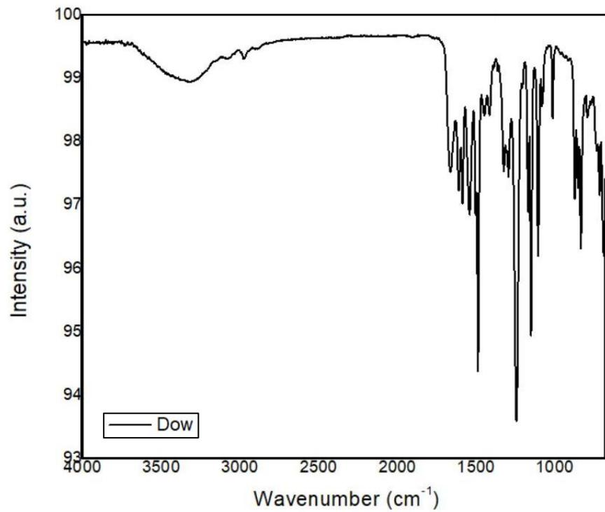
Figure 20: FTIR spectroscopy for Synthesis One using a reverse osmosis membrane from Dow.
