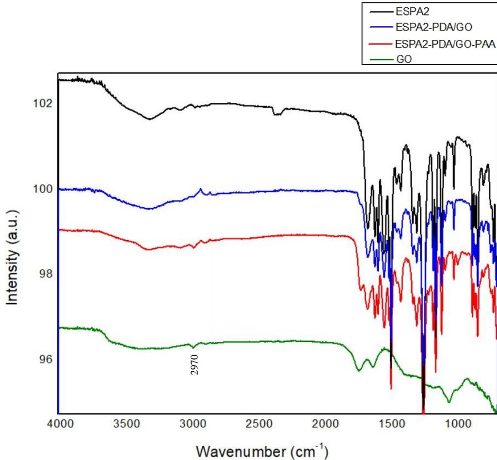
Figure 17: FTIR spectroscopy for the low wavenumber section of the spectrum for the ESPA2 membrane for Synthesis Two through the addition of polyacrylic acid (PAA) with control samples.
