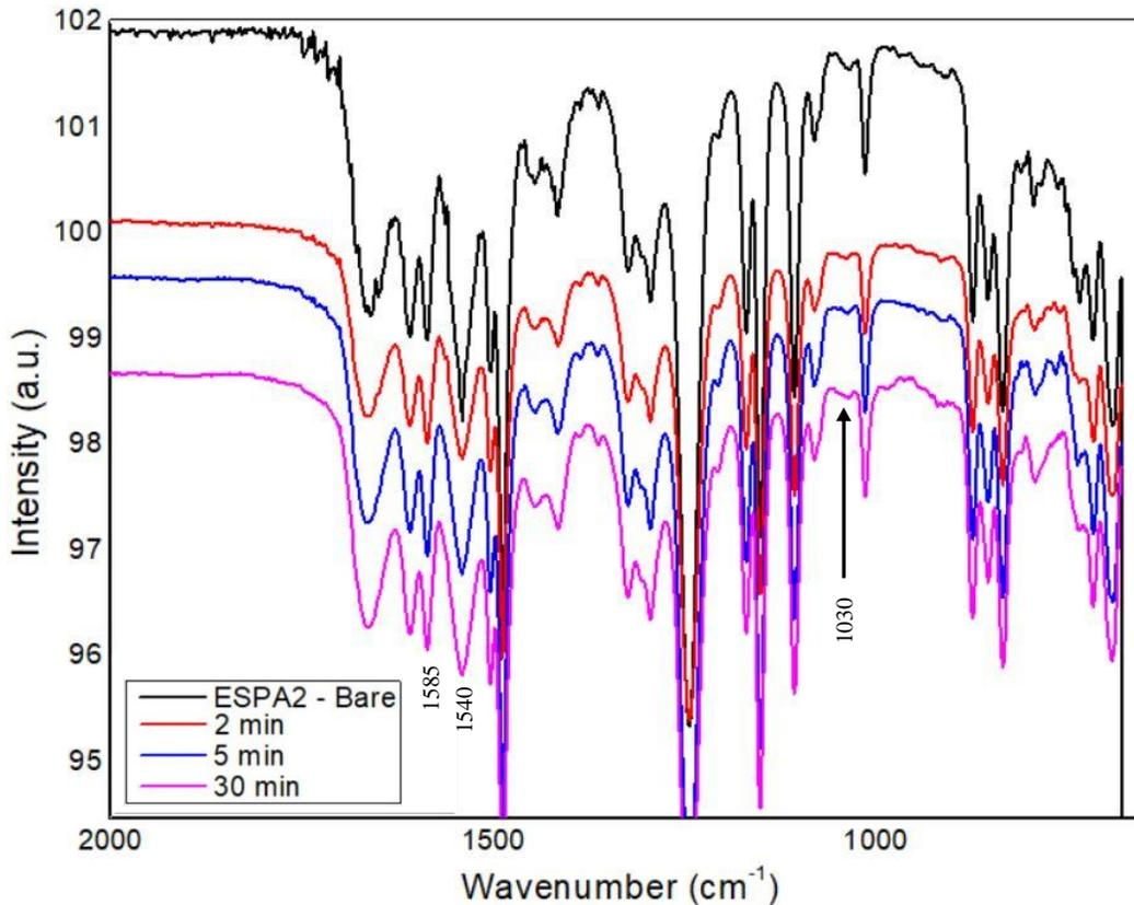
Figure 8: Enlarged view of the low wavenumber portion of Figure 7 for the NaOCl reaction of Synthesis One.
