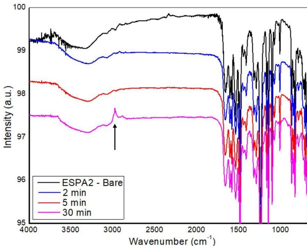
Figure 7: FTIR spectroscopy for the NaOCl reaction of Synthesis One for 2, 5, and 30 minutes along with the bare membrane.
