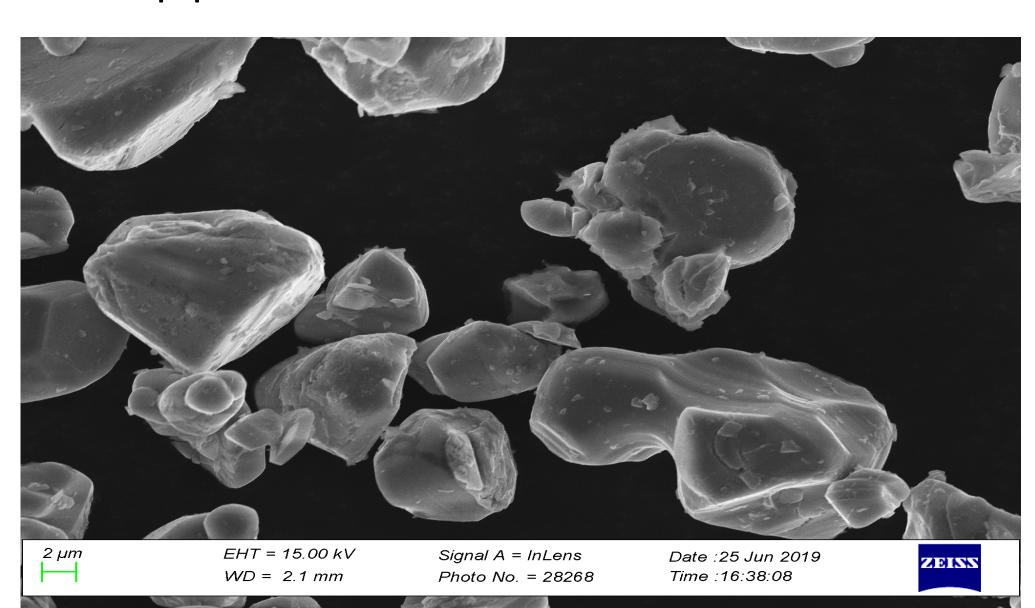
Lithium Cobalt Oxide can either be coated with Al2O3 or with Lithium Niobium Oxide but the later is the better choice.
