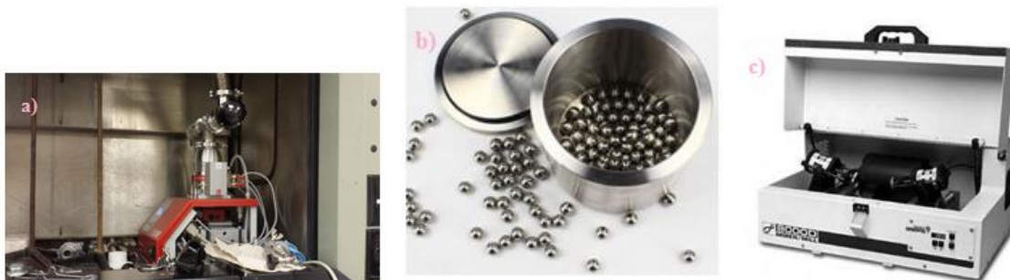
Fig. 3.3.2 a) Pumping system, b) Stainless steel jar and ball, and c) Ball-milling machine (SPEX 8000 M)
