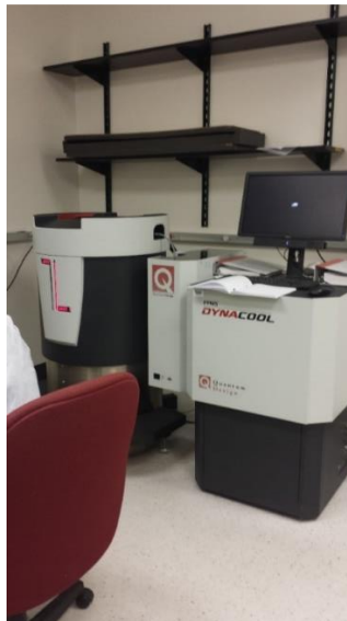
Fig. 2.5.1 PPMS (Quantum Design) for carrier concentration and mobility measurement.
