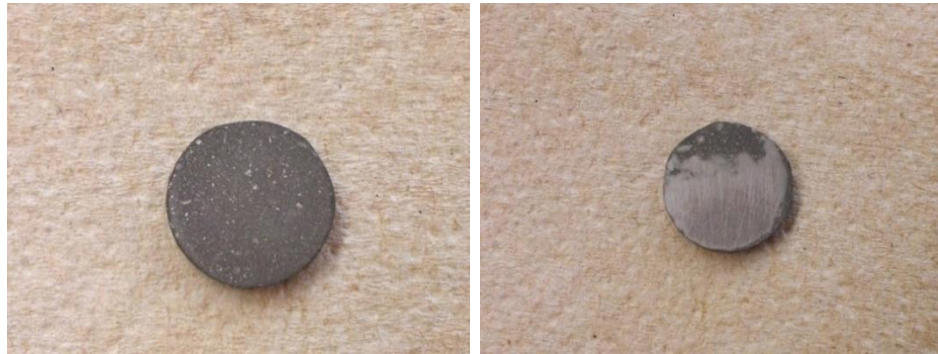
Fig. 7.3.7 Two sides of n -type Si 80 Ge 20 P 2 sample hot pressed using MoSi 2 as contact layer.
