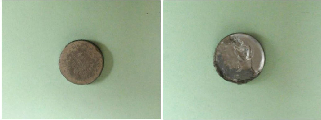
Fig. 7.3.9 n -type \text{Si}_{80}\text{Ge}_{20}\text{P}_2 sample hot pressed using \text{MoSi}_2\text{Ni}_{0.05} as contact alloy.
