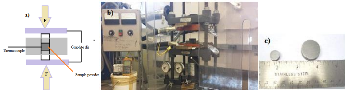
Fig. 3.3.3 a) Schematic picture of hot press, b) Lab-made hot press-system, and c) Consolidated sample disk of different size.
