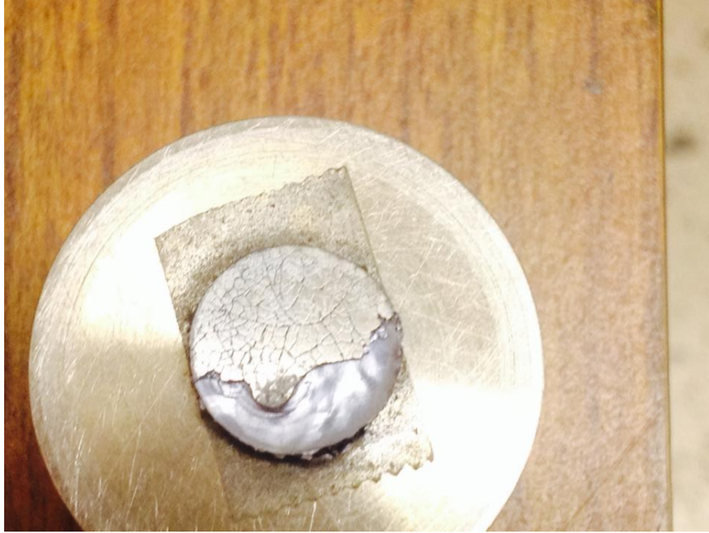
Fig. 7.3.1 n -type \text{Si}_{80}\text{Ge}_{20}\text{P}_2 sample hot pressed together with \text{CoSi}_2 as a contact layer.
