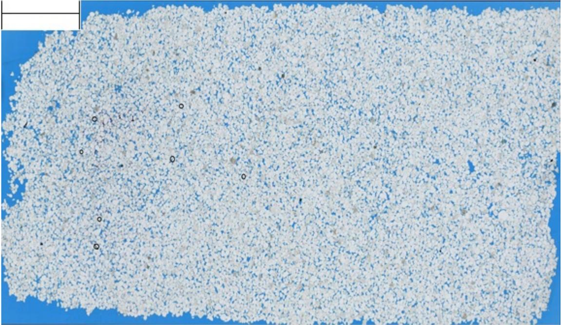
Figure 55: Pre-test Fontainebleau-1 Sandstone thin-section. The black circles show the regions from which tiles were selected for quantitative analysis. The scale bar is 0.2 in.
