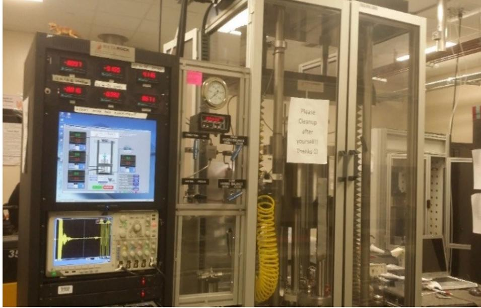
Figure 8: Experimental setup including the computerized control panel. The entire apparatus is PID controlled and capable of 75000 lb. axial load and 12000 psi confining stress.
