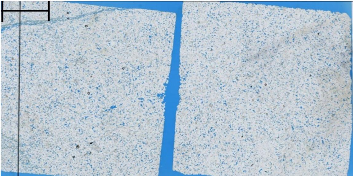
Figure 58: Post-test Fontainebleau-1-10 Sandstone thin-section image showing regions of interest. The sample was tested to a confining pressure of 2500 psi. An incipient failure surface can be seen in the thin-section. The black circles are the regions from which tiles were selected for detailed analysis. The scale bar is 0.2 in.
