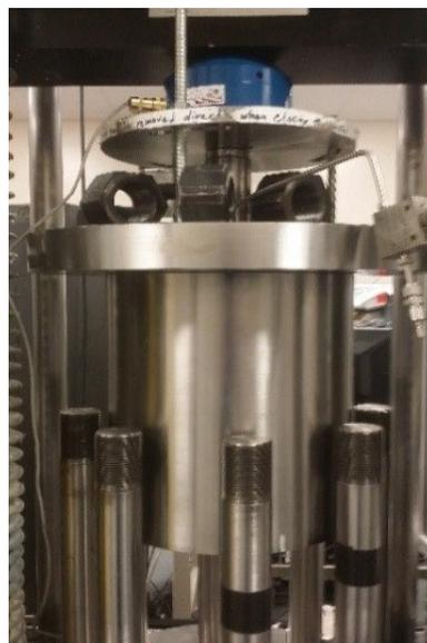
Figure 7: The cylindrical pressure vessel in which the sample assembly is placed. The maximum confining pressure is 12000 psi which is applied by displacement pumps under PID (proportional integral differential) control.
