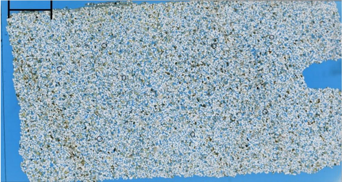
Figure 80: Pre-test Miocene sandstone thin-section. The black circles are the regions from which tiles were selected for analysis.
