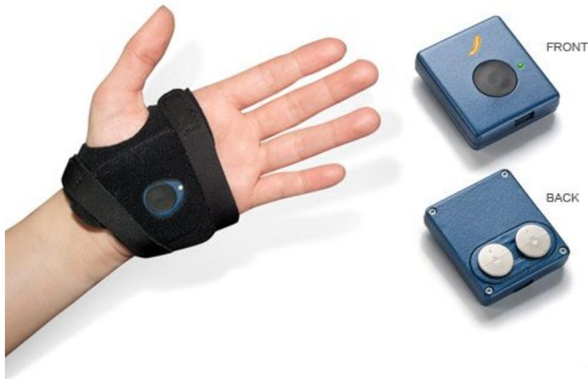
Figure 2.7: The Q Sensor worn on the palm, with the palm strap.
