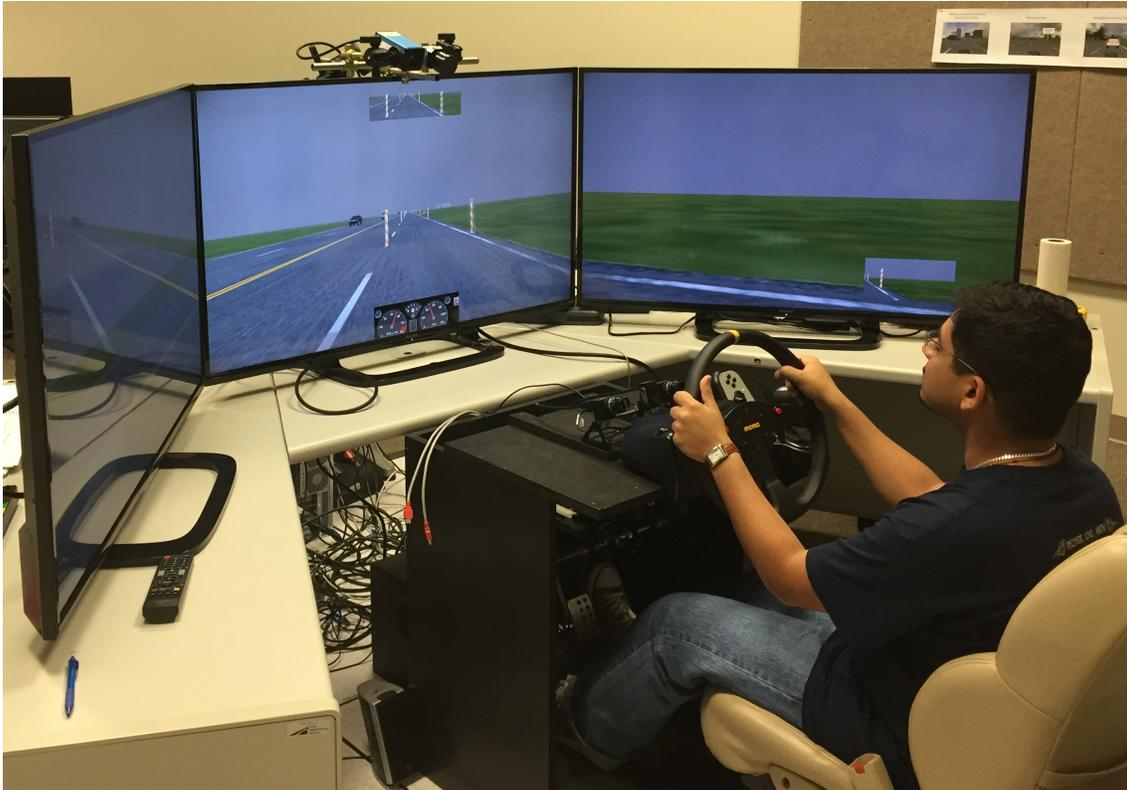
Figure 3.4: The driving simulator experimental setup. A thermal imaging camera mounted above the center TV screen records the subjects face. The virtual car is controlled by an accelerator pedal and a brake pedal, and steered with a steering wheel.
