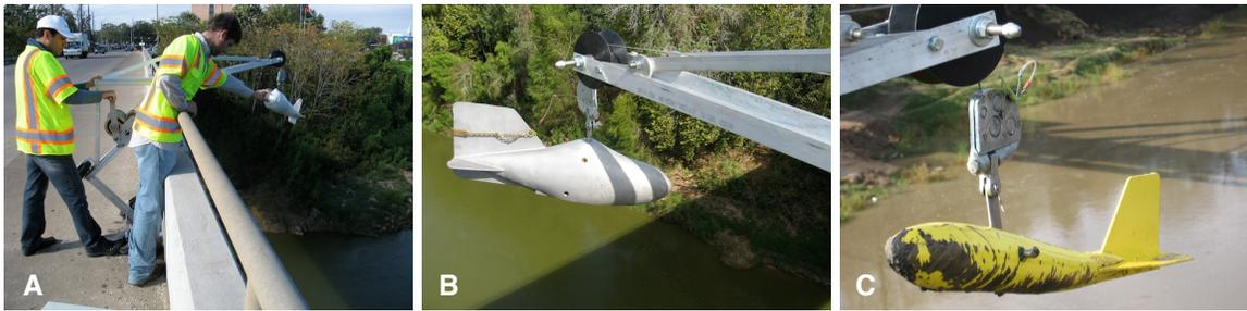
**Figure 2.3:** Primary sampling equipment. (A) US DH-2TM bag-type sampler suspended from the sampling crane; (B) US BMH-60 bed material sampler; and (C) sounding weight.
