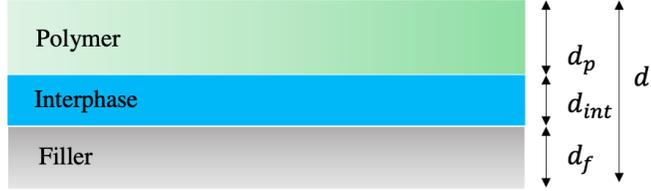
Figure 4.3: Schematic of a multi-layer composite electrolyte consisting of a filler, an interphase and a polymer.
