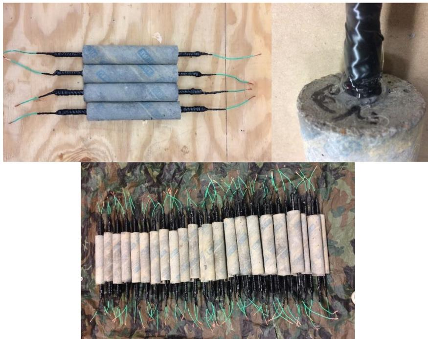
Fig. 3-5: Details of specimen ends protection from corrosion
