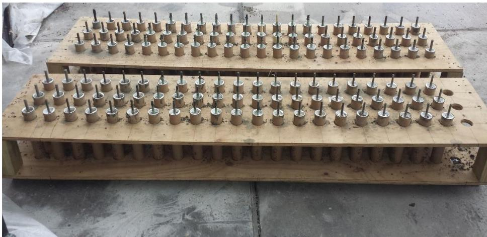
Fig. 3-3: The specimens after casting the concrete
