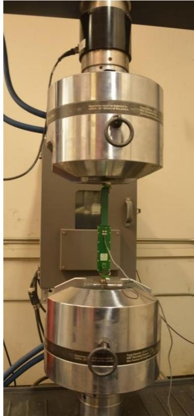
Fig. 3-11: Test setup for tensile strength tests of corroded steel rebars
