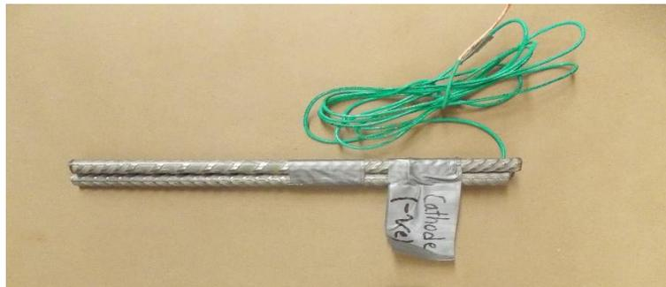
Fig. 3-6: Stainless steel cathodes rebar
