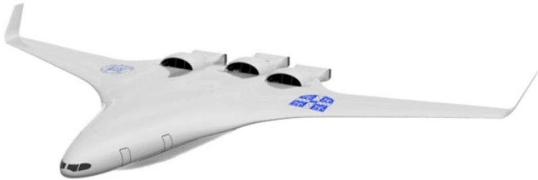
Figure 2.3: HWB distributed propulsion conceptual design [19]
