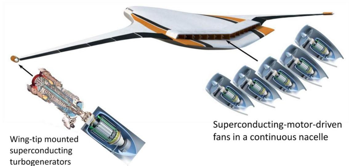
Figure 2.4: Distributed turbo-electric propulsion conceptual design [25]
